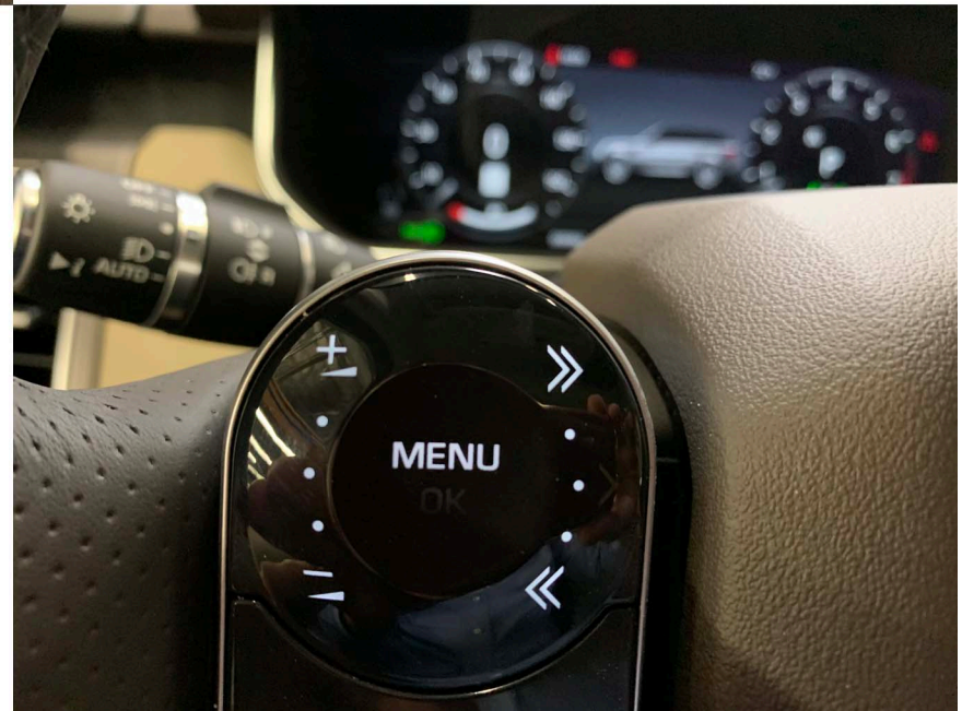
Figure A14. Controls for Changing Vehicle Parameters
