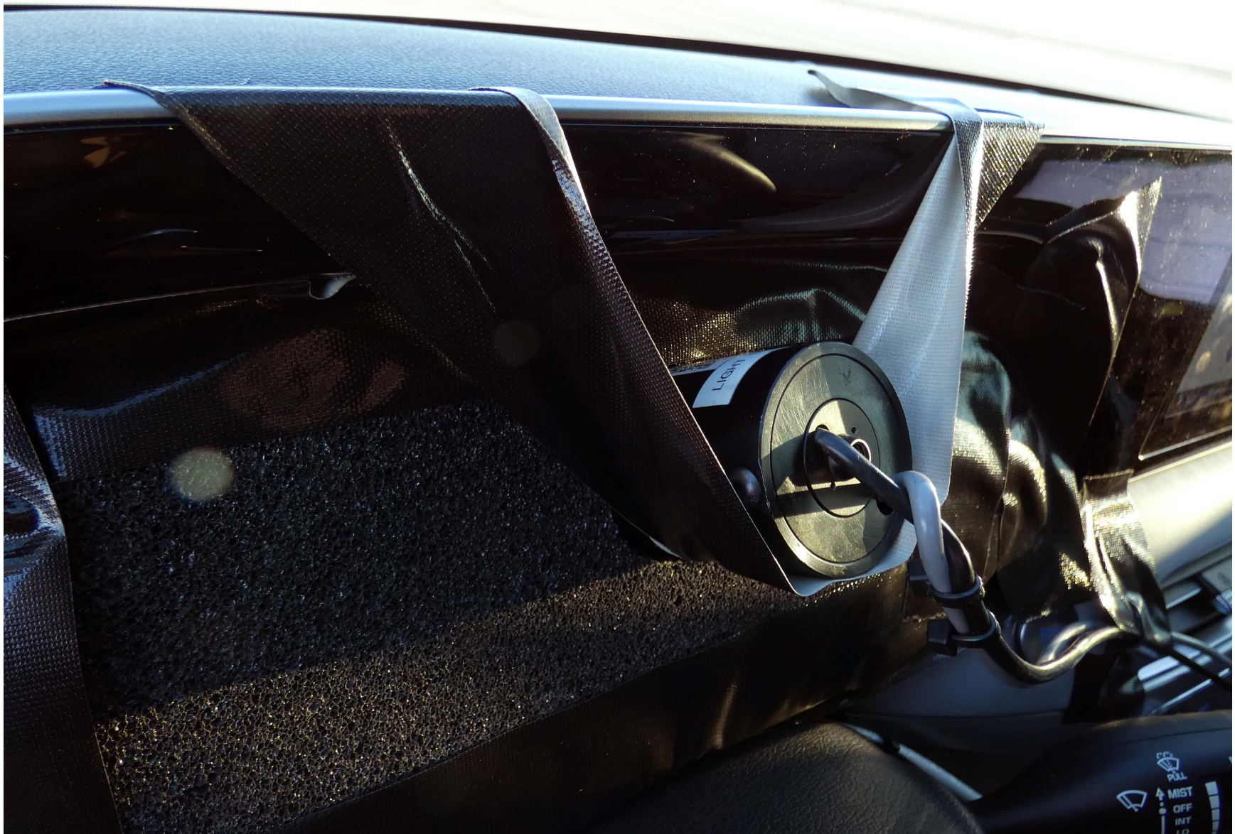
Figure A12. Sensor for Detecting Visual Alert
