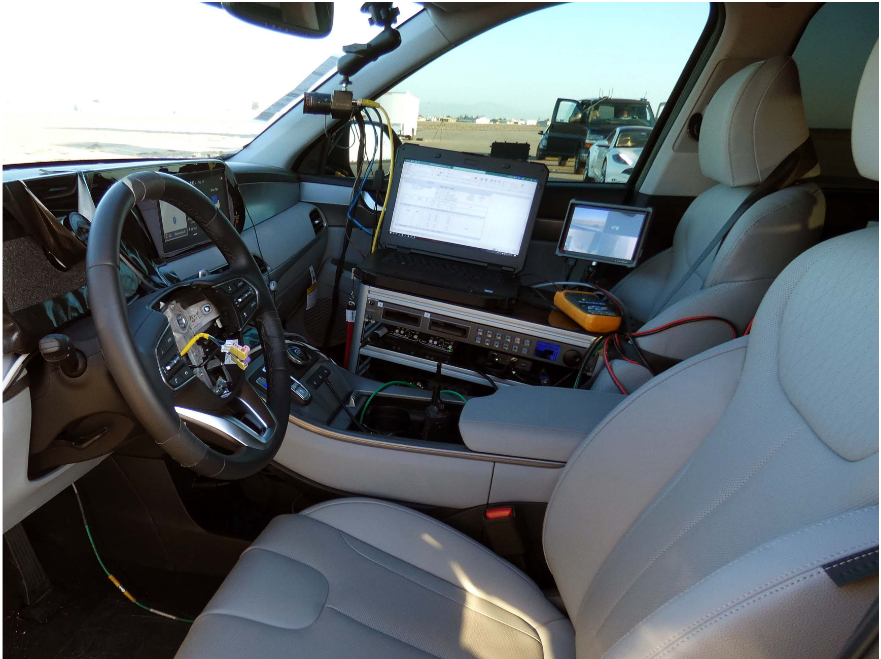
Figure A13. Computer Installed in Subject Vehicle
