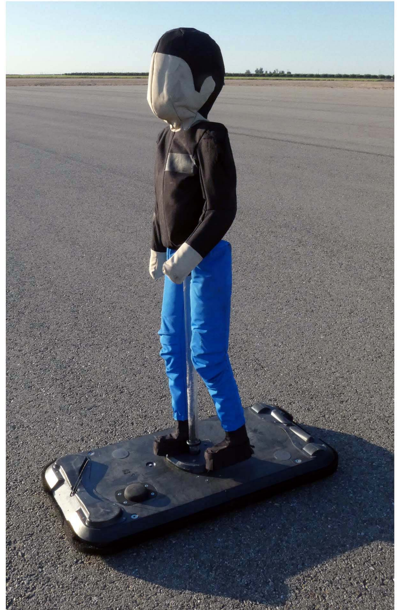
Figure A8. Adult and Child Pedestrian Surrogates and Motion Platform
