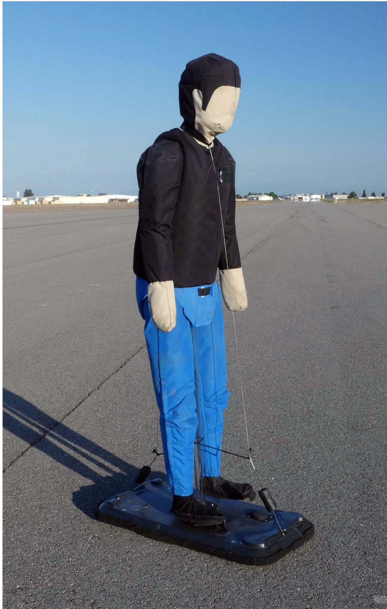
Figure A8. Adult and Child Pedestrian Surrogates and Motion Platform
