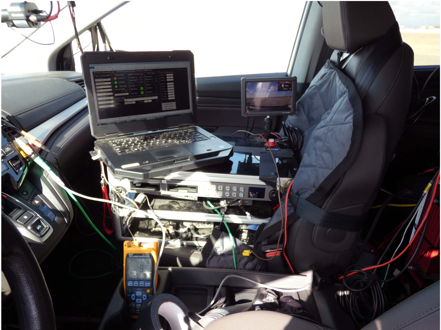
Figure A12. Computer Installed in Subject Vehicle
