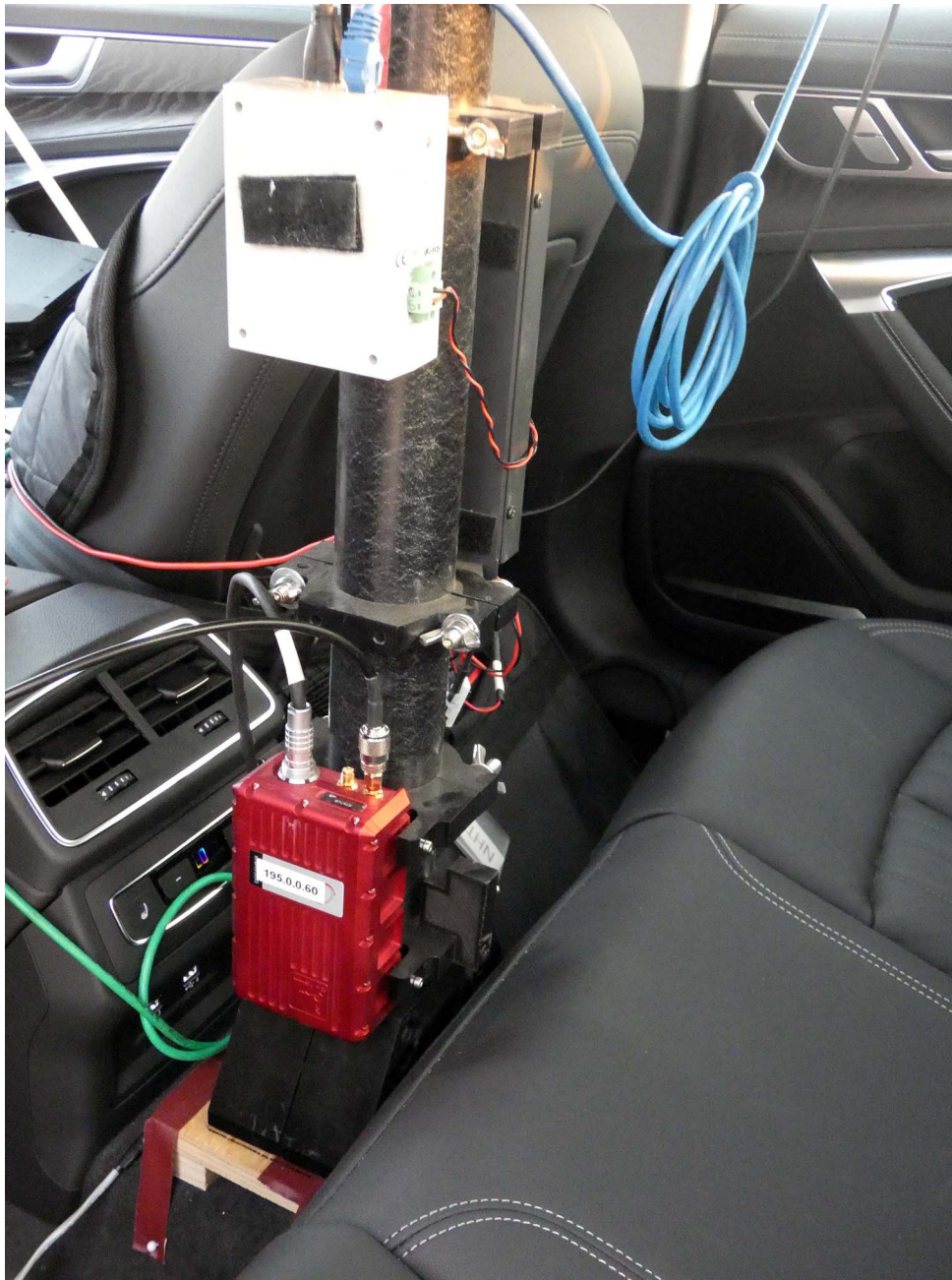
Figure A10. DGPS, Inertial Measurement Unit, and MicroAutoBox Installed in Subject Vehicle
