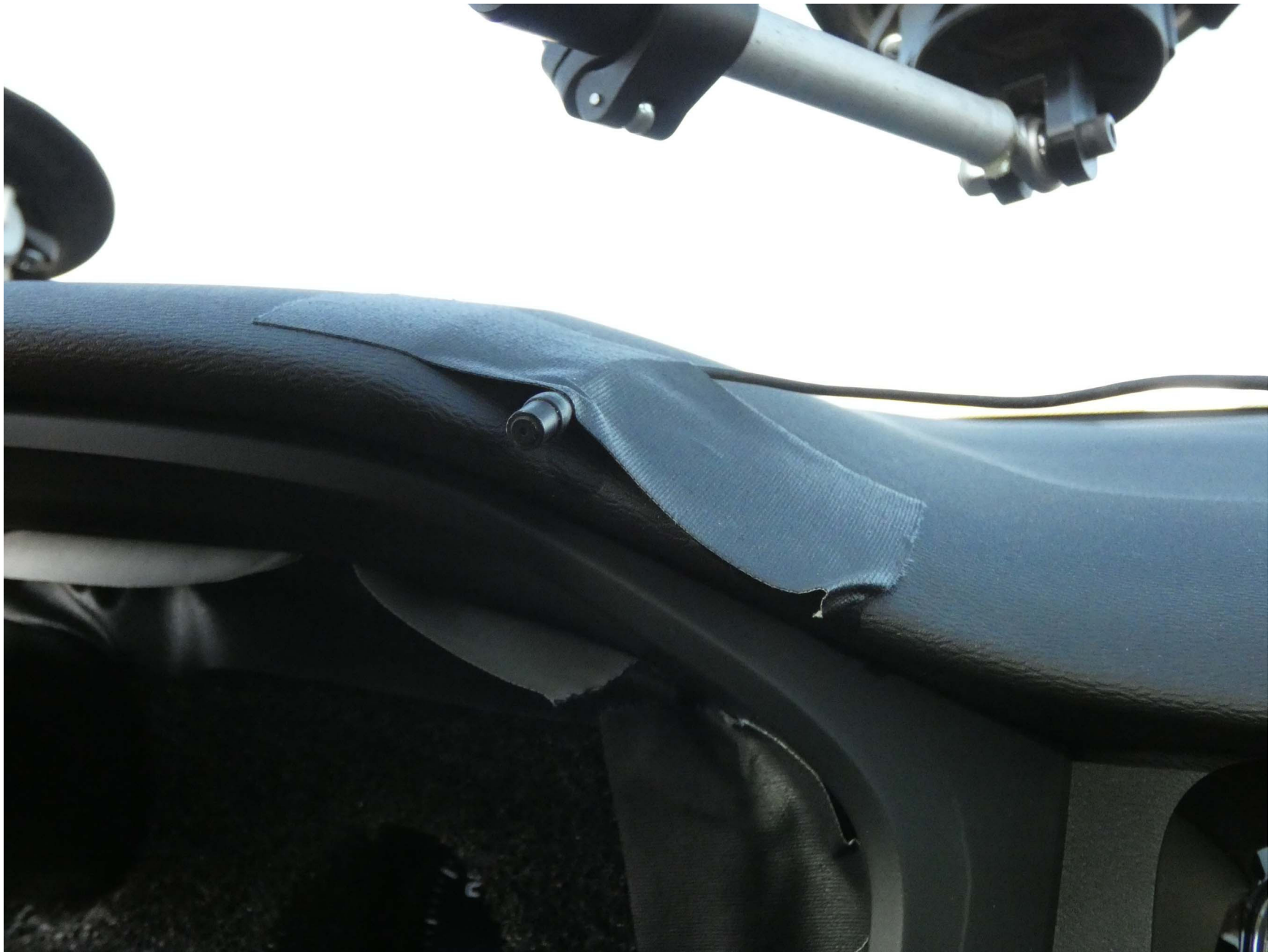
Figure A9. Sensors for Detecting Auditory Alerts
