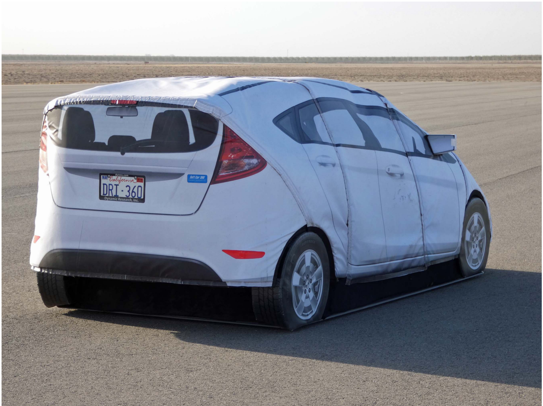
Figure A7. Rear View of Principal Other Vehicle: Global Vehicle Target
