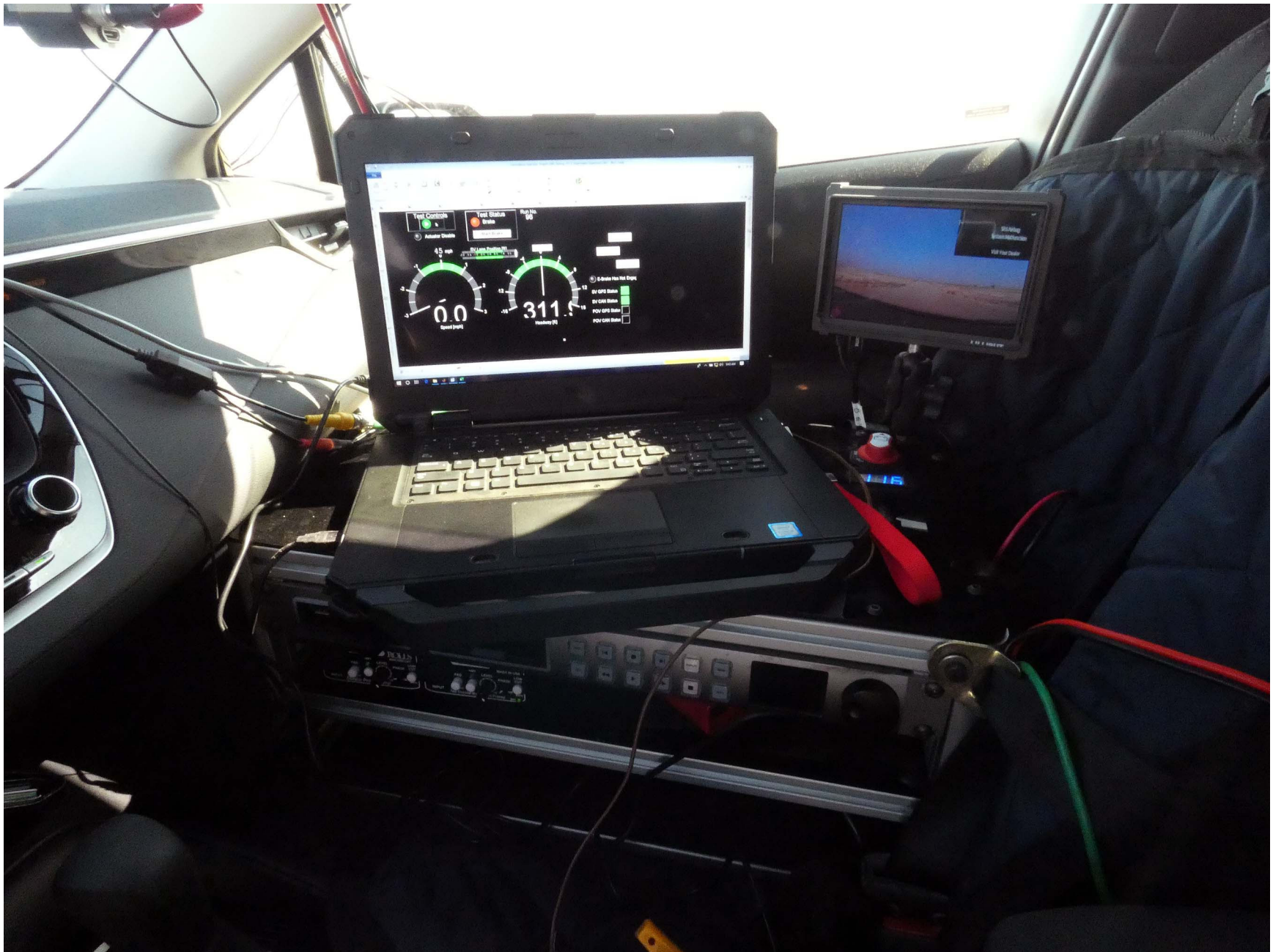
Figure A11. Computer Installed in Subject Vehicle
