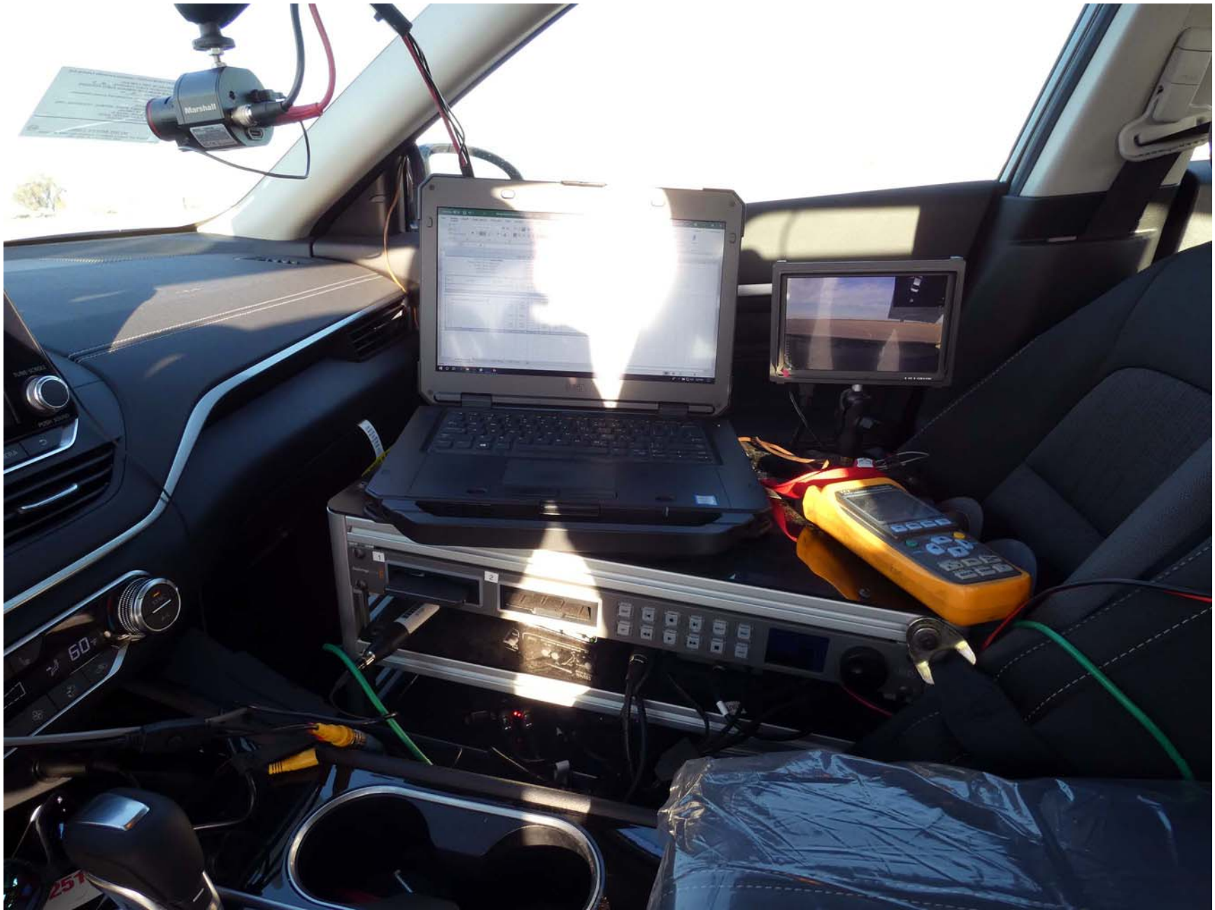
Figure A11. Computer Installed in Subject Vehicle
