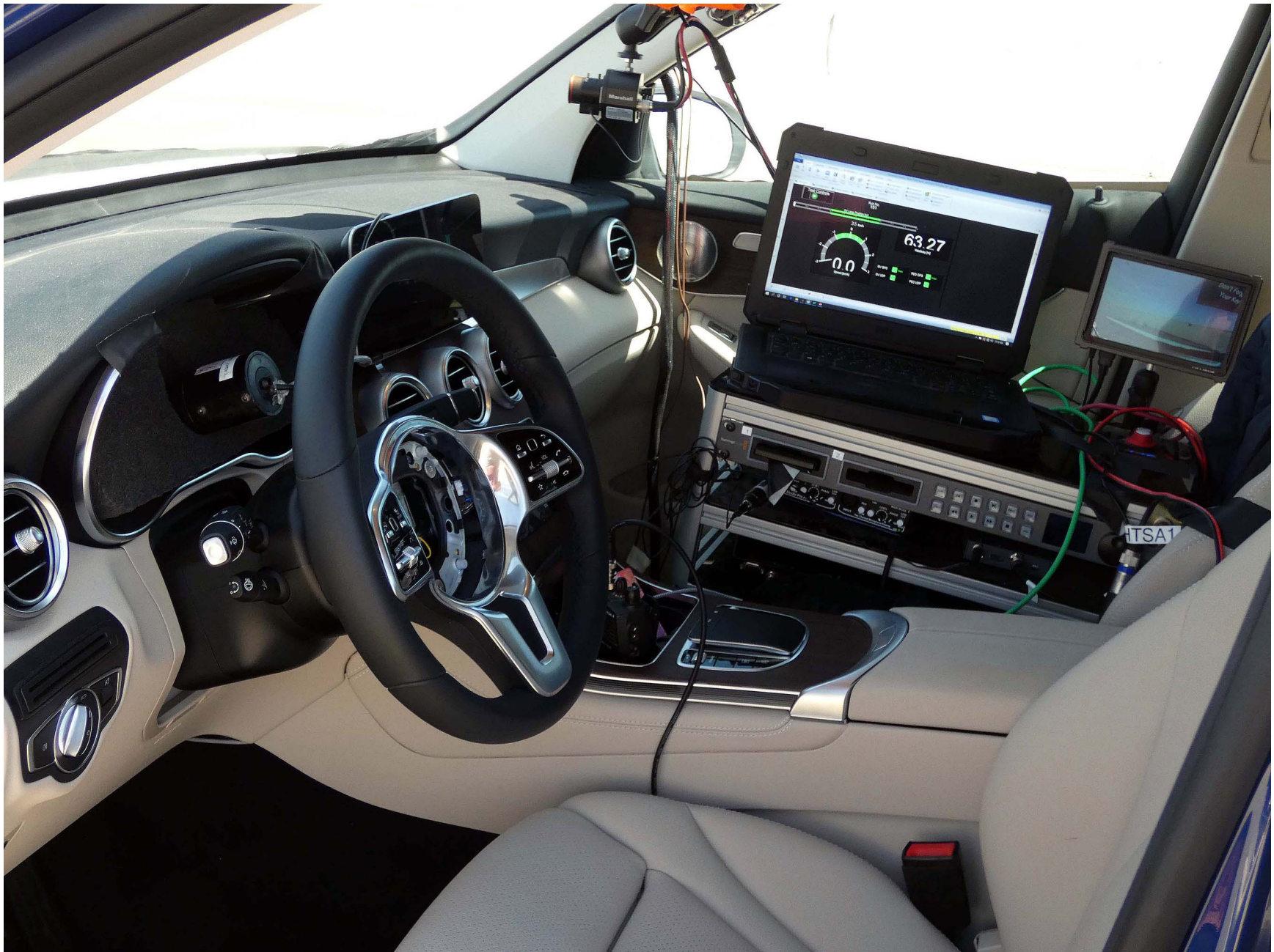
Figure A10. Computer Installed in Subject Vehicle
