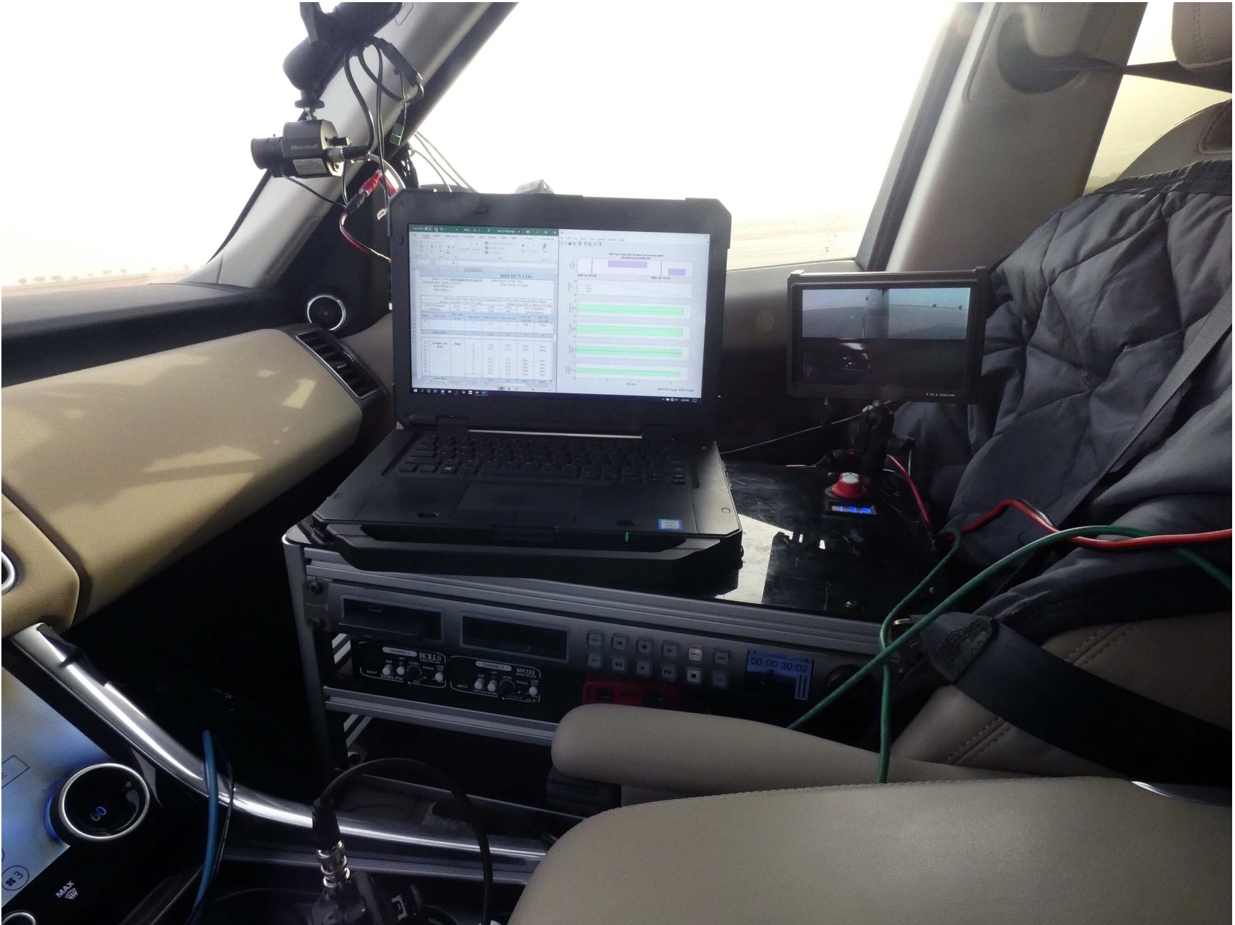
Figure A10. Computer Installed in Subject Vehicle
