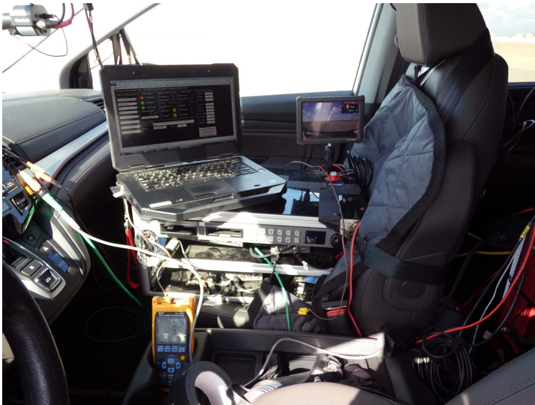
Figure A11. Computer Installed in Subject Vehicle
