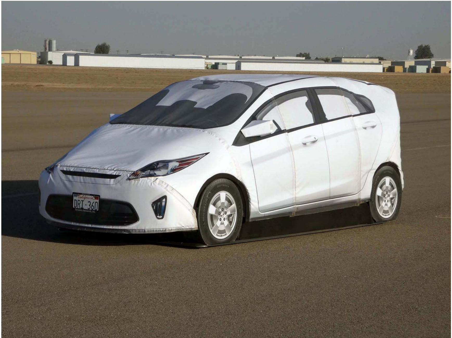
Figure A6. Front View of Principal Other Vehicle: Global Vehicle Target
