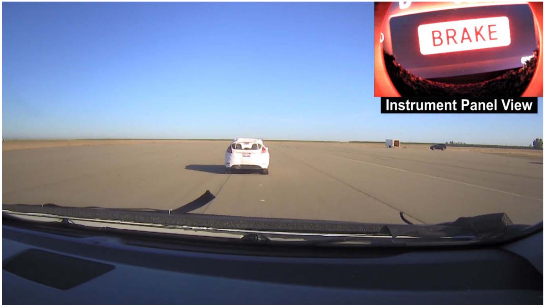
Figure A14. CIB (CMBS) Visual Alert shown as Inset in Out-the-Window View
