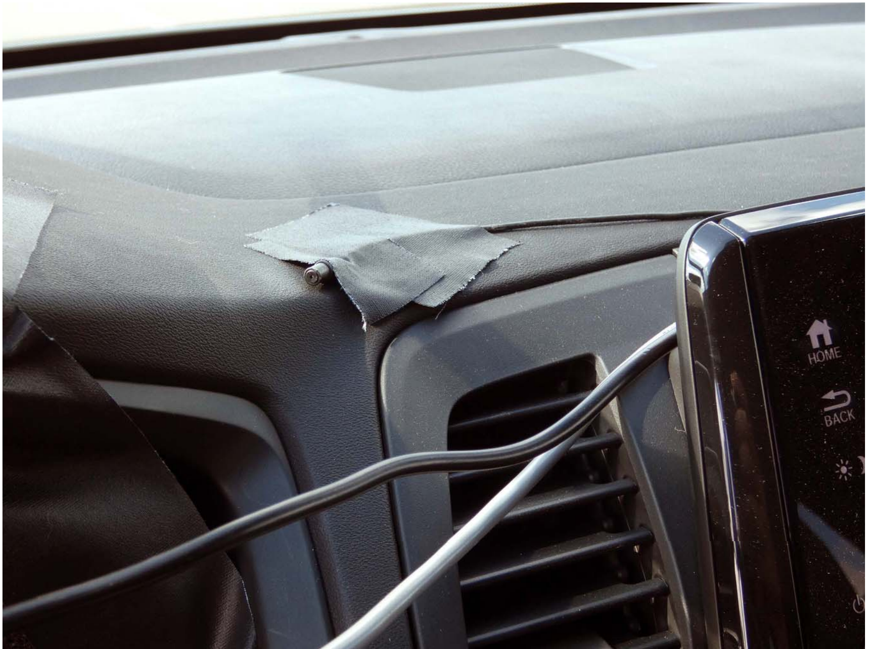
Figure A9. Sensor for Detecting Auditory Alerts
