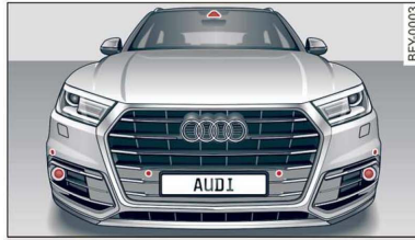
Fig. 110 Front of the vehicle: sensors and video camera
