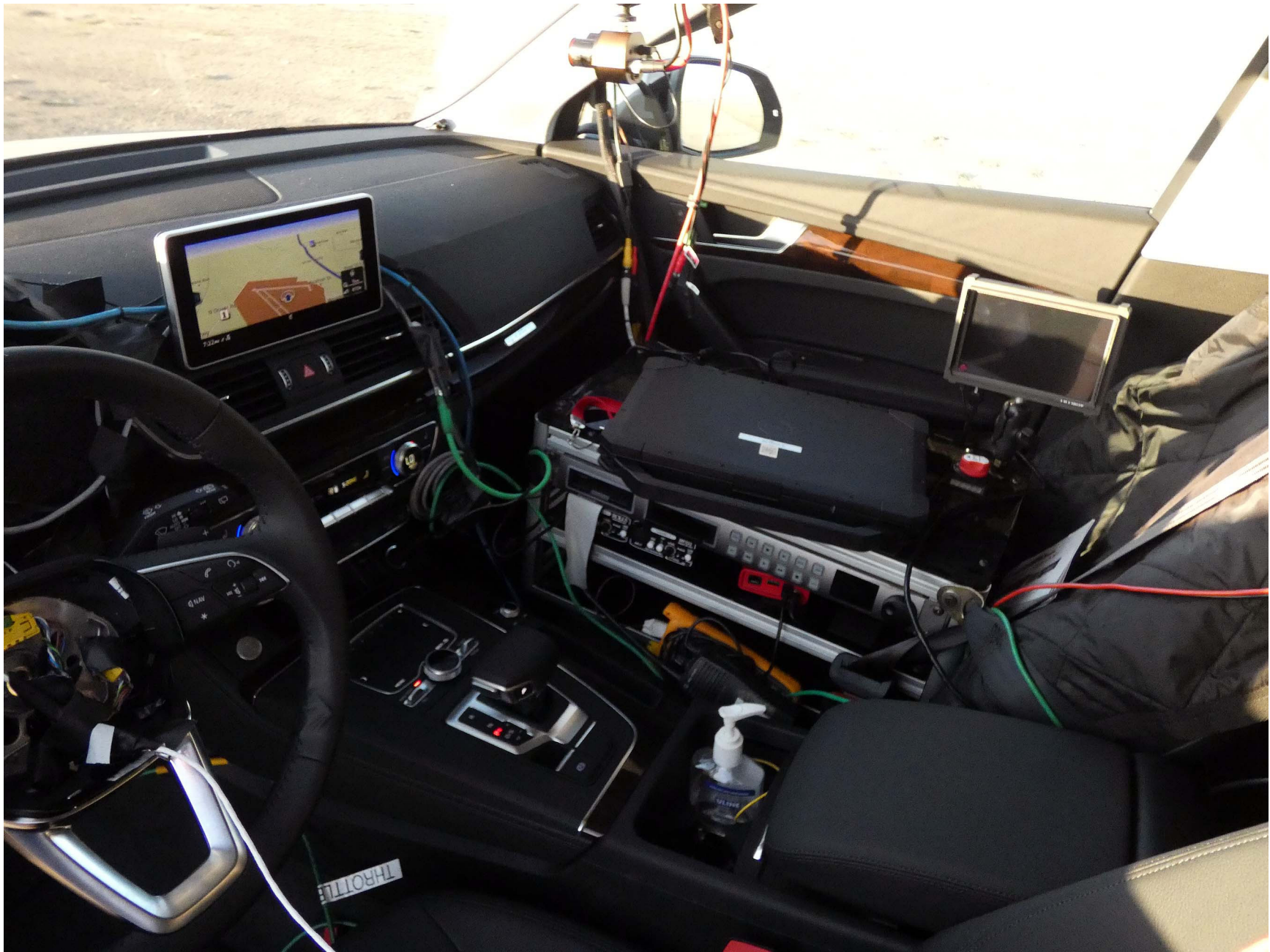
Figure A10. Computer Installed in Subject Vehicle
