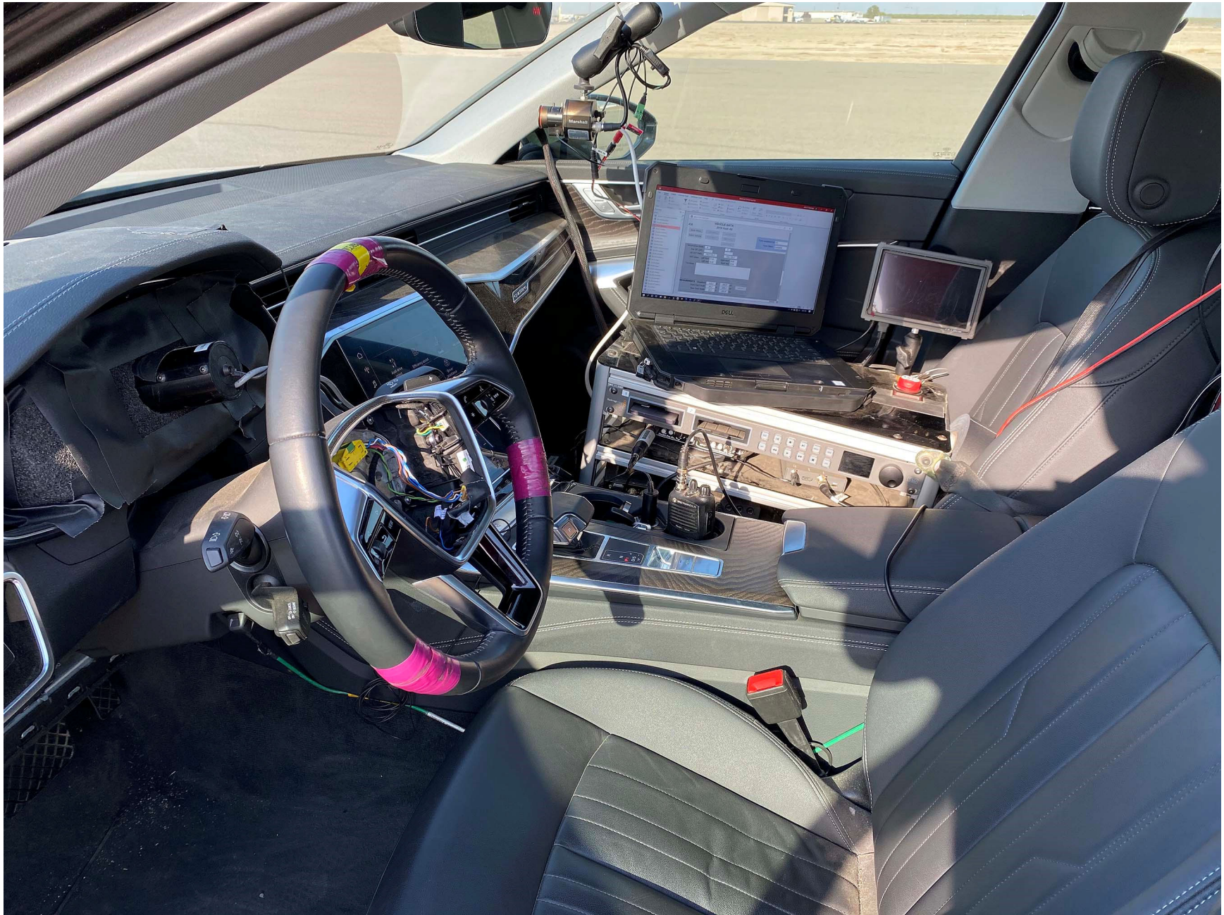
Figure A10. Computer Installed in Subject Vehicle
