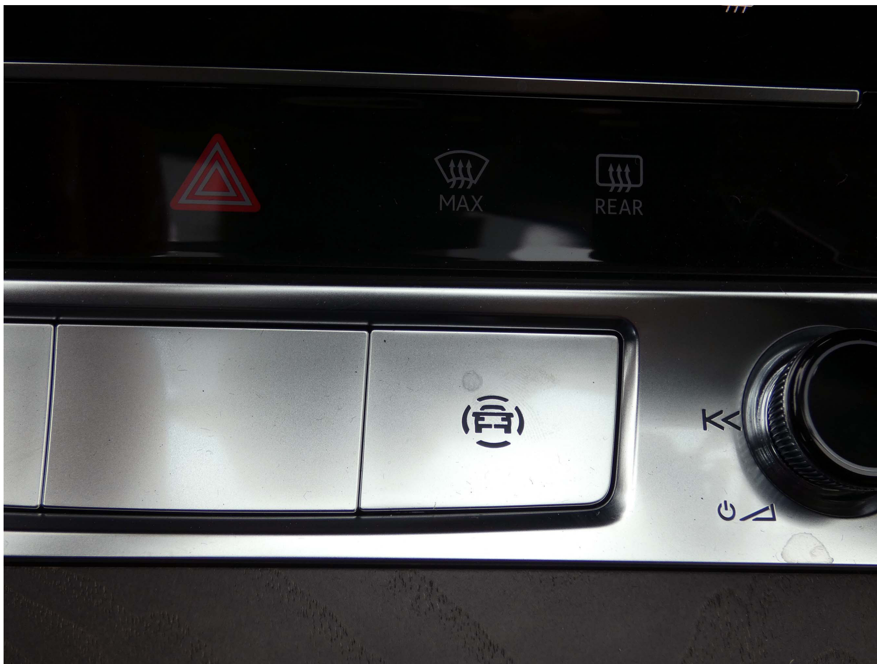
Figure A13. Button for Directly Accessing Driver Assistance Settings Menus
