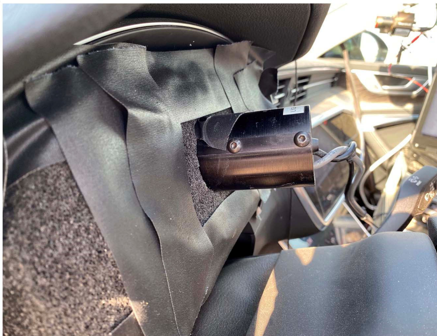
Figure A9. Sensors for Detecting Auditory and Visual Alerts
