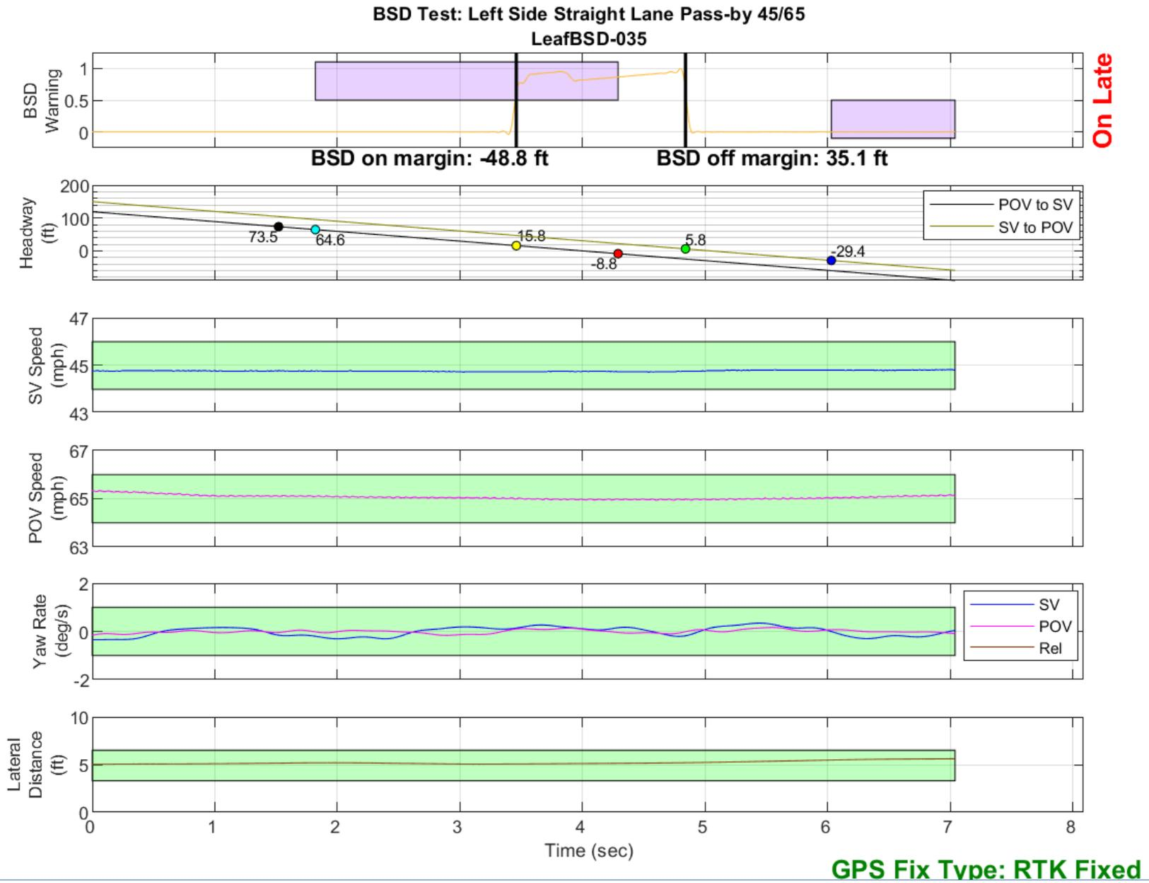
Figure D68. BSD Run 35, Straight Lane Pass-by, SV 45 mph, POV 65 mph
