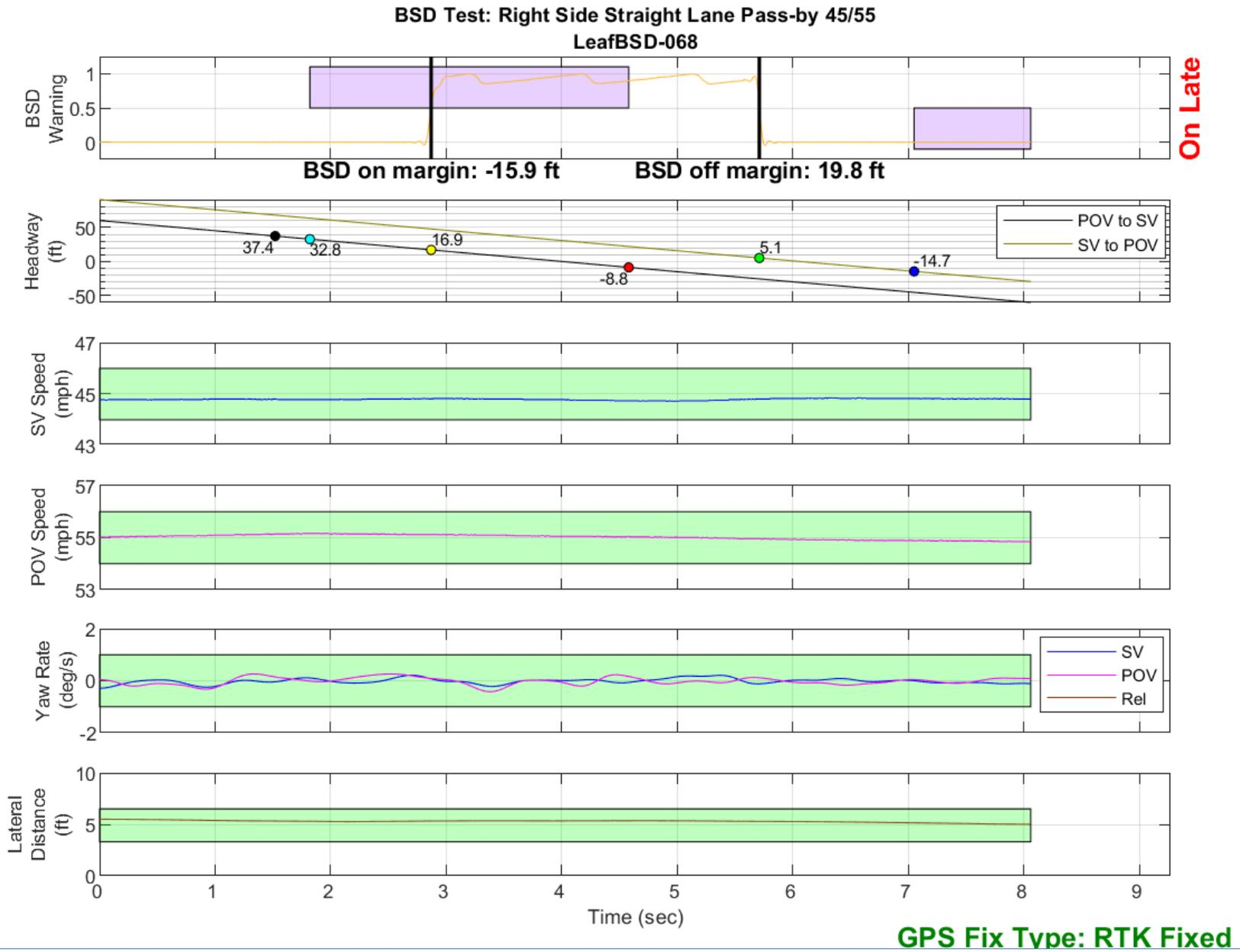
Figure D39. BSD Run 68, Straight Lane Pass-by, SV 45 mph, POV 55 mph
