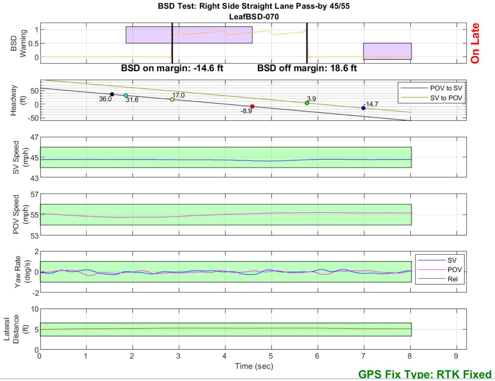
Figure D41. BSD Run 70, Straight Lane Pass-by, SV 45 mph, POV 55 mph
