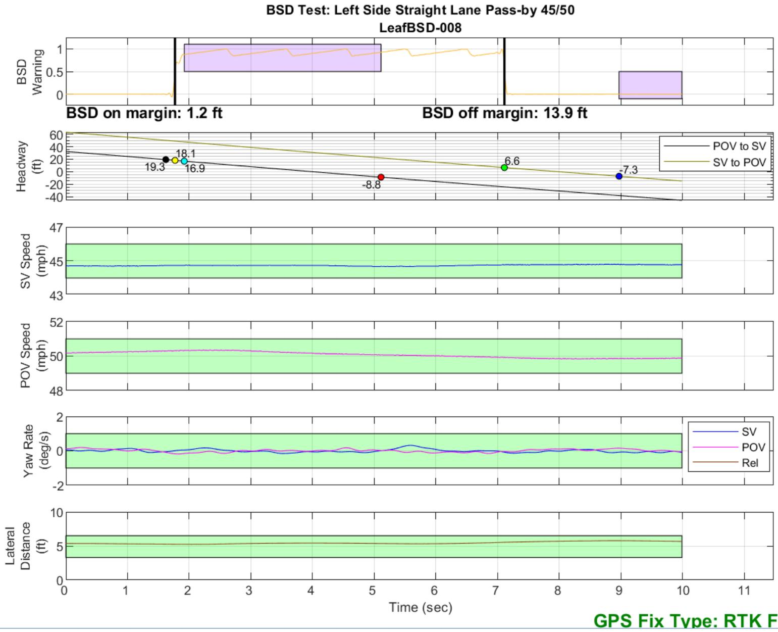
Figure D22. BSD Run 8, Straight Lane Pass-by, SV 45 mph, POV 50 mph
