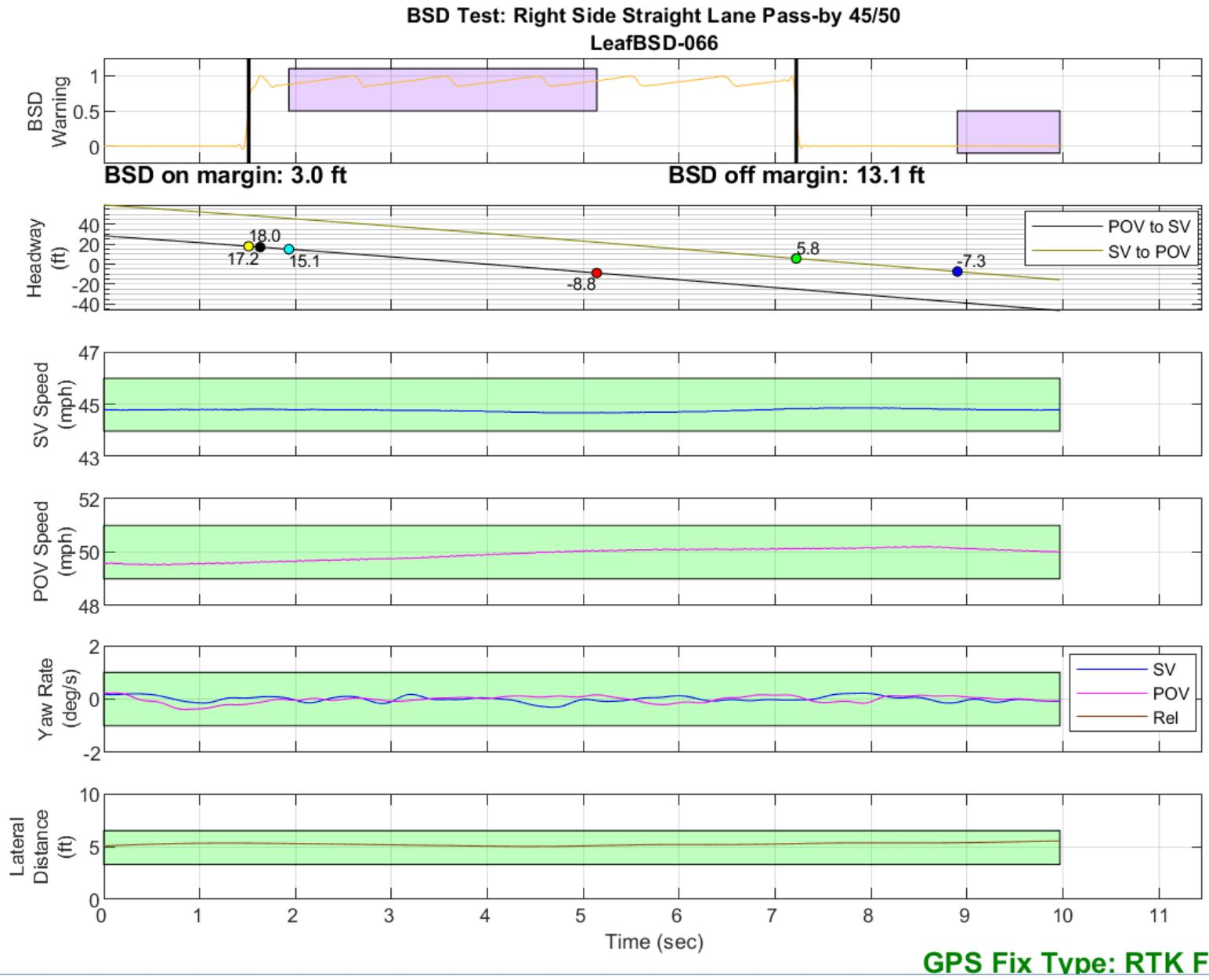
Figure D30. BSD Run 66, Straight Lane Pass-by, SV 45 mph, POV 50 mph
