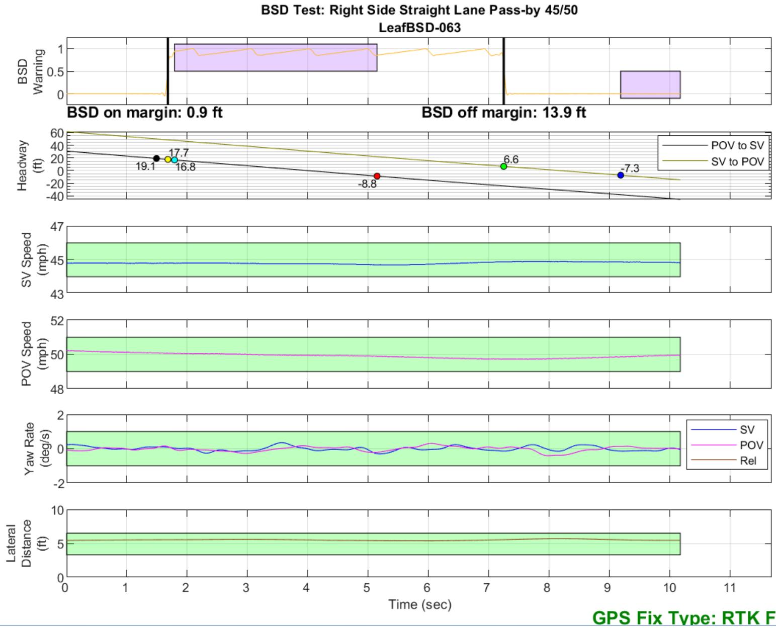
Figure D27. BSD Run 63, Straight Lane Pass-by, SV 45 mph, POV 50 mph
