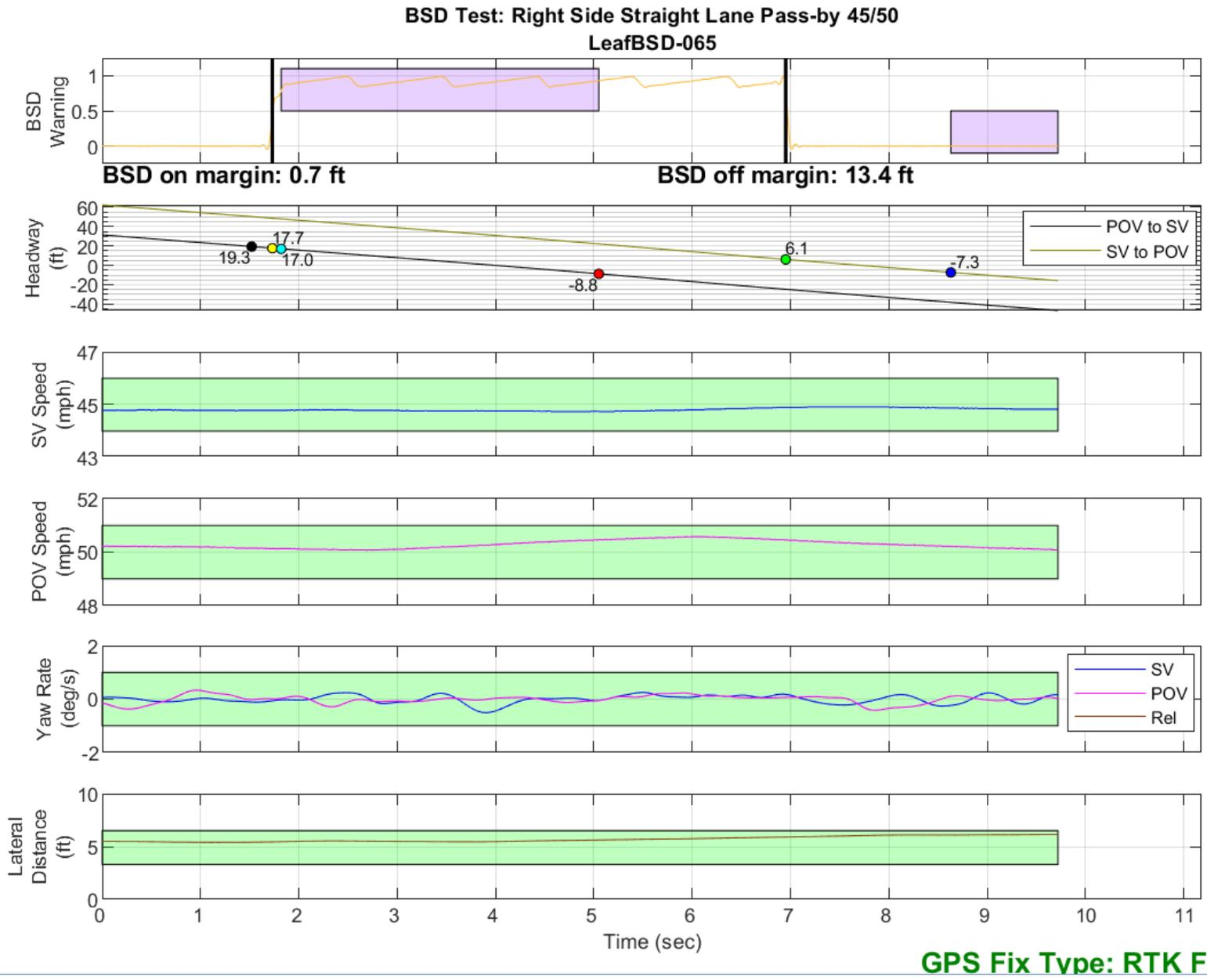
Figure D29. BSD Run 65, Straight Lane Pass-by, SV 45 mph, POV 50 mph
