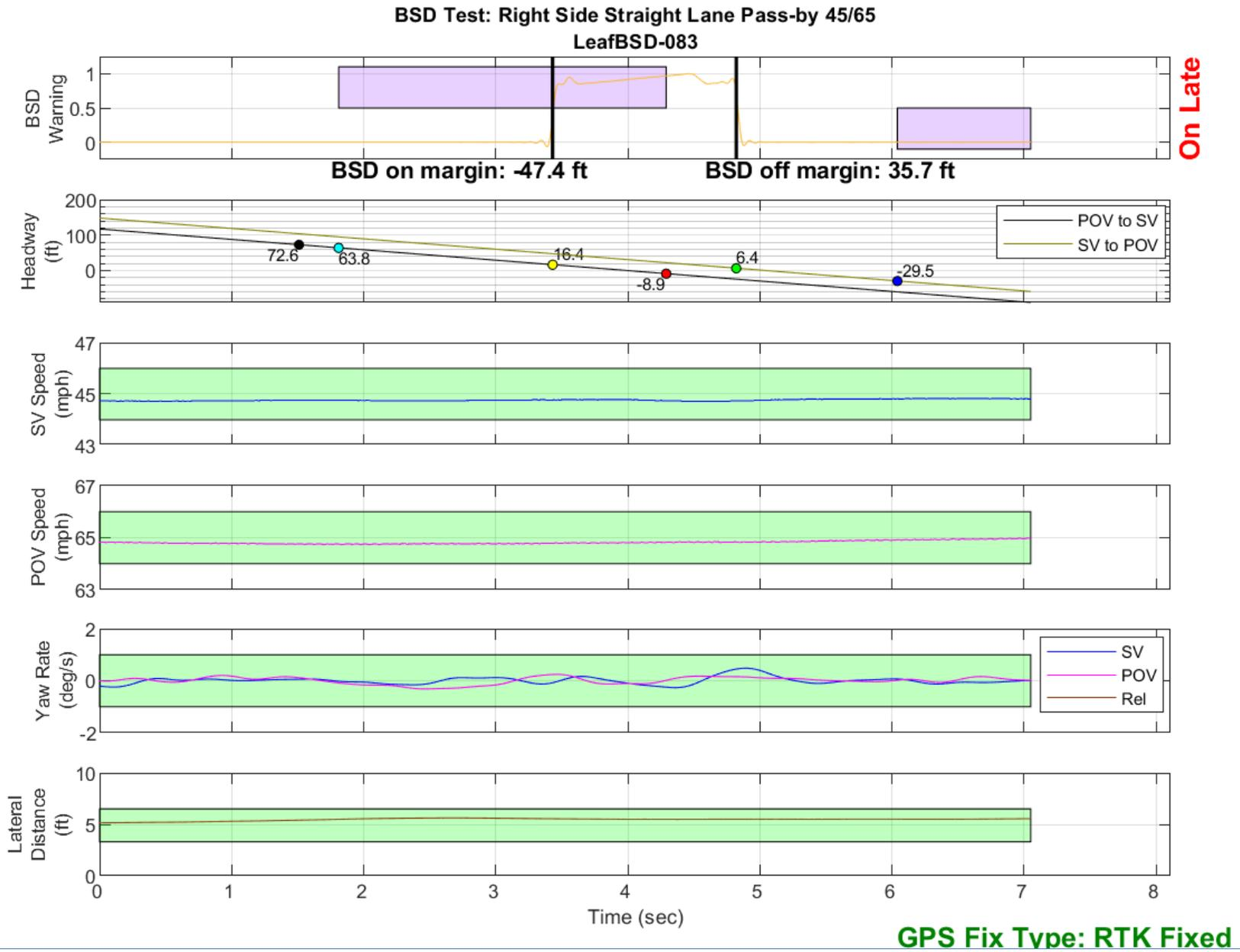
Figure D70. BSD Run 83, Straight Lane Pass-by, SV 45 mph, POV 65 mph
