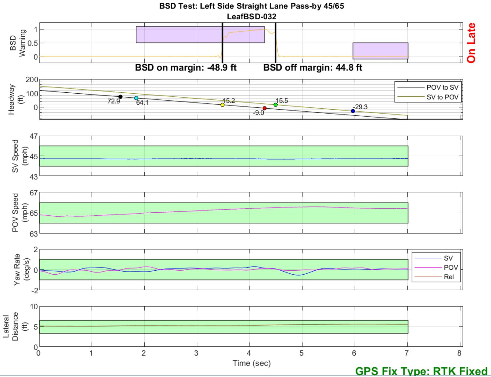
Figure D66. BSD Run 32, Straight Lane Pass-by, SV 45 mph, POV 65 mph
