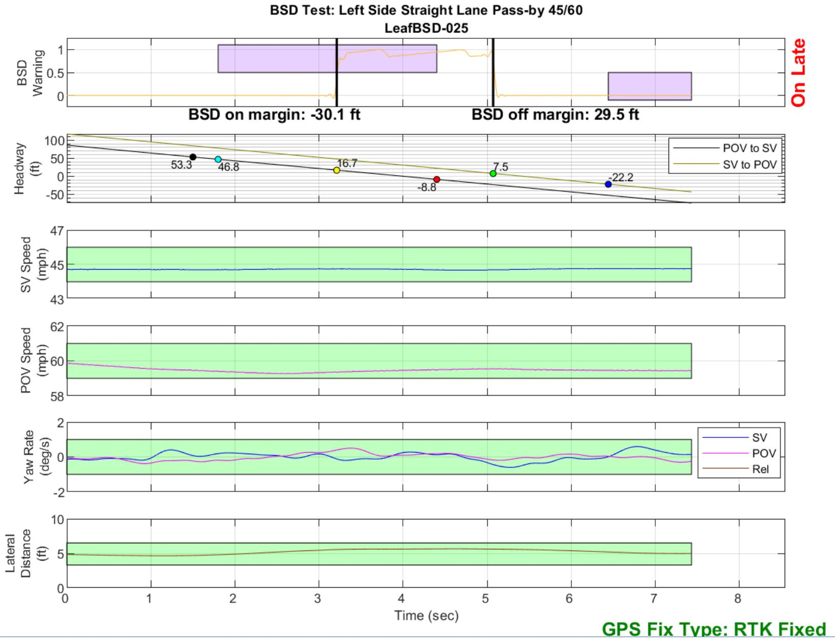
Figure D52. BSD Run 25, Straight Lane Pass-by, SV 45 mph, POV 60 mph
