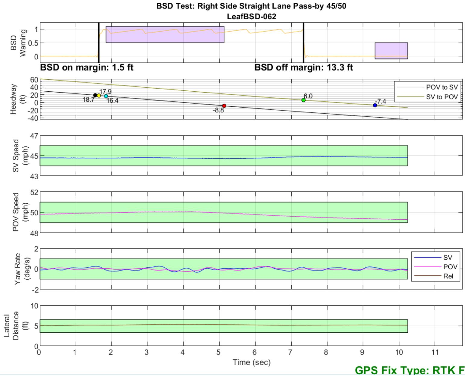
Figure D26. BSD Run 62, Straight Lane Pass-by, SV 45 mph, POV 50 mph
