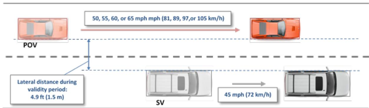
Figure 2. Straight Lane Pass-by Test
