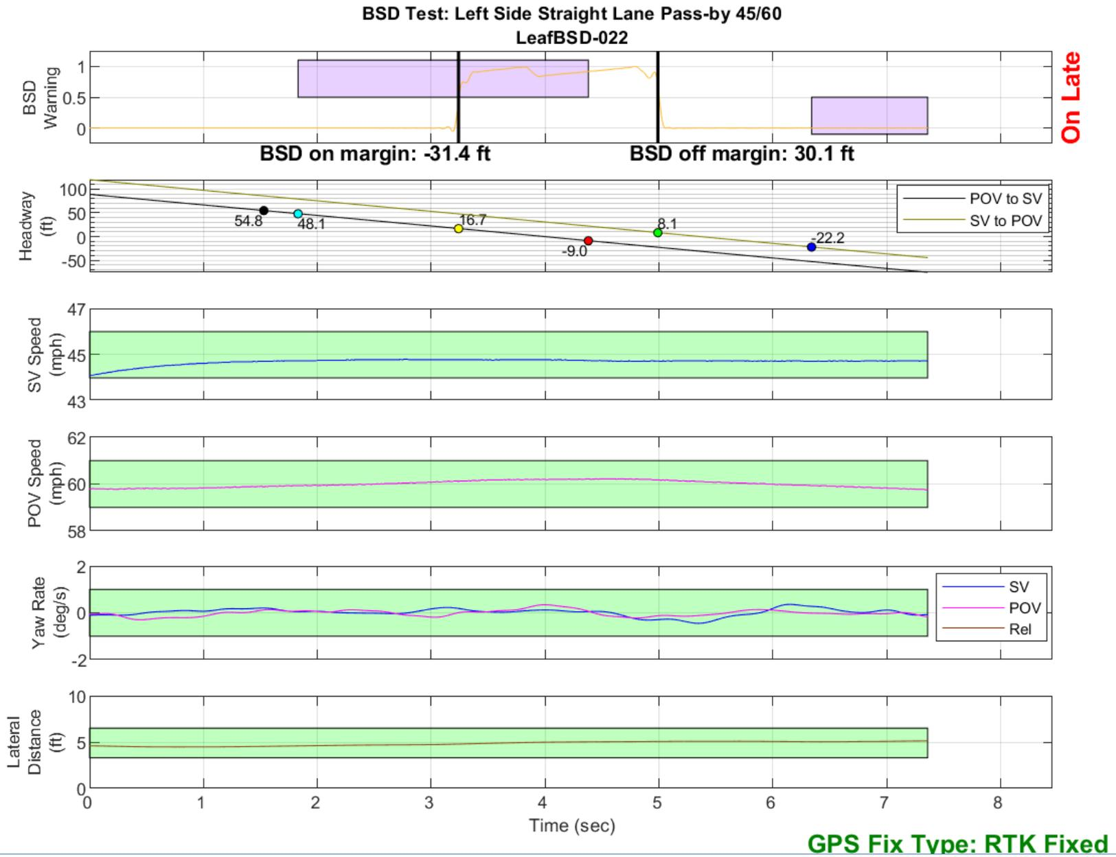
Figure D49. BSD Run 22, Straight Lane Pass-by, SV 45 mph, POV 60 mph
