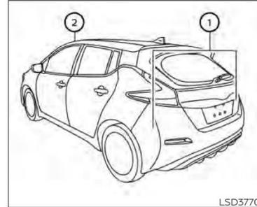
The I-BSI system uses radar sensors ① installed near the rear bumper to detect other vehicles in an adjacent lane. In addition to the radar sensors, the I-BSI system uses a camera ② installed behind the windshield to monitor the lane markers of your traveling lane.
