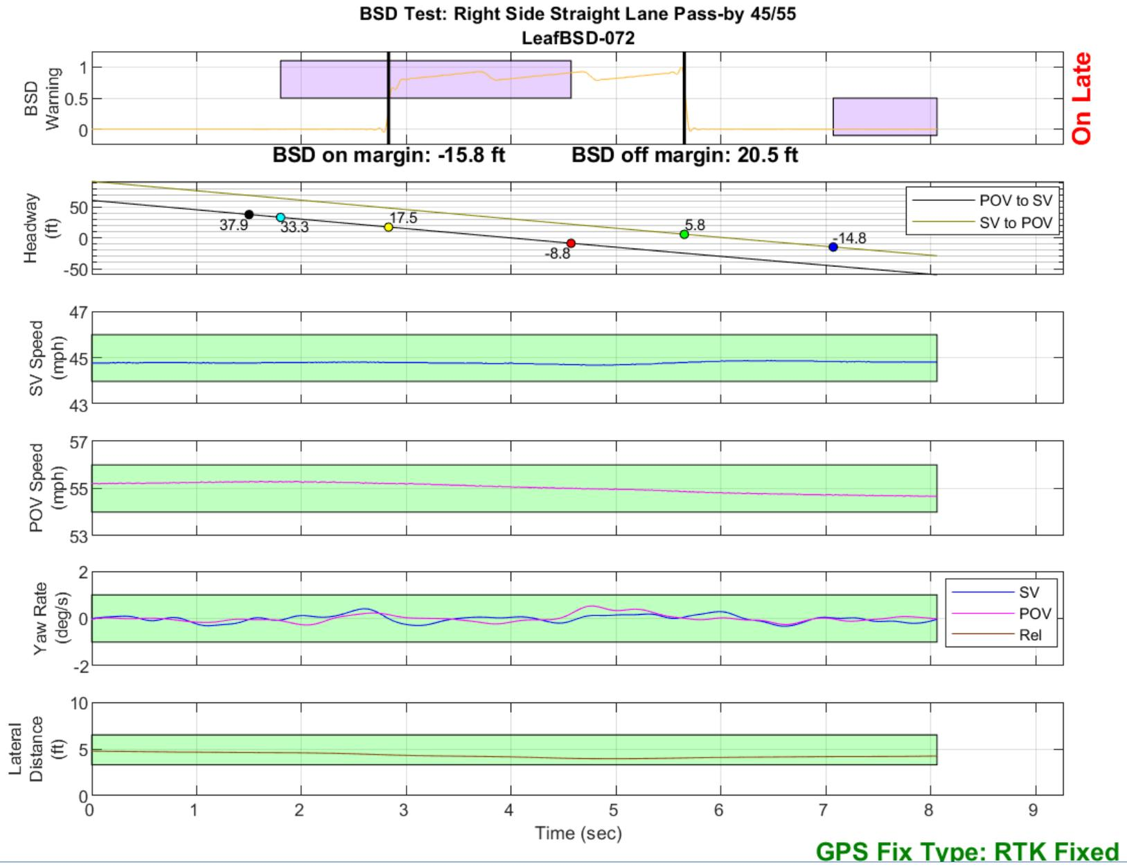
Figure D43. BSD Run 72, Straight Lane Pass-by, SV 45 mph, POV 55 mph
