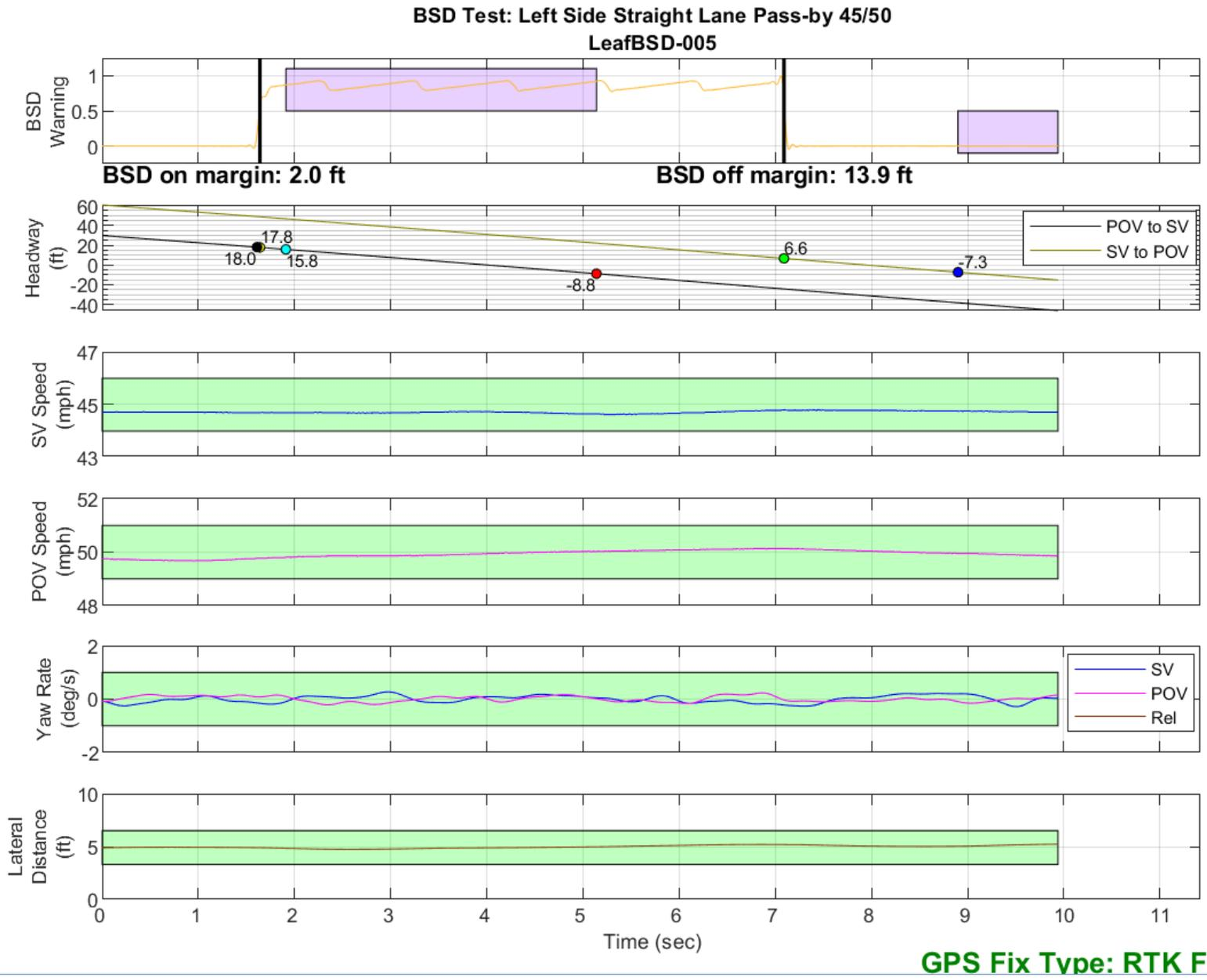
Figure D19. BSD Run 5, Straight Lane Pass-by, SV 45 mph, POV 50 mph
