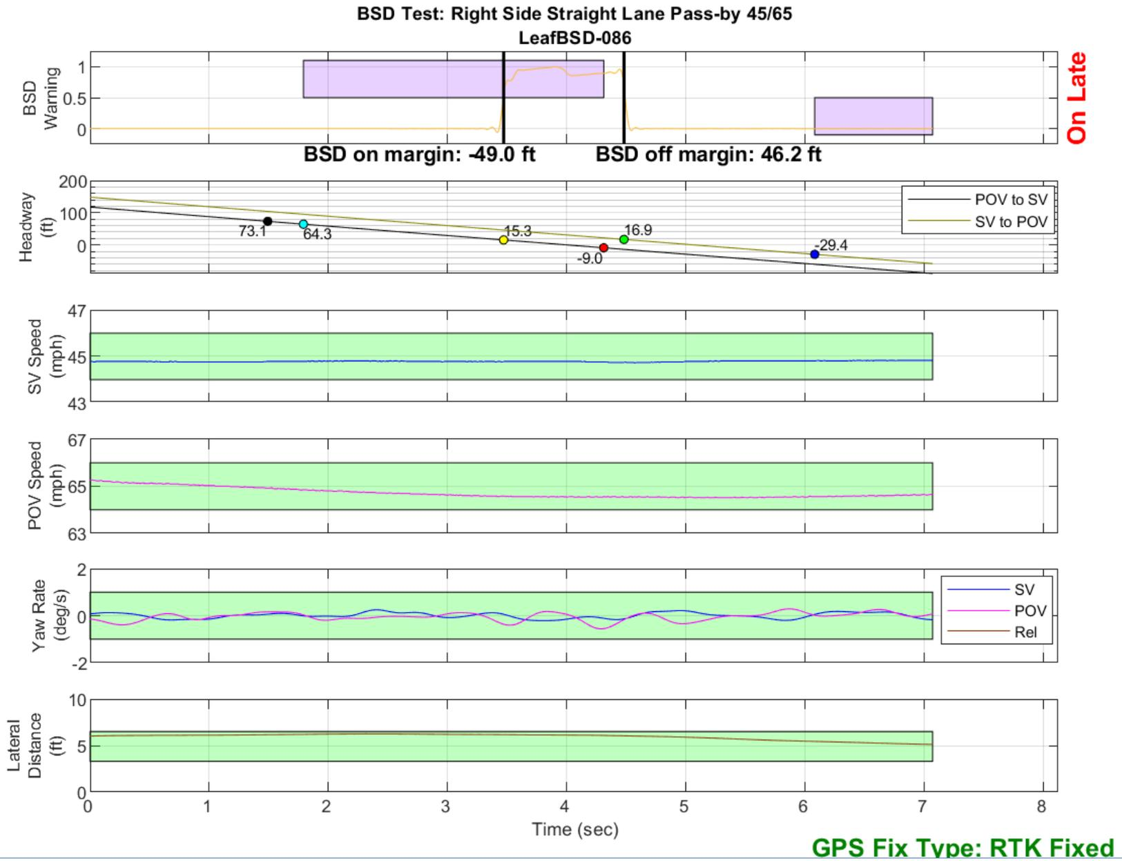
Figure D73. BSD Run 86, Straight Lane Pass-by, SV 45 mph, POV 65 mph
