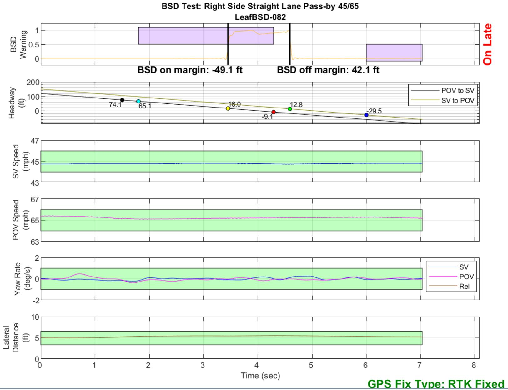
Figure D69. BSD Run 82, Straight Lane Pass-by, SV 45 mph, POV 65 mph
