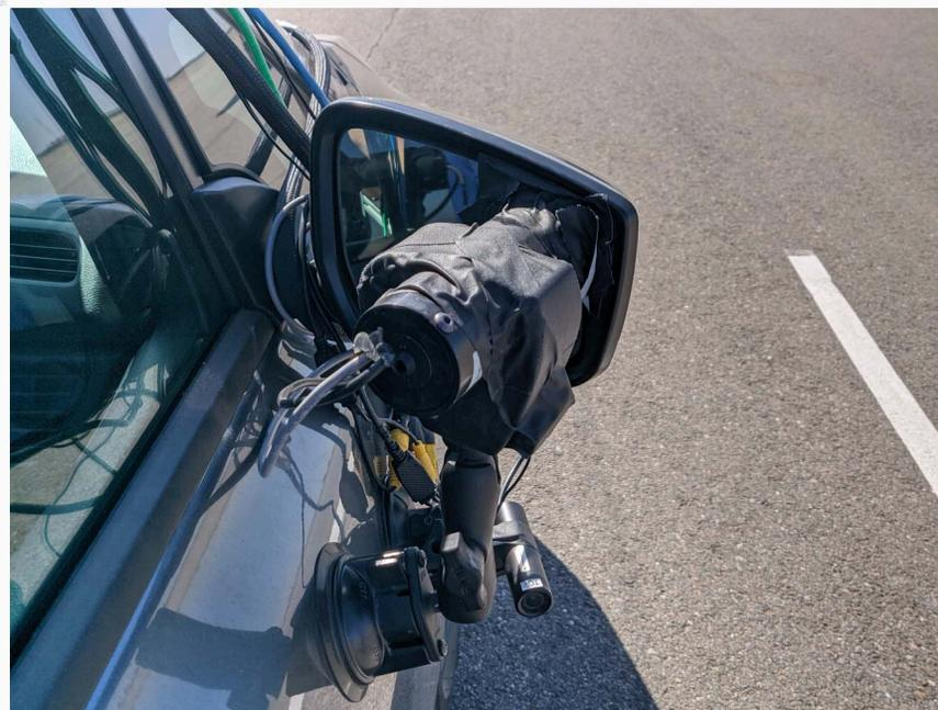
Figure A9. Sensors for Detecting Visual Alerts
