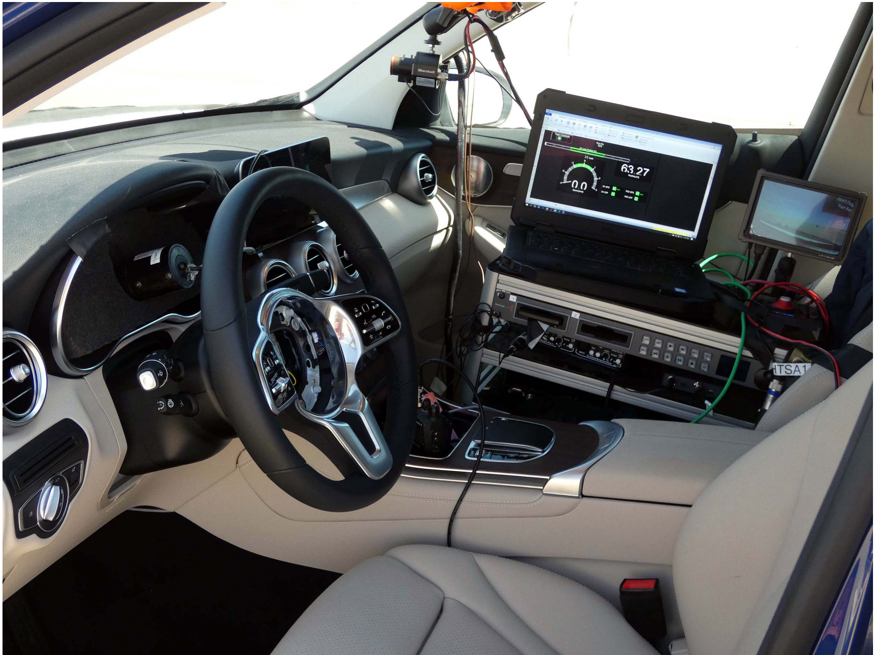
Figure A10. Computer Installed in Subject Vehicle
