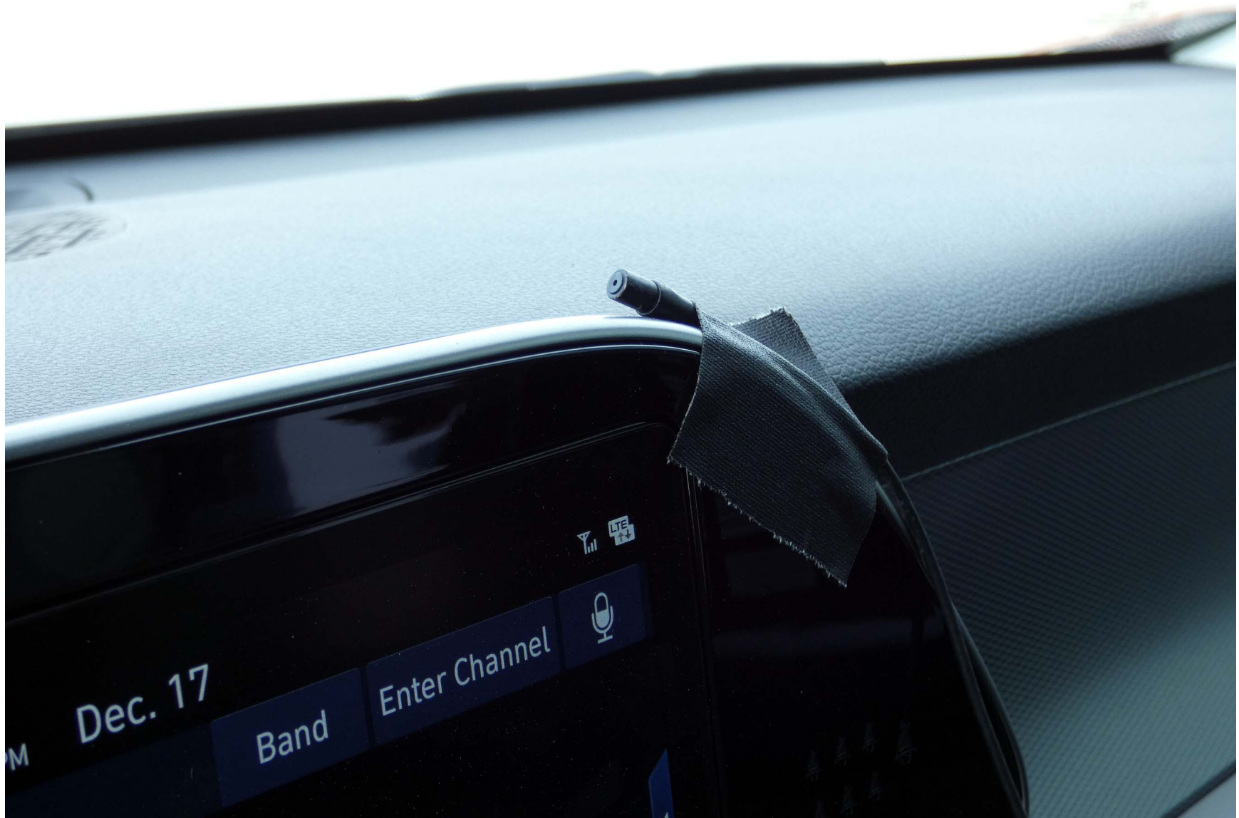
Figure A10. Sensor for Detecting Auditory Alerts
