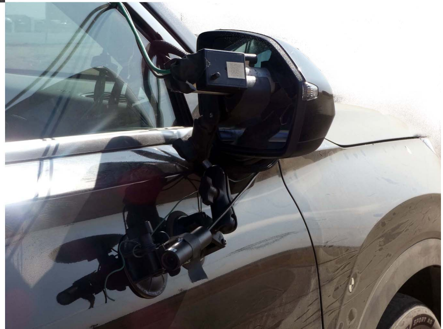
Figure A9. Sensors for Detecting Visual Alerts
