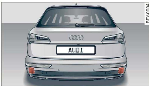
Fig. 131 Rear of the vehicle: sensor locations
