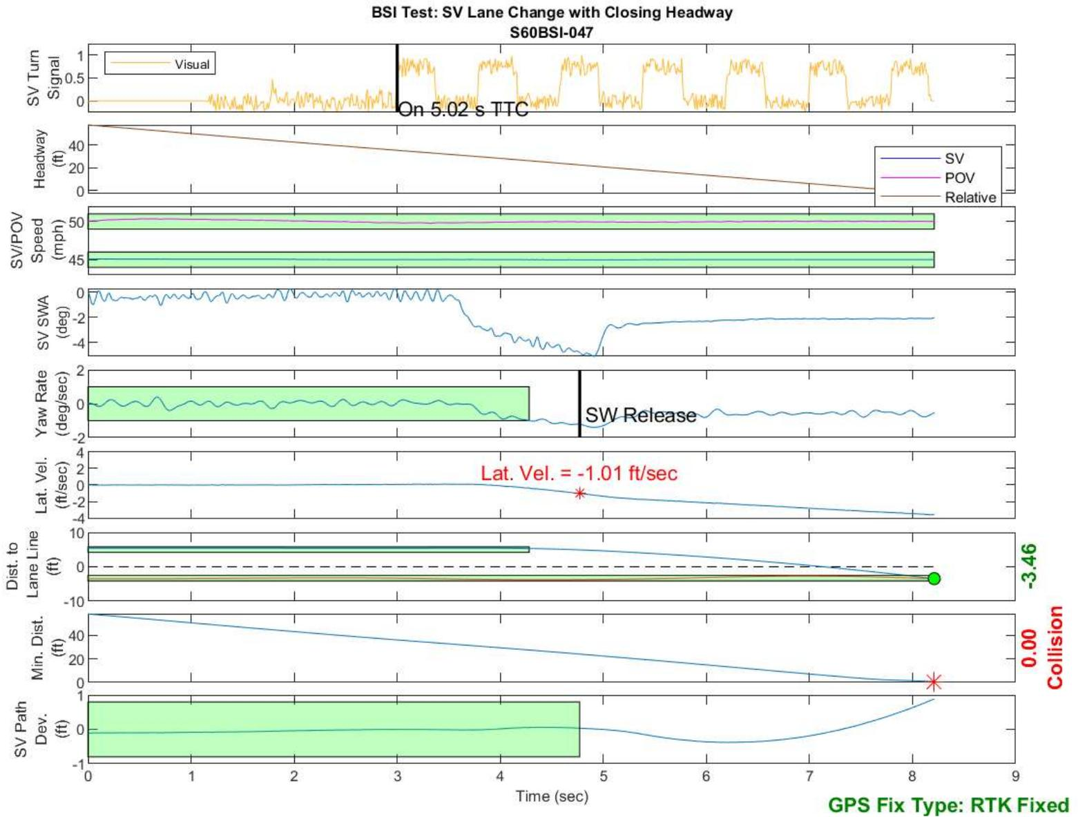
Figure D17. BSI Run 47, Subject Vehicle Lane Change with Closing Headway
