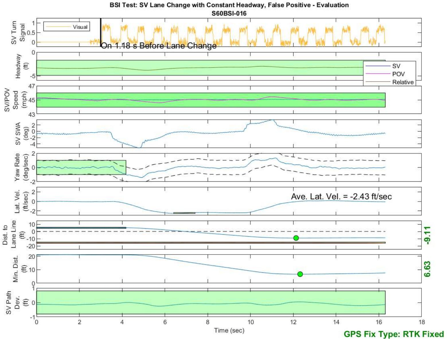
Figure D29. BSI Run 16, Subject Vehicle Lane Change with Constant Headway, False Positive Assessment - Evaluation
