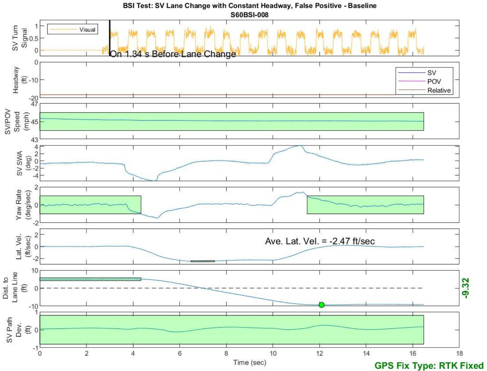
Figure D24. BSI Run 8, Subject Vehicle Lane Change with Constant Headway, False Positive Assessment - Baseline
