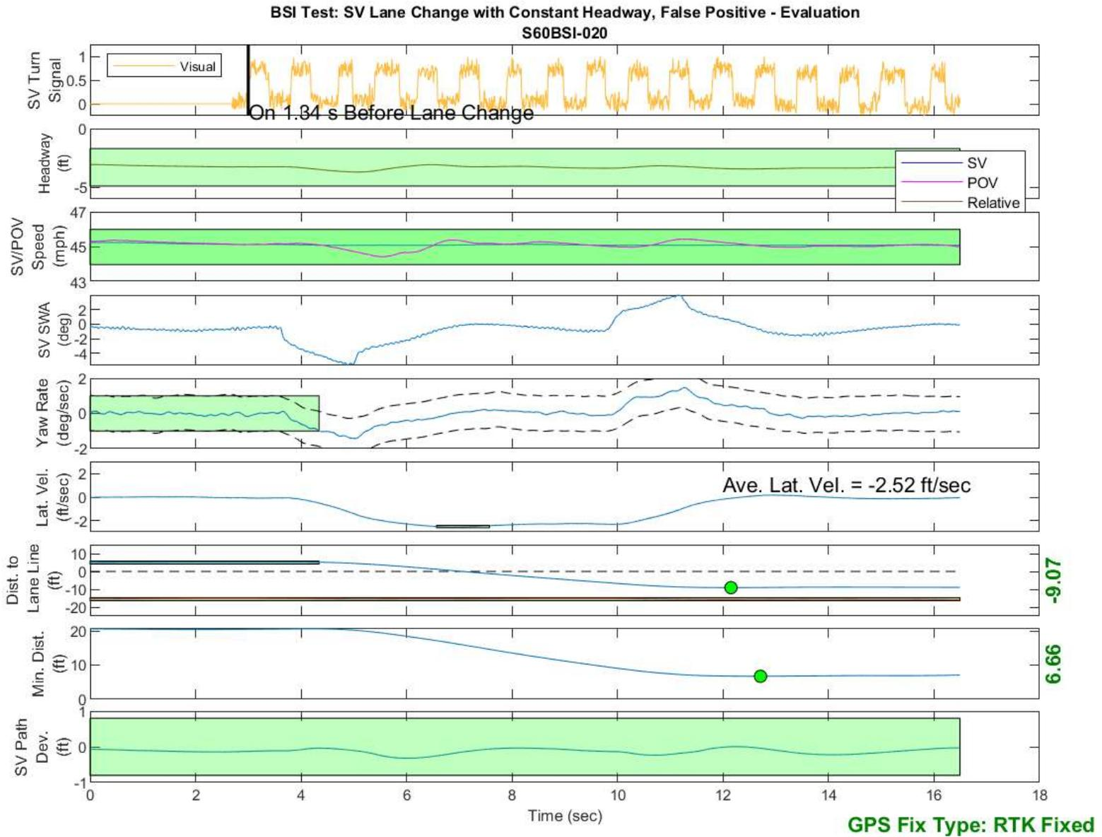
Figure D31. BSI Run 20, Subject Vehicle Lane Change with Constant Headway, False Positive Assessment - Evaluation
