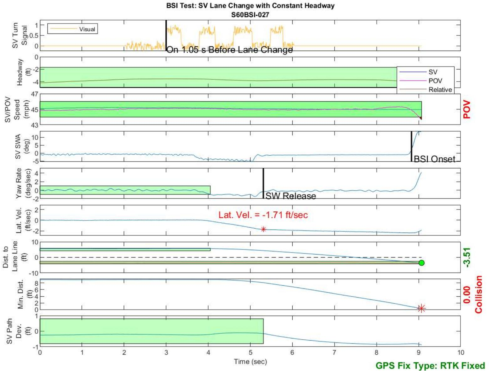
Figure D8. BSI Run 27, Subject Vehicle Lane Change with Constant Headway
