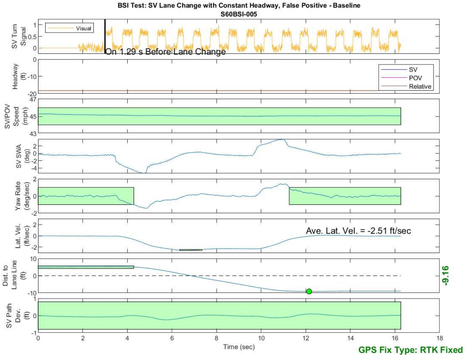
Figure D21. BSI Run 5, Subject Vehicle Lane Change with Constant Headway, False Positive Assessment - Baseline
