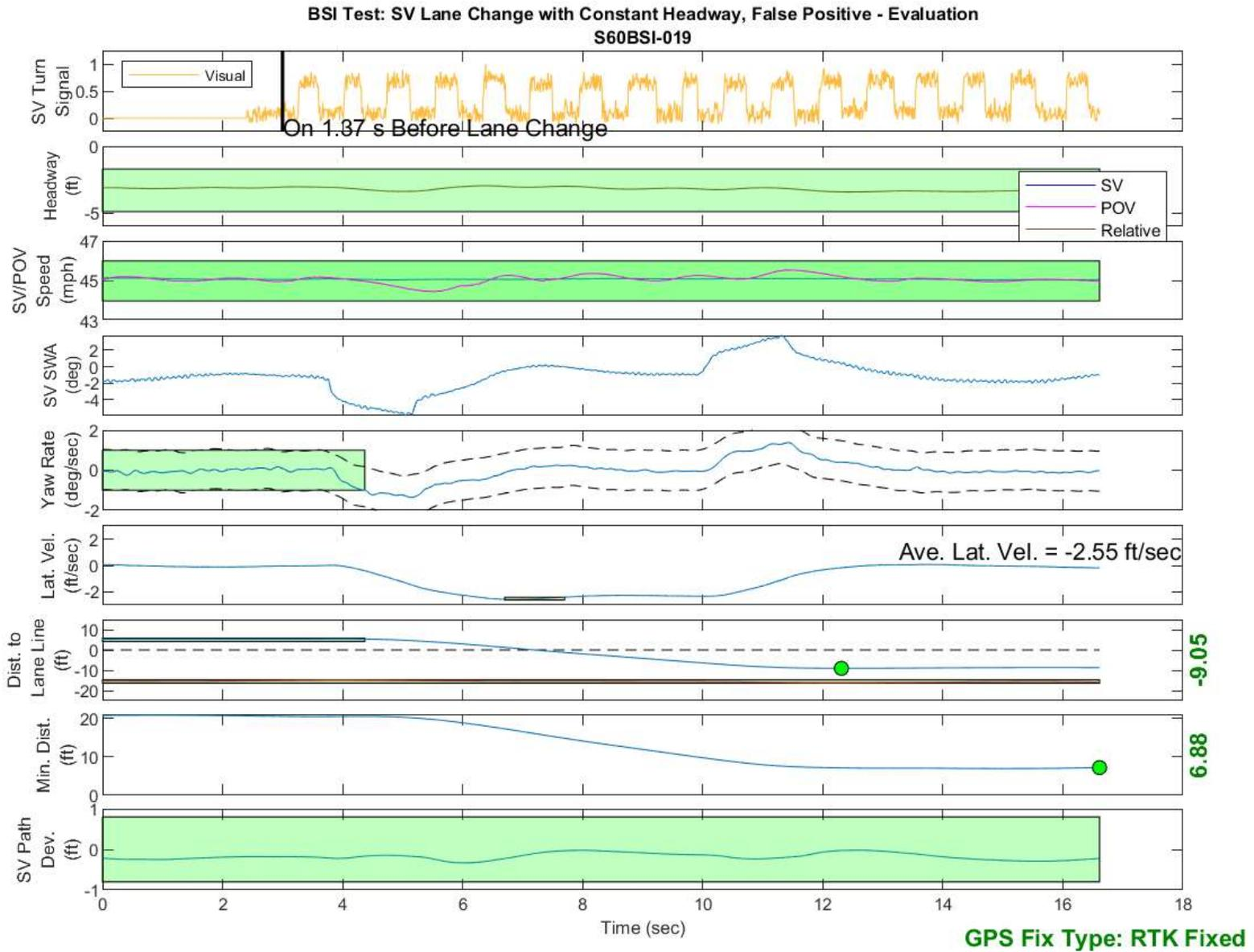
Figure D30. BSI Run 19, Subject Vehicle Lane Change with Constant Headway, False Positive Assessment - Evaluation
