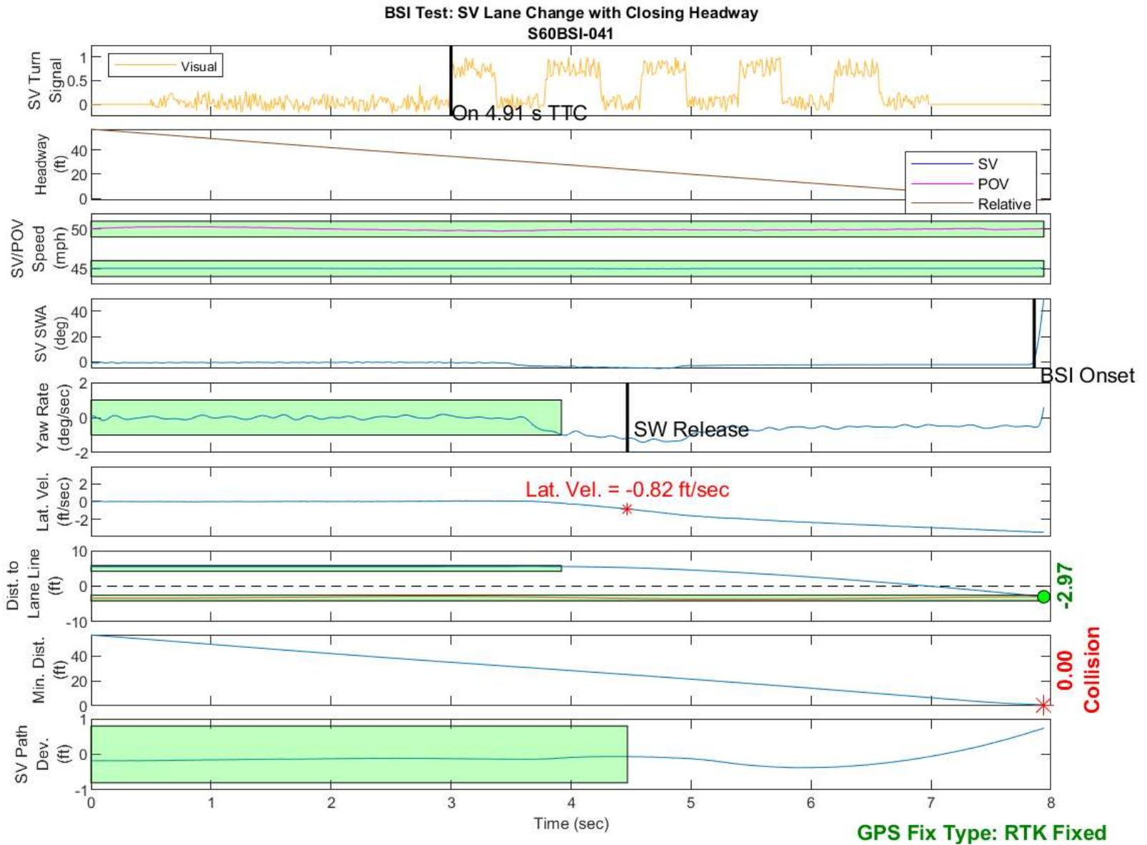
Figure D12. BSI Run 41, Subject Vehicle Lane Change with Closing Headway
