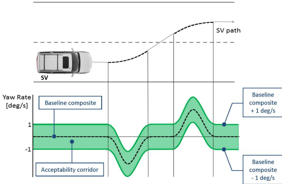
Figure 8. Definition of a Yaw Rate Acceptability Corridor
