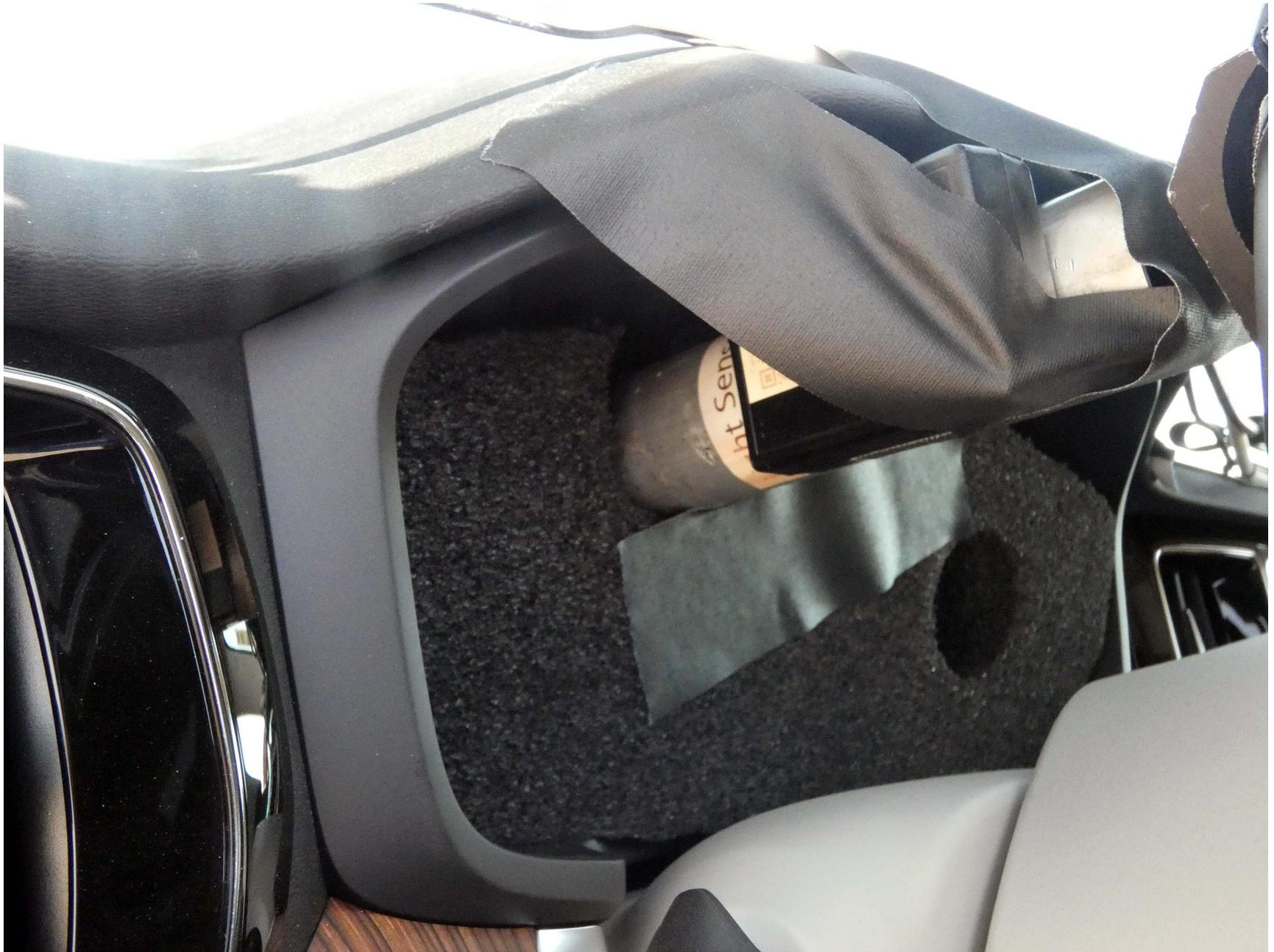
Figure A12. Sensor for Monitoring Turn Signal On/Off
