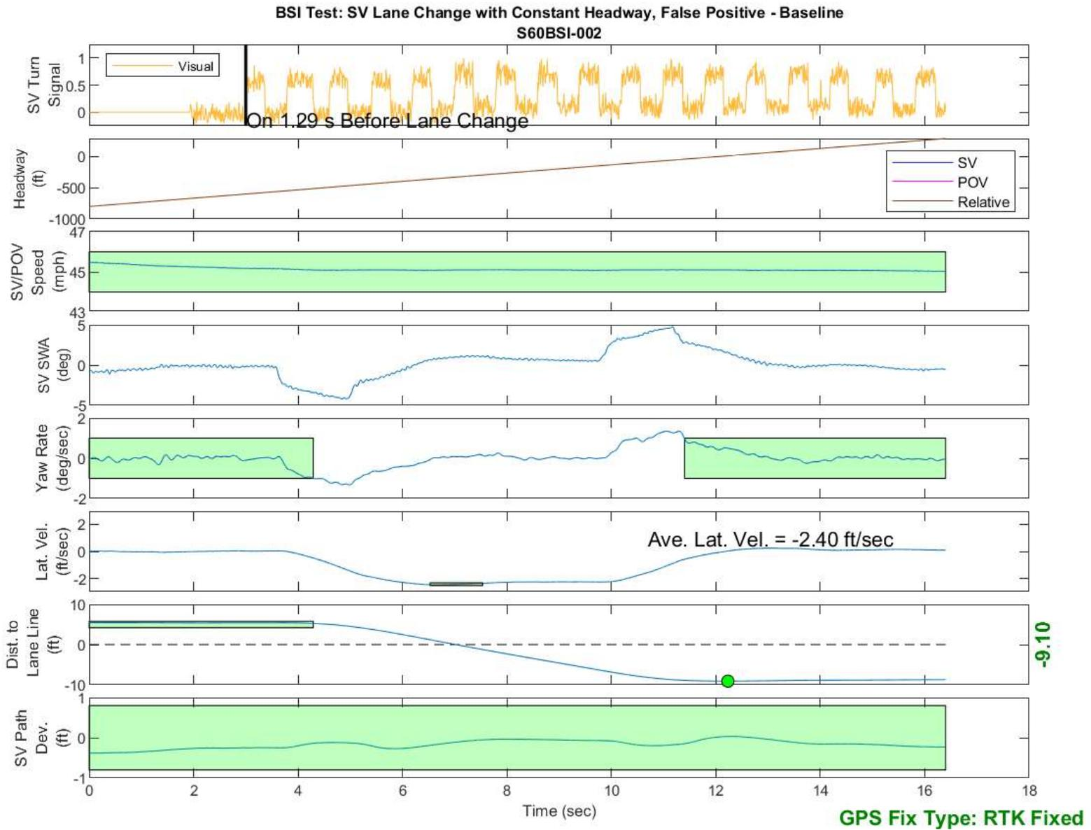
Figure D18. BSI Run 2, Subject Vehicle Lane Change with Constant Headway, False Positive Assessment - Baseline
