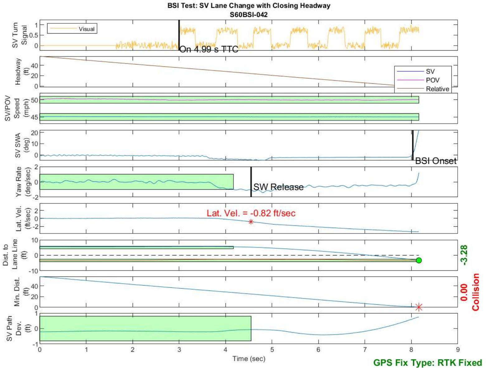
Figure D13. BSI Run 42, Subject Vehicle Lane Change with Closing Headway
