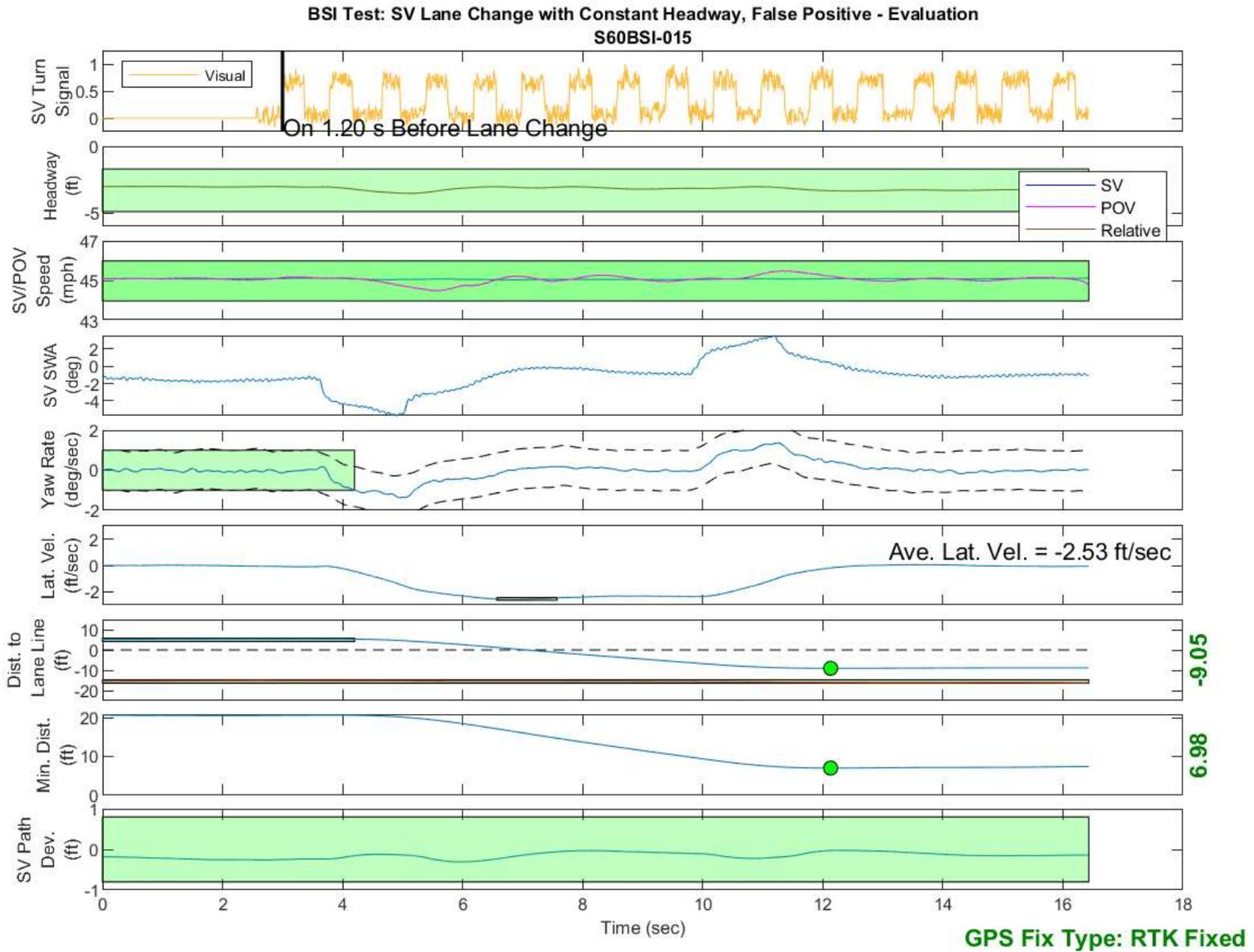
Figure D28. BSI Run 15, Subject Vehicle Lane Change with Constant Headway, False Positive Assessment - Evaluation
