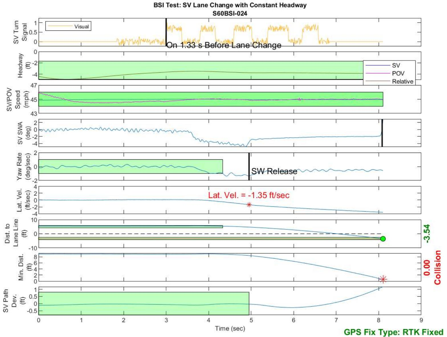
Figure D5. BSI Run 24, Subject Vehicle Lane Change with Constant Headway
