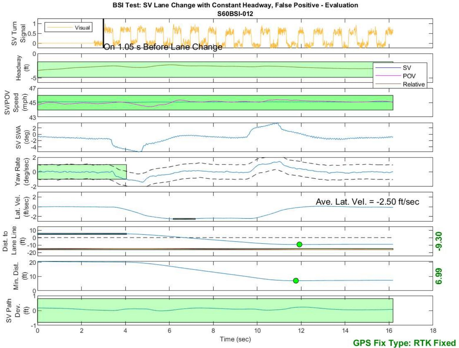
Figure D26. BSI Run 12, Subject Vehicle Lane Change with Constant Headway, False Positive Assessment - Evaluation
