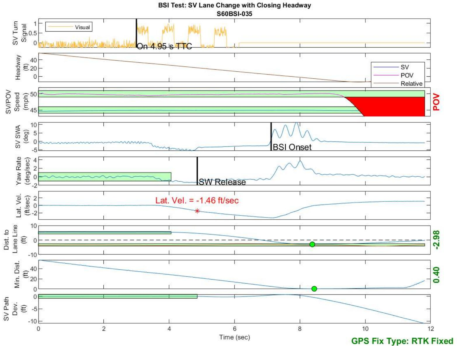
Figure D11. BSI Run 35, Subject Vehicle Lane Change with Closing Headway
