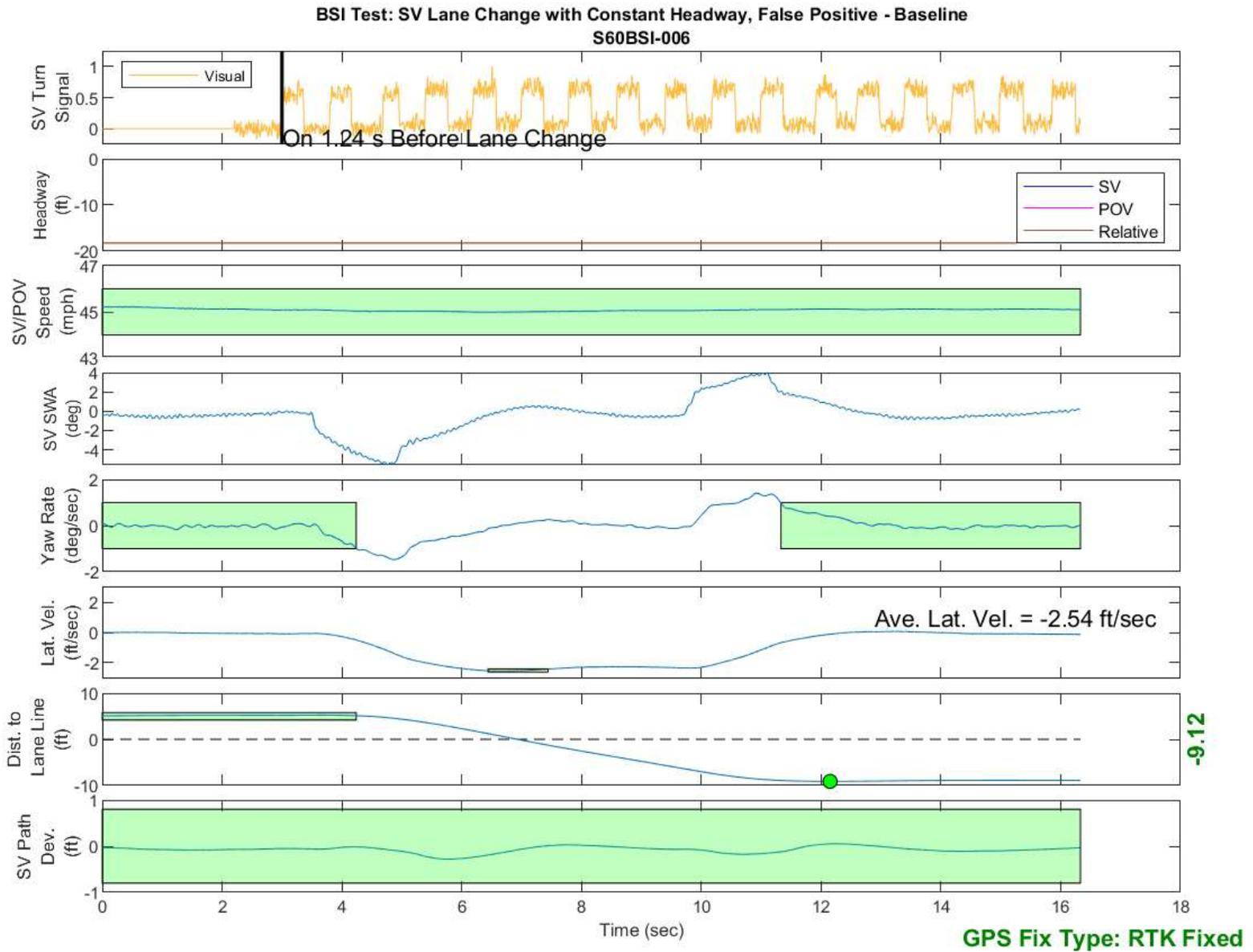
Figure D22. BSI Run 6, Subject Vehicle Lane Change with Constant Headway, False Positive Assessment - Baseline
