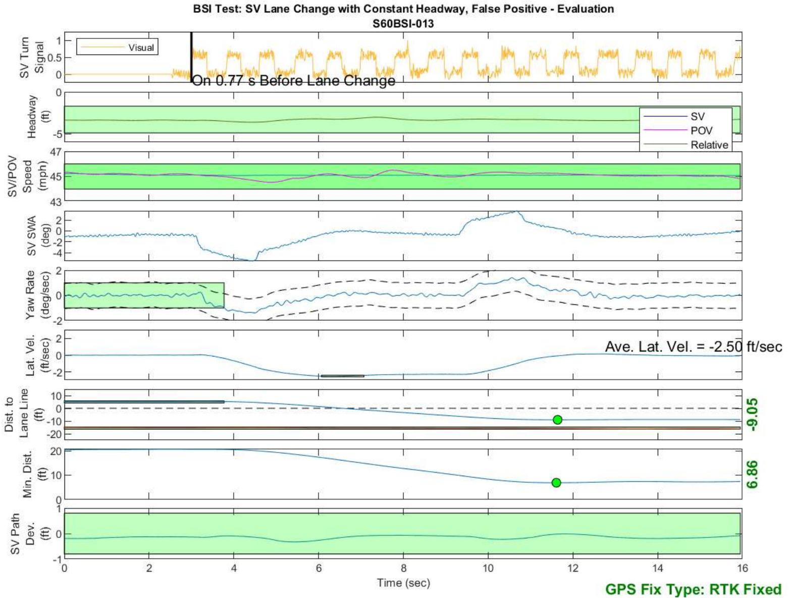
Figure D27. BSI Run 13, Subject Vehicle Lane Change with Constant Headway, False Positive Assessment - Evaluation
