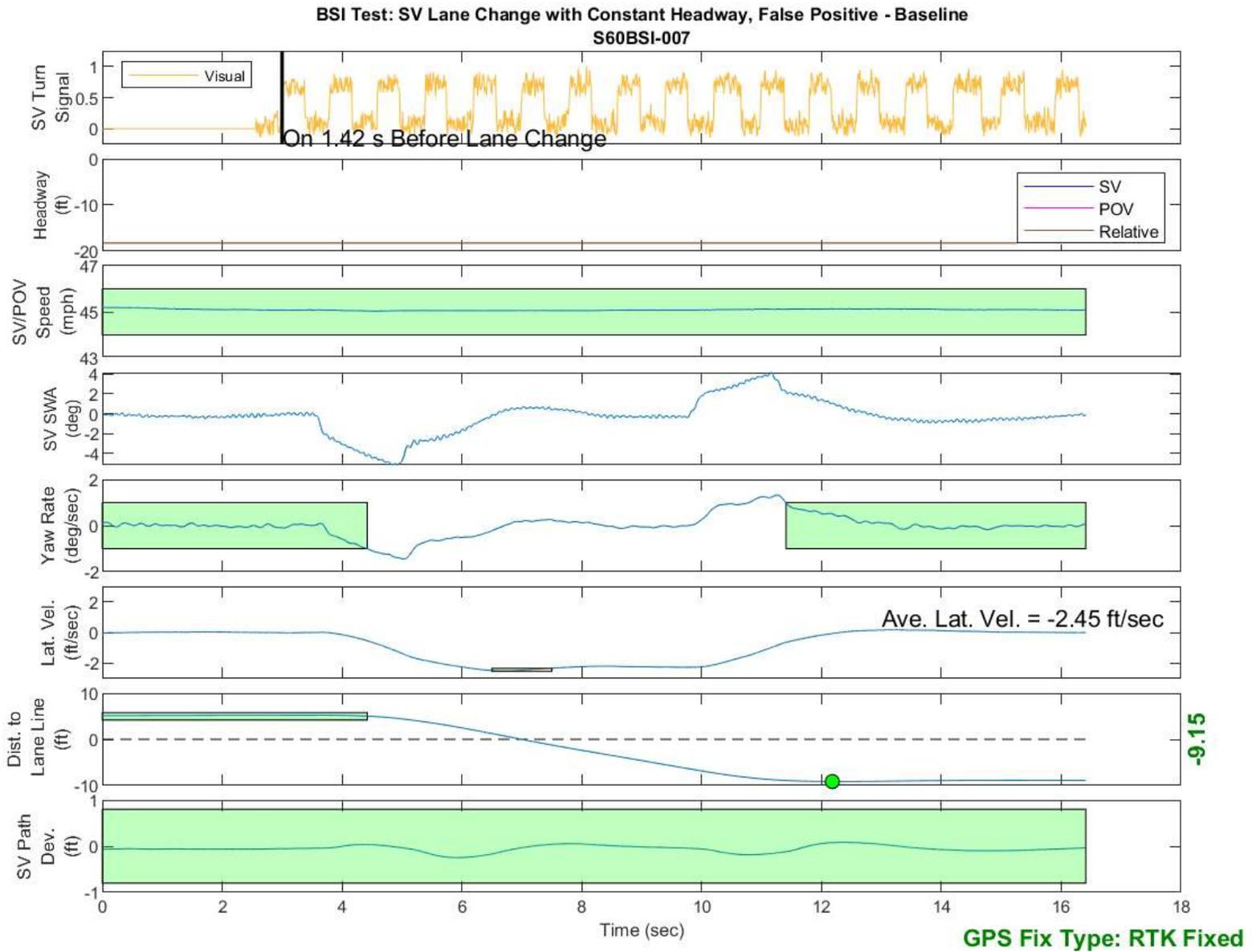
Figure D23. BSI Run 7, Subject Vehicle Lane Change with Constant Headway, False Positive Assessment - Baseline
