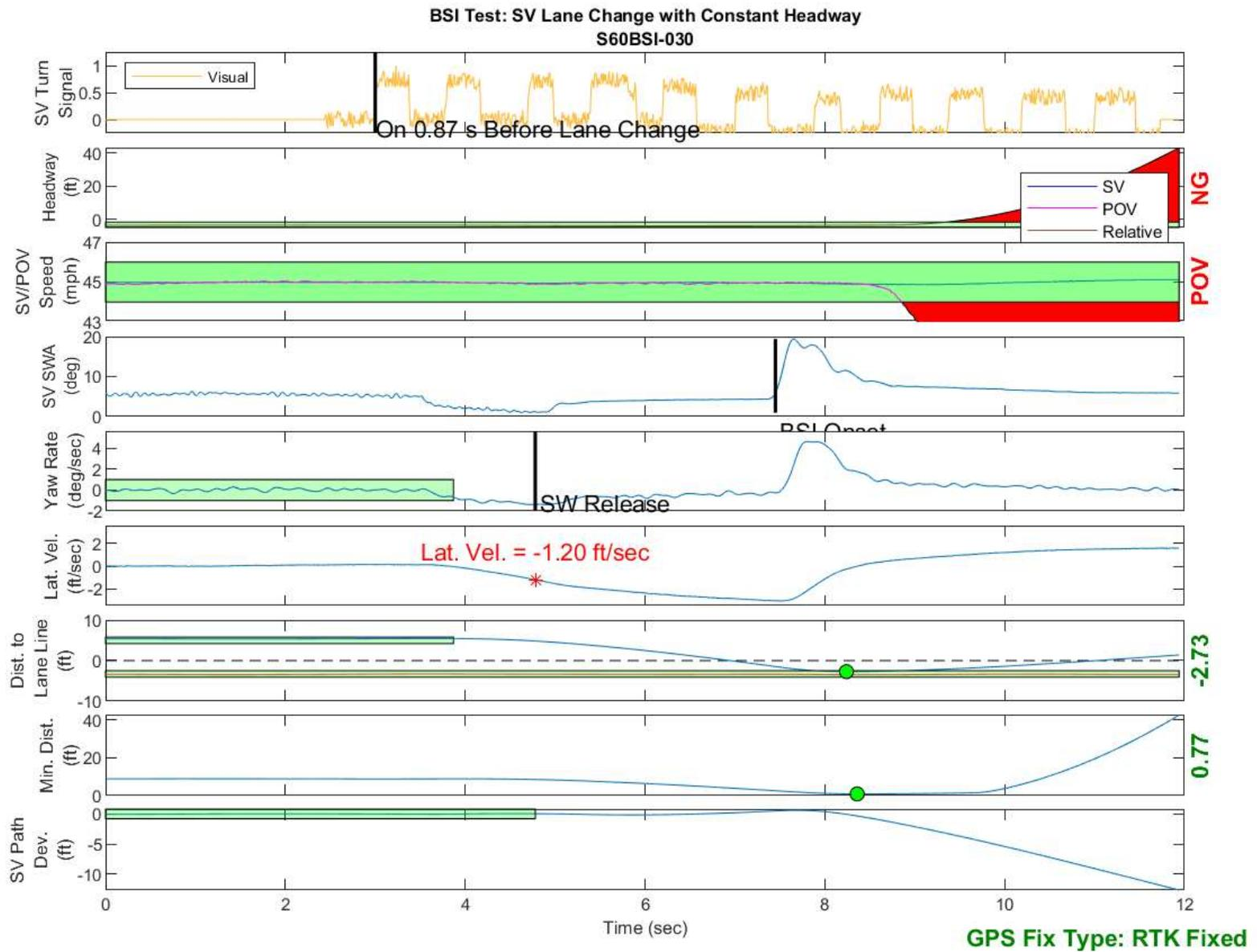
Figure D10. BSI Run 30, Subject Vehicle Lane Change with Constant Headway
