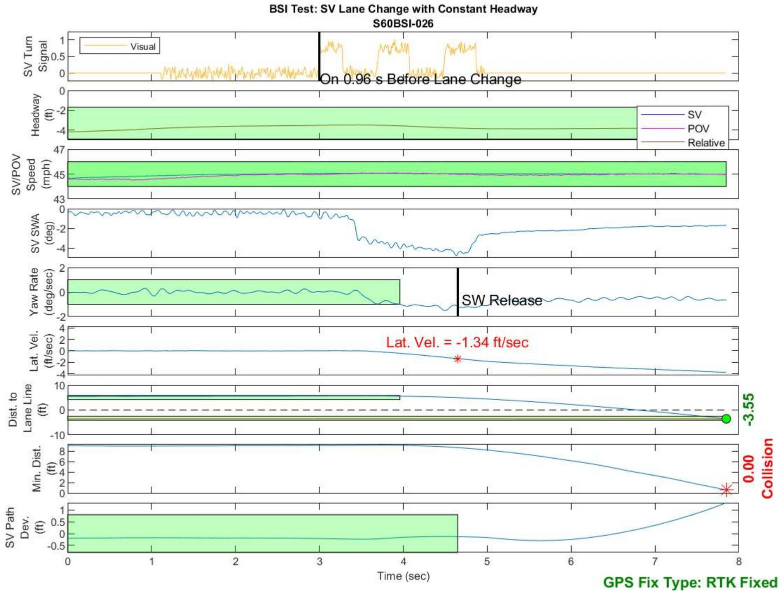
Figure D7. BSI Run 26, Subject Vehicle Lane Change with Constant Headway
