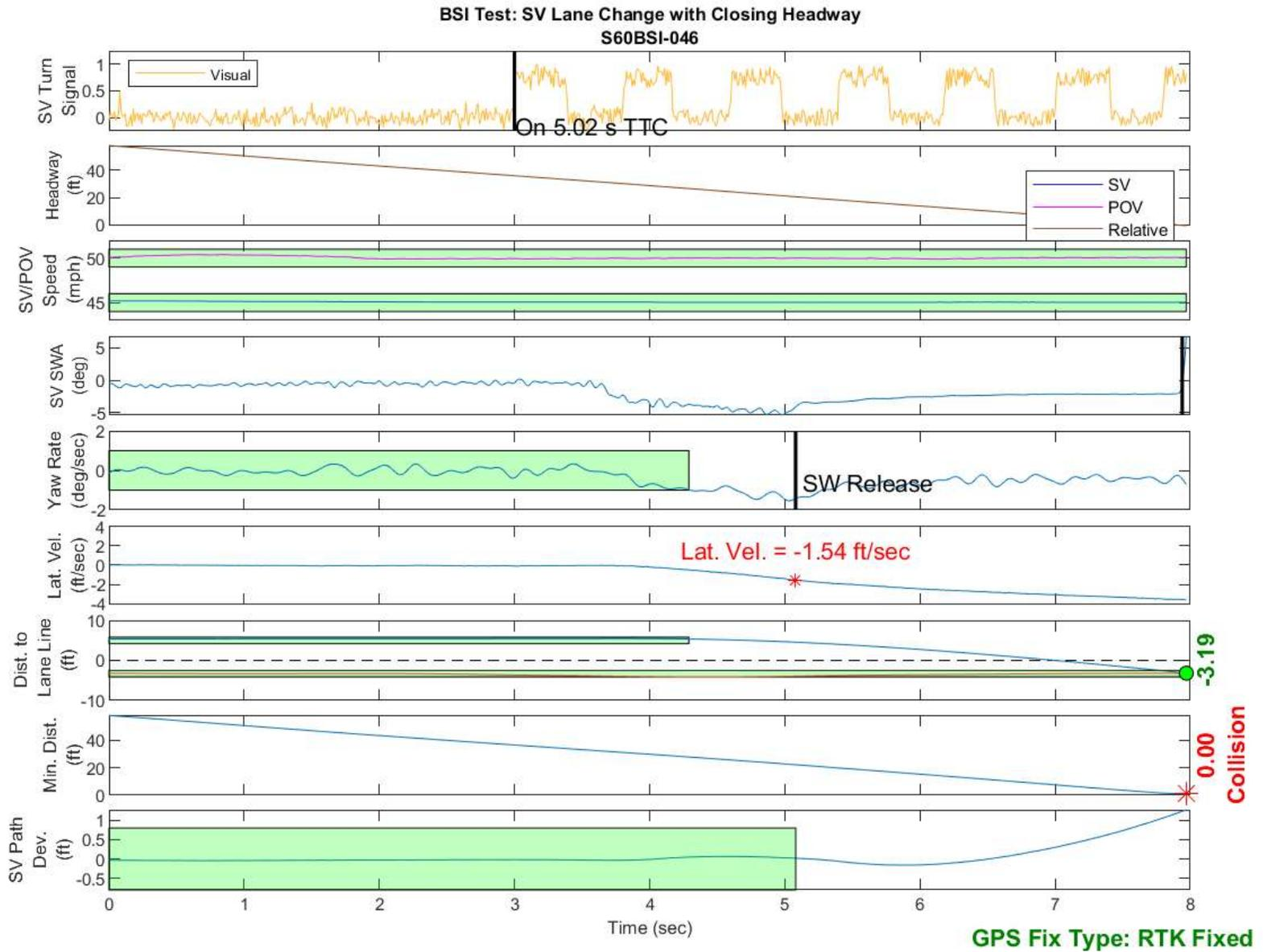
Figure D16. BSI Run 46, Subject Vehicle Lane Change with Closing Headway
