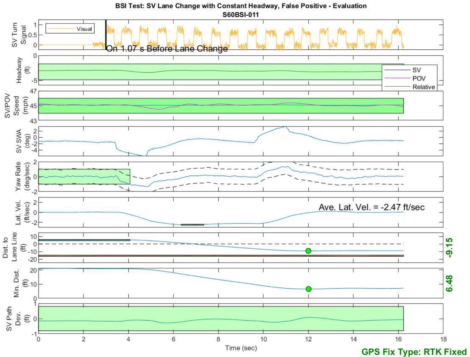
Figure D25. BSI Run 11, Subject Vehicle Lane Change with Constant Headway, False Positive Assessment - Evaluation
