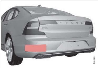
Keep the marked area clean (on both the left and right sides of the vehicle)<sup>68</sup>.
