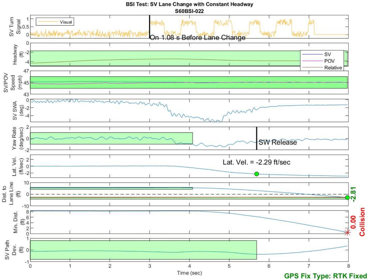
Figure D4. BSI Run 22, Subject Vehicle Lane Change with Constant Headway
