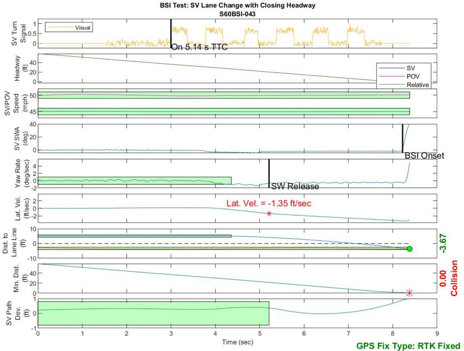
Figure D14. BSI Run 43, Subject Vehicle Lane Change with Closing Headway
