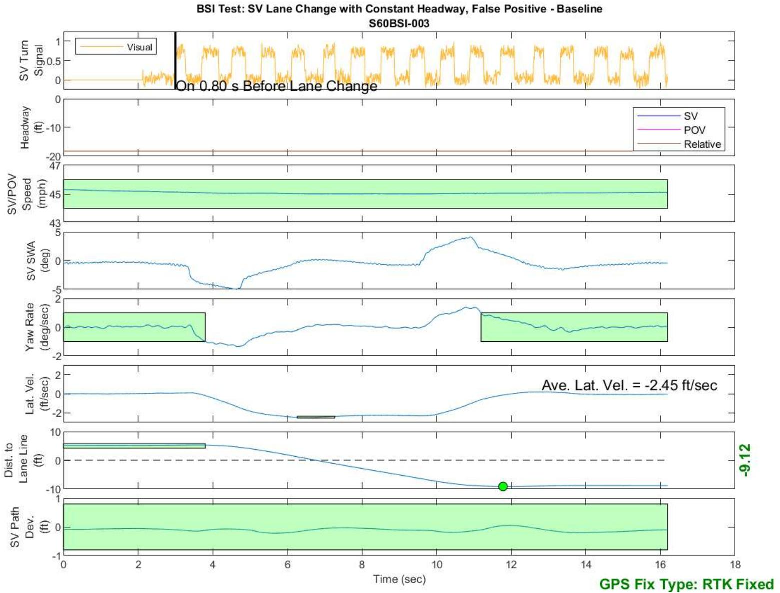
Figure D19. BSI Run 3, Subject Vehicle Lane Change with Constant Headway, False Positive Assessment - Baseline
