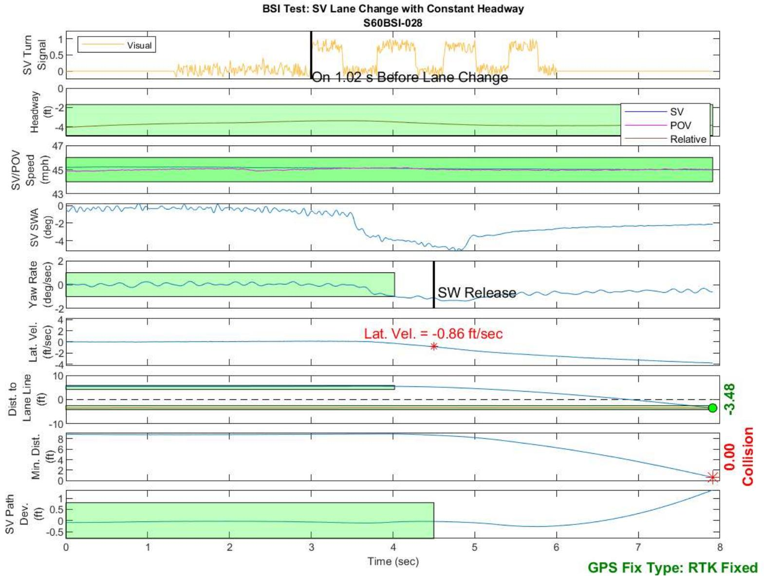
Figure D9. BSI Run 28, Subject Vehicle Lane Change with Constant Headway
