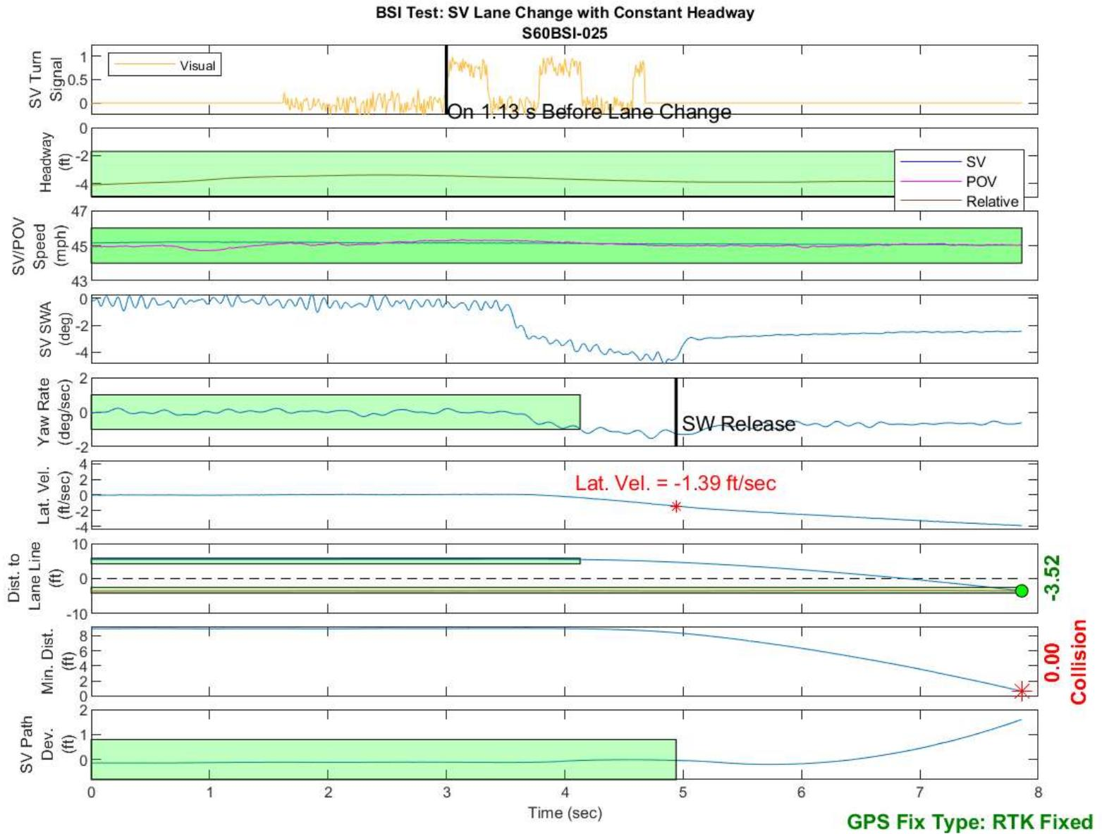
Figure D6. BSI Run 25, Subject Vehicle Lane Change with Constant Headway
