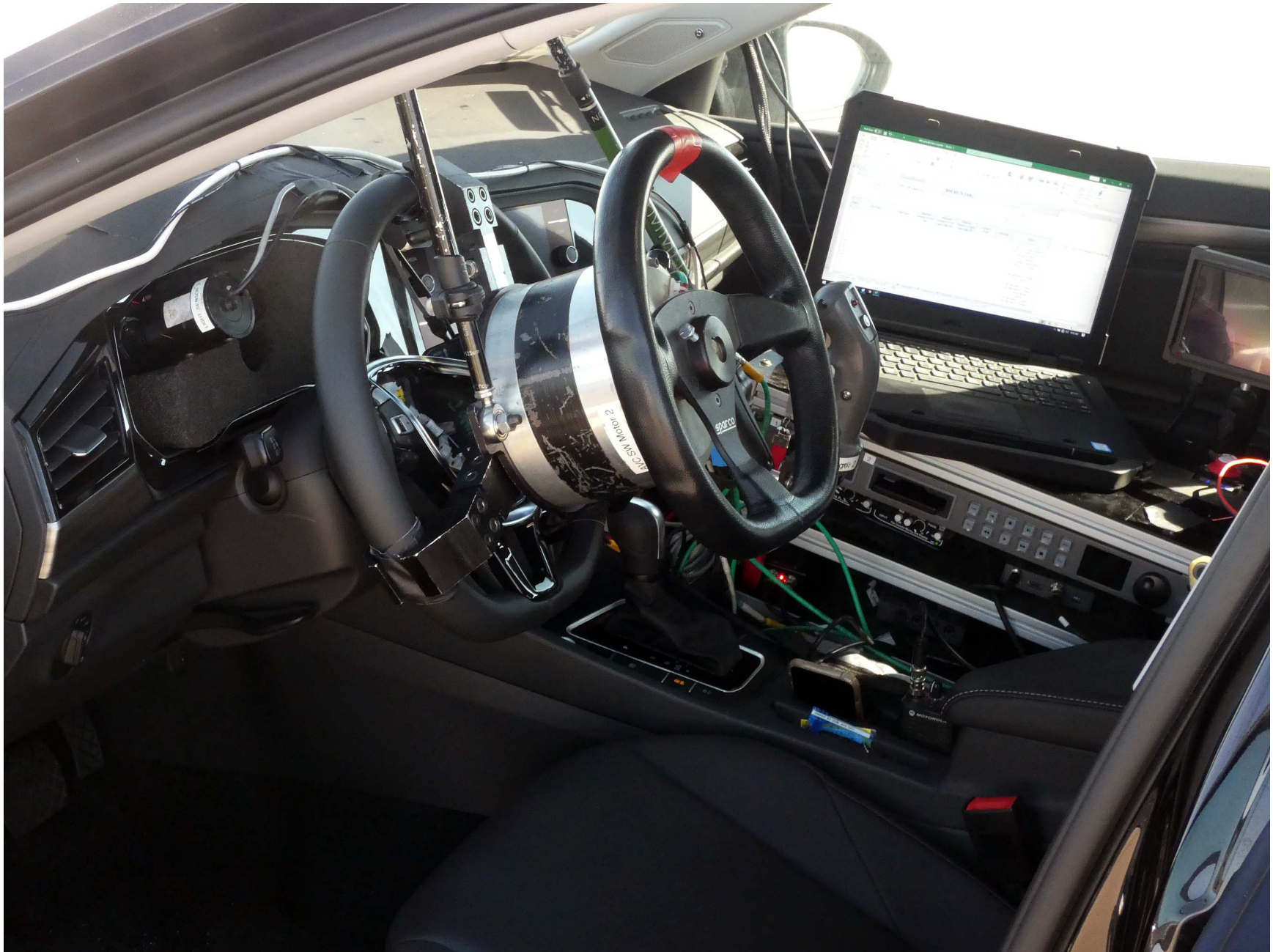
Figure A10. Computer and Steering Controller Installed in Subject Vehicle
