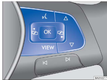
Fig. 17 Right side of the multi-function steering wheel: buttons for operating the menus and information displays in the instrument cluster
