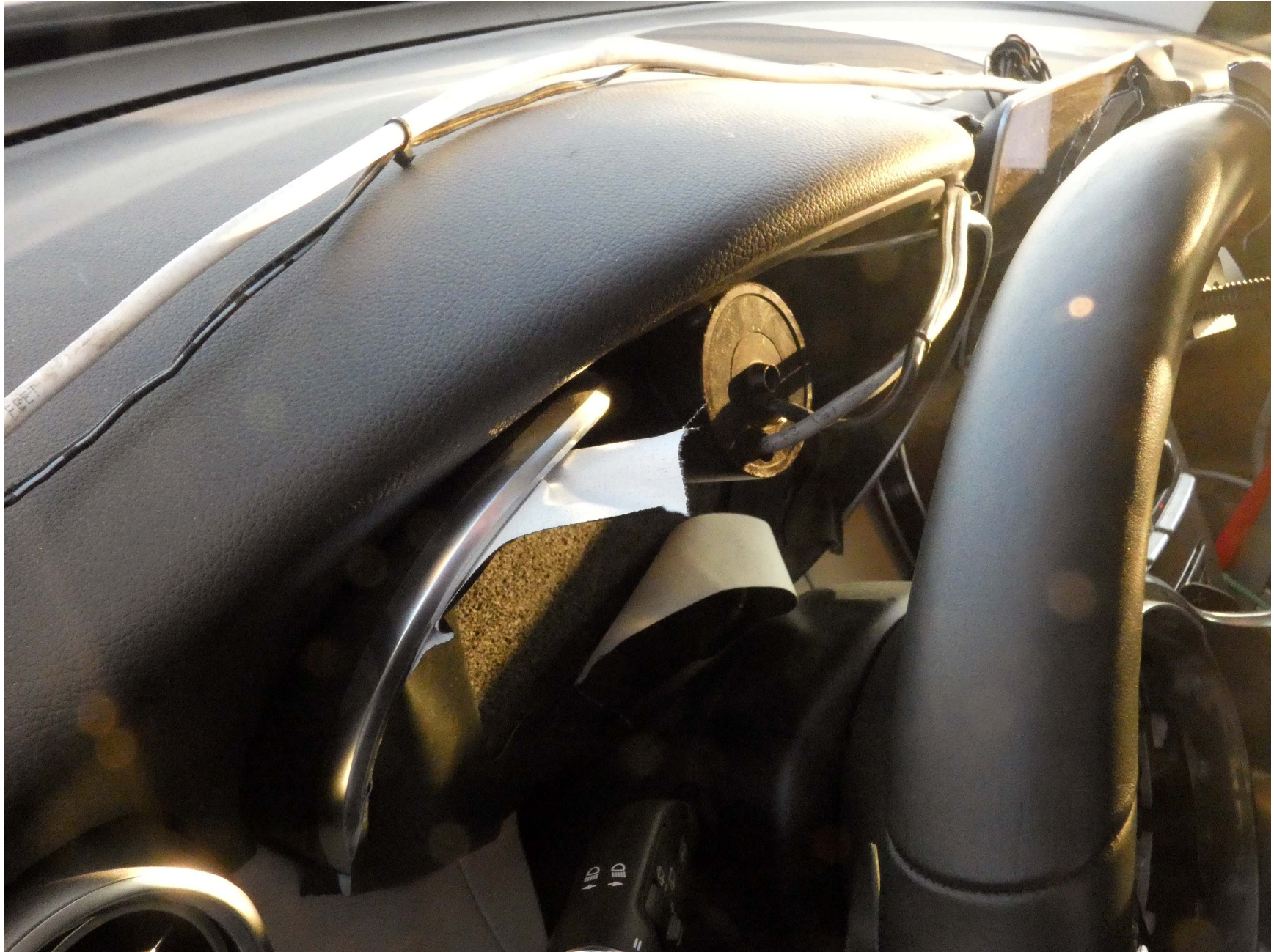
Figure A10. Sensor for Detecting Visual Alerts
