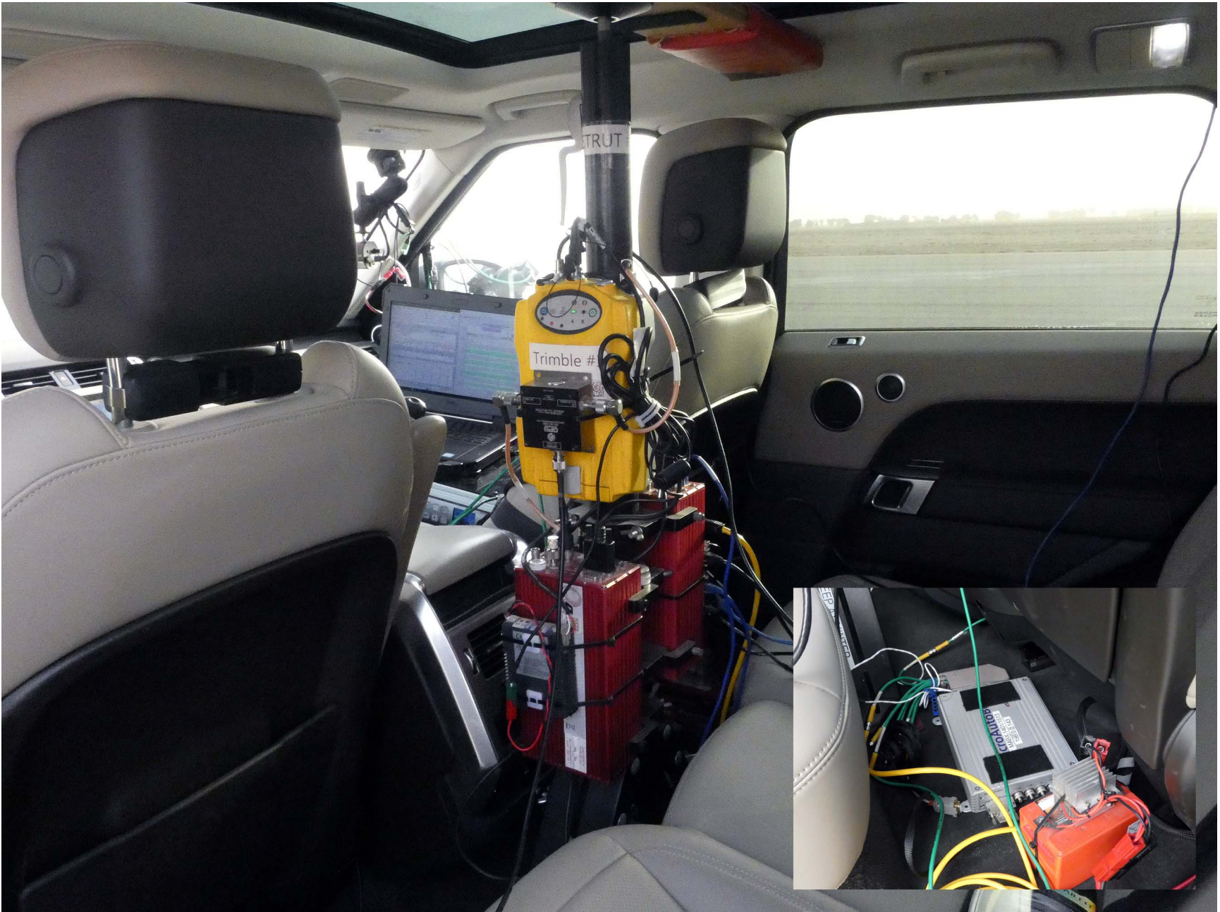
Figure A11. DGPS, Inertial Measurement Unit, and MicroAutoBox Installed in Subject Vehicle
