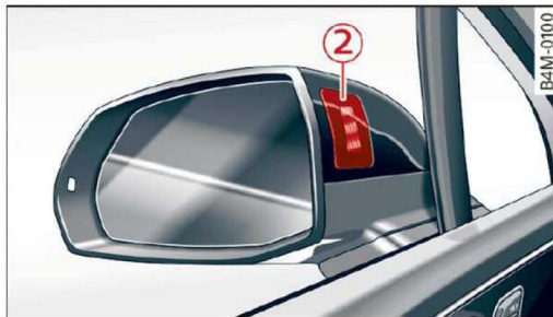
Fig. 129 Indicator on the exterior mirror
