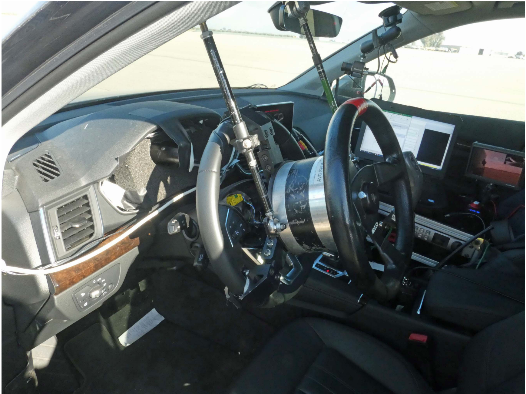
Figure A12. Computer and Steering Controller Installed in Subject Vehicle
