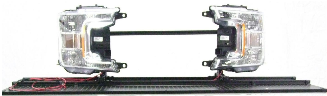
Figure 10. NHTSA-Specified Stimulus Lamps, Oncoming F-150 Truck Headlamps
