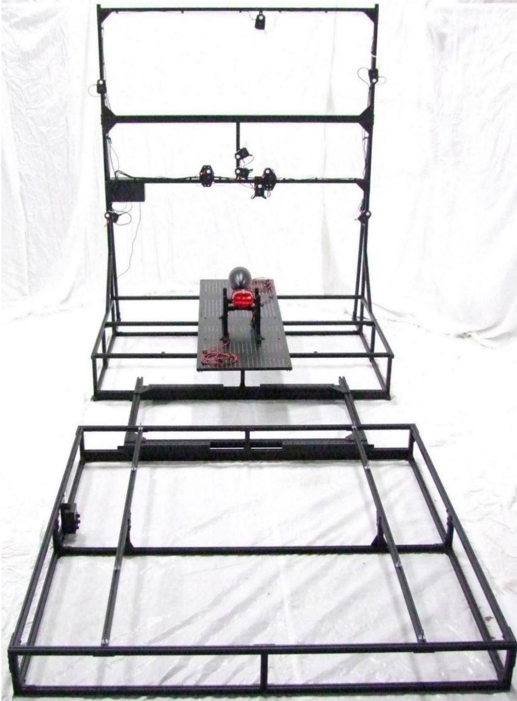
Figure 19. NHTSA Test Fixture Photo, Harley Davidson Motorcycle Taillamp Stimulus Lamp
