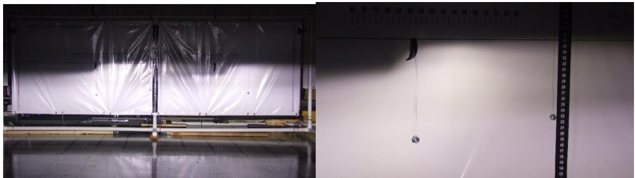
Figure 101. Volvo XC90 Headlamp Adjustment, Set to 36 Inches
