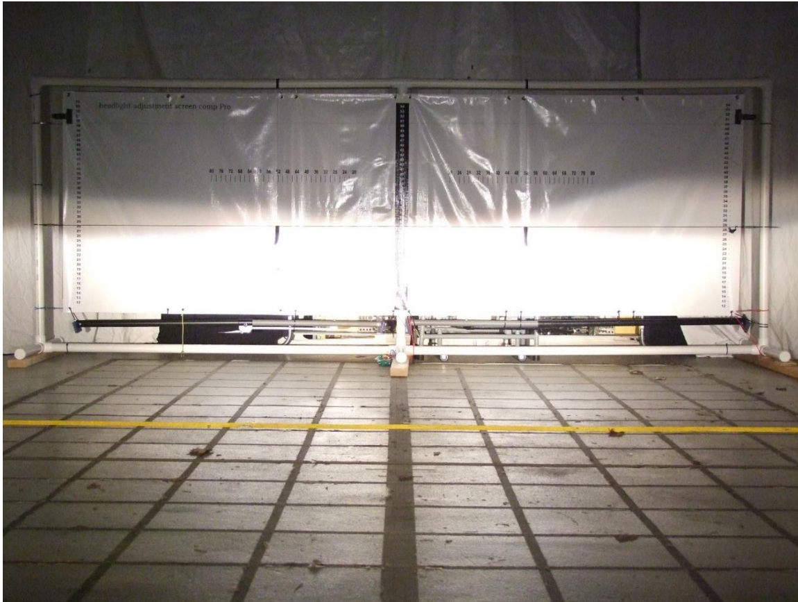
Figure 87. Ford Fusion Headlamp Adjustment (Adjusted_Fusion_Both_Lights.jpg)
