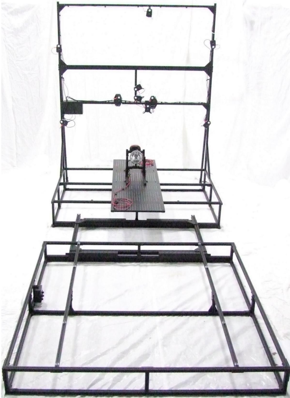
Figure 18. NHTSA Test Fixture Photo, Harley Davidson Motorcycle Headlamp Stimulus Lamp
