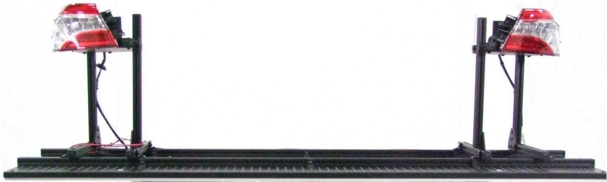
Figure 9. NHTSA-Specified Stimulus Lamps, Same Direction Camry Taillamps
