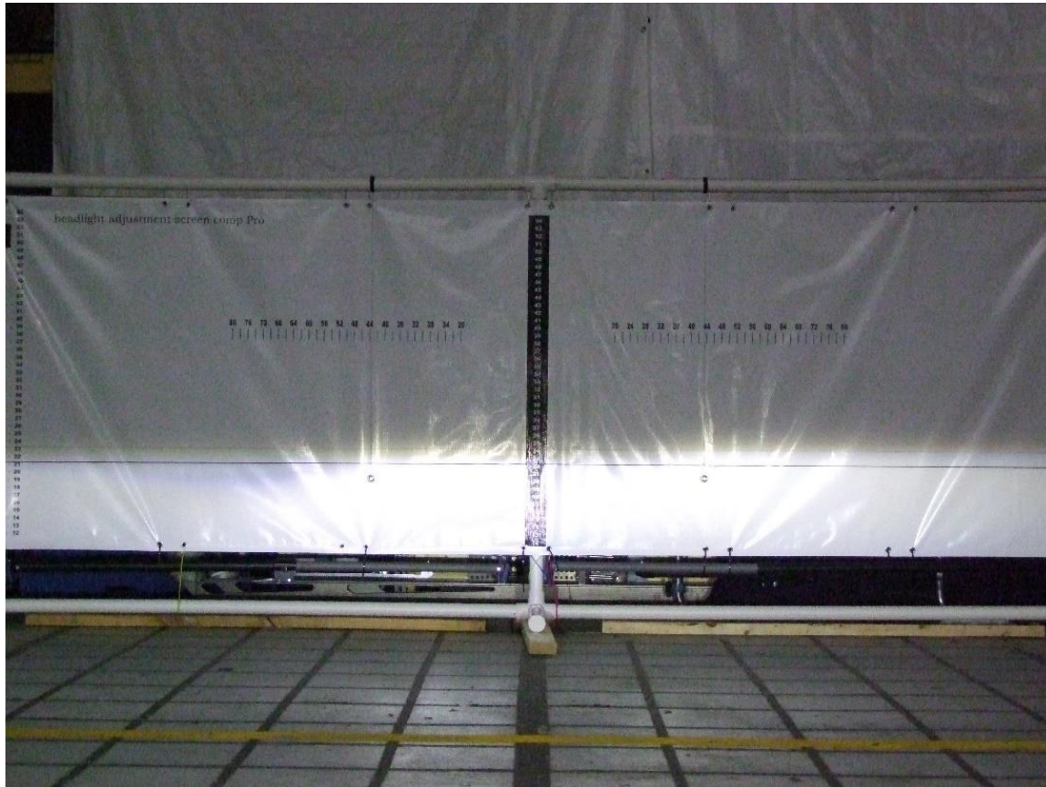
Figure 89. NHTSA Stimulus Camry Headlamp Adjustment (Adjusted_Camry_Headlights2.jpg)
