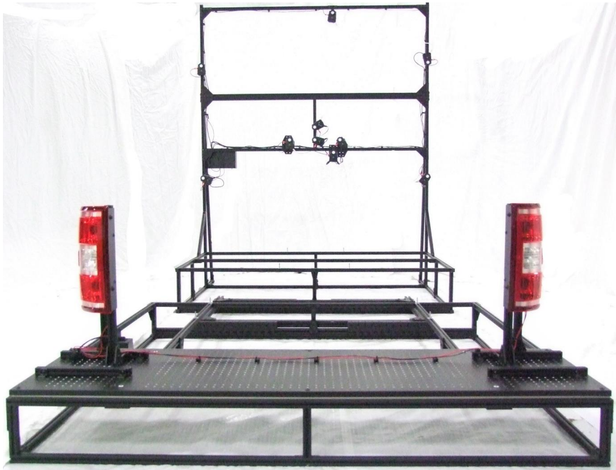
Figure 17. NHTSA Test Fixture Photo, F-150 Truck Taillamp Stimulus Lamps
