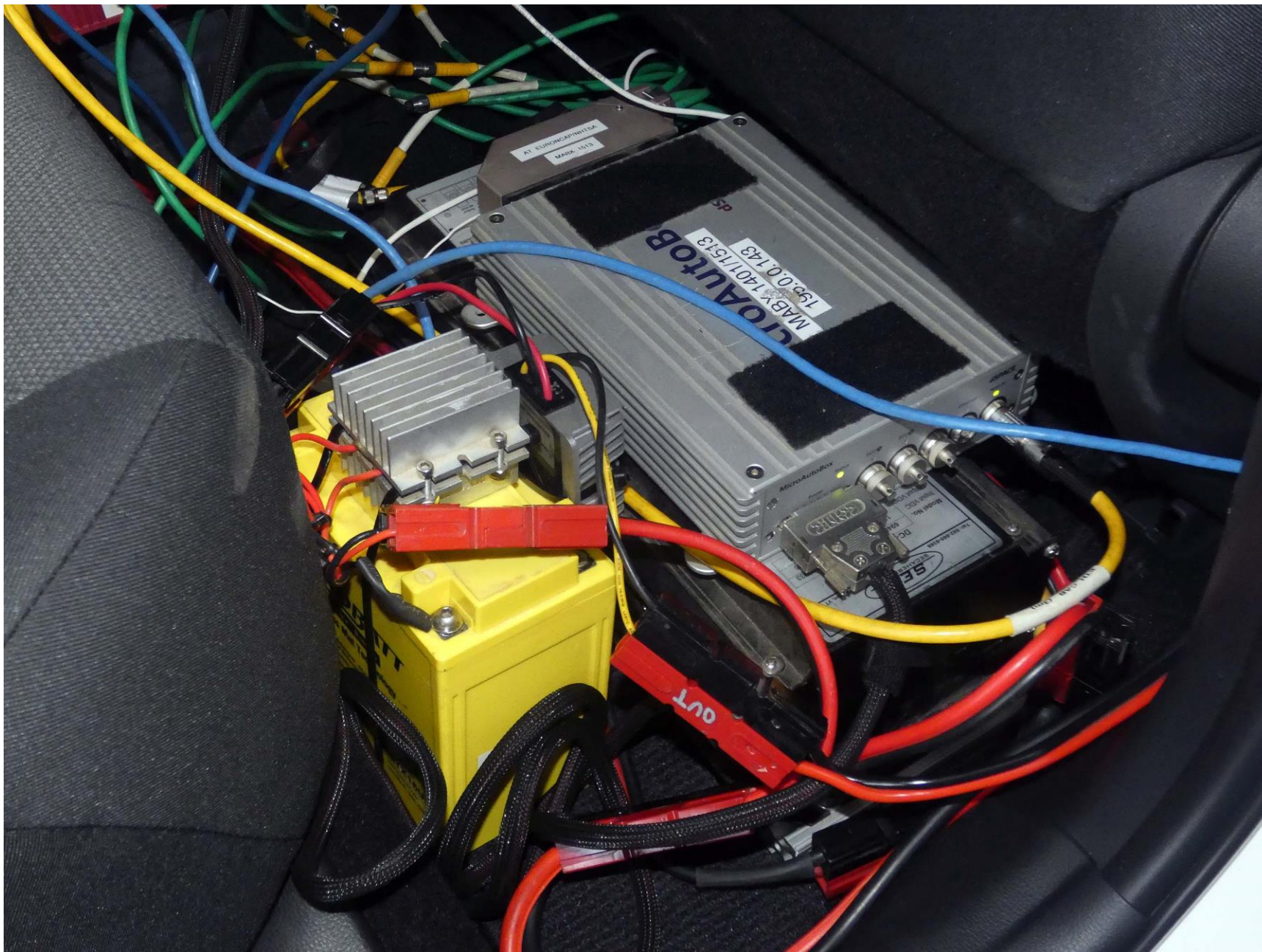
Figure A6. MicroAutoBox Installed in Subject Vehicle
