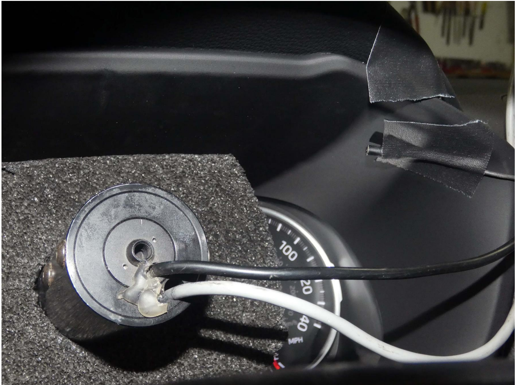
Figure A9. Sensors for Detecting Auditory and Visual Alerts
