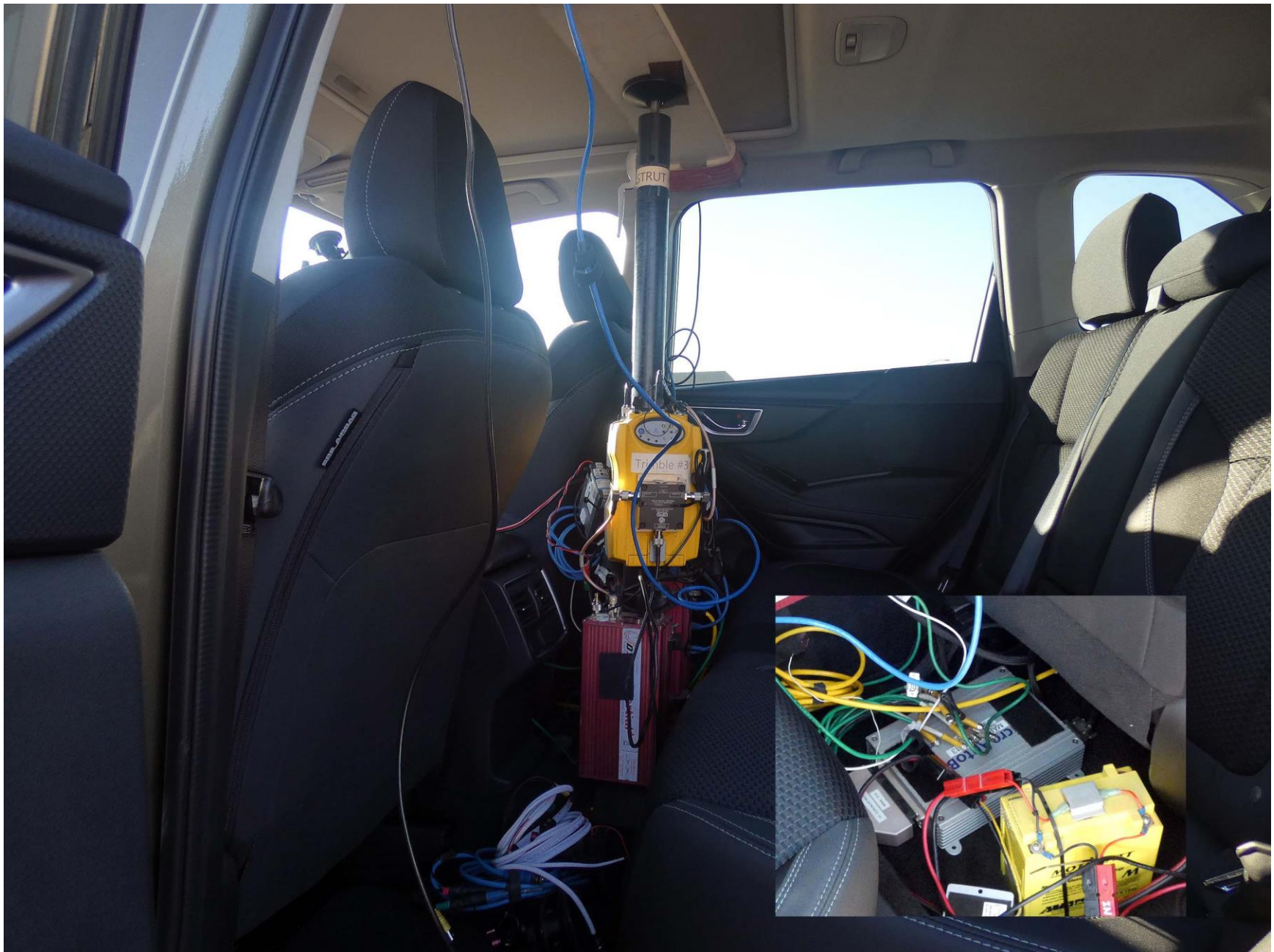
Figure A6. DGPS, Inertial Measurement Unit, and MicroAutoBox Installed in Subject Vehicle
