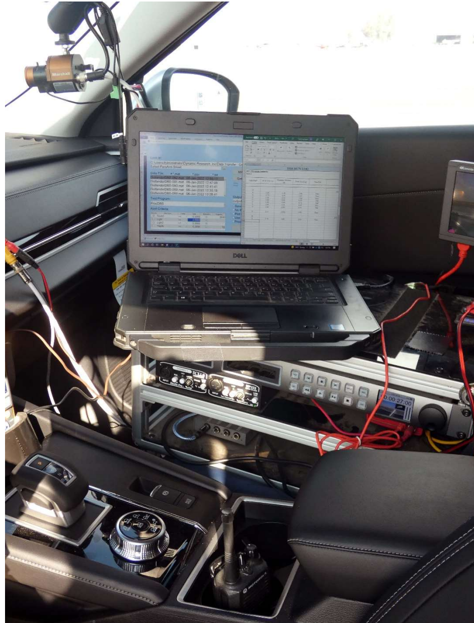
Figure A8. Computer Installed in Subject Vehicle
