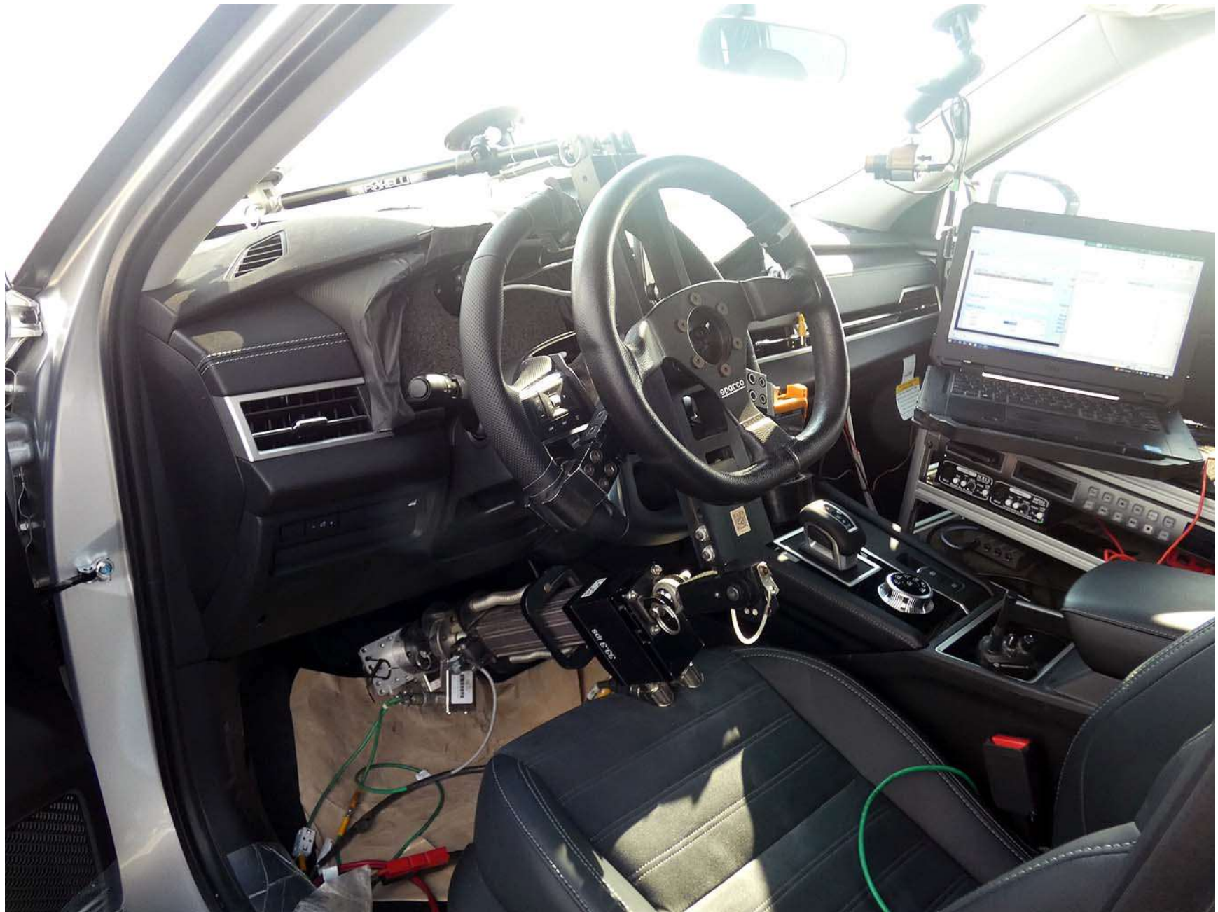
Figure A12. Computer Installed in Subject Vehicle
