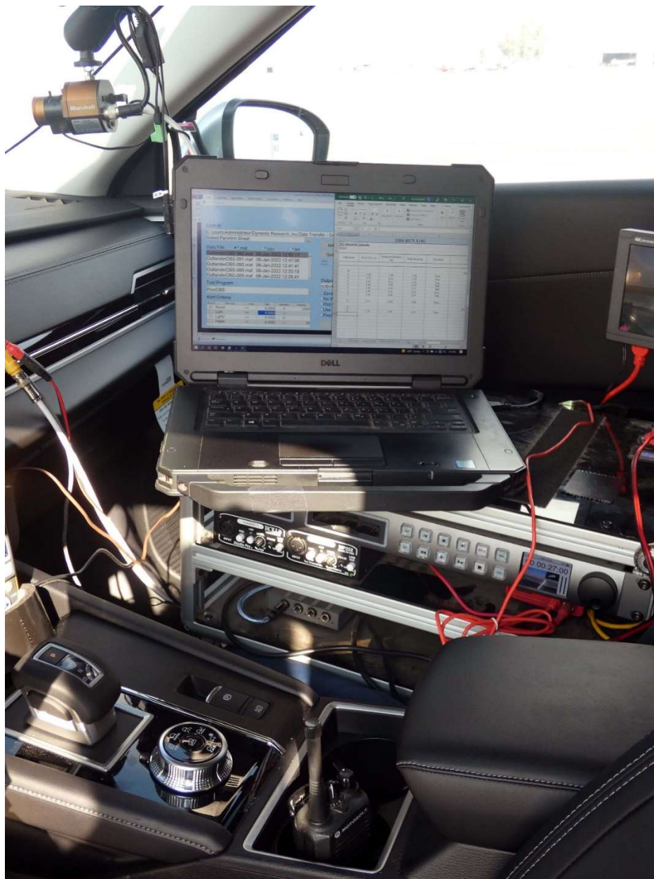
Figure A10. Computer Installed in Subject Vehicle
