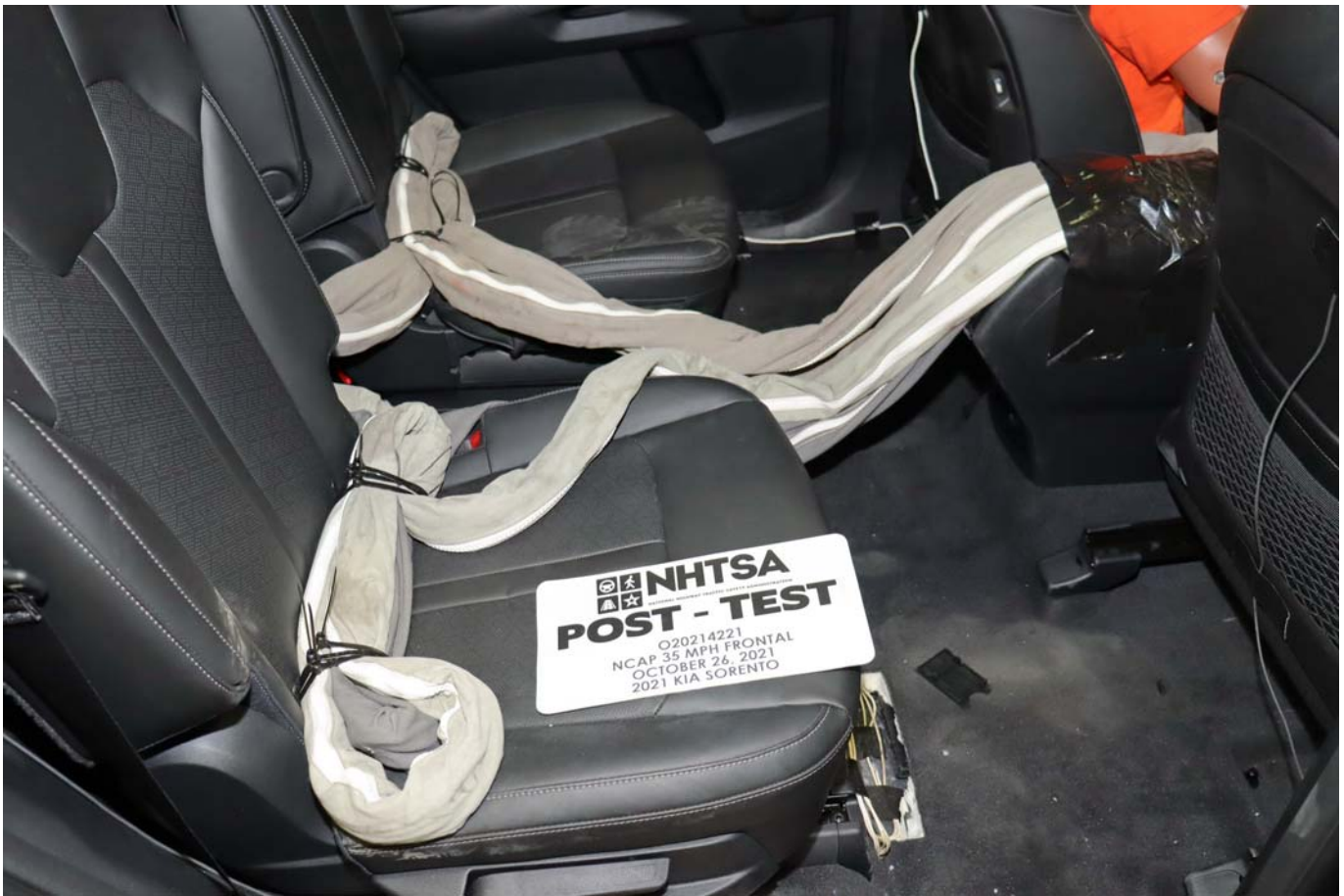
Photo No. 029 - Post-Test Dummy Cable Routing
