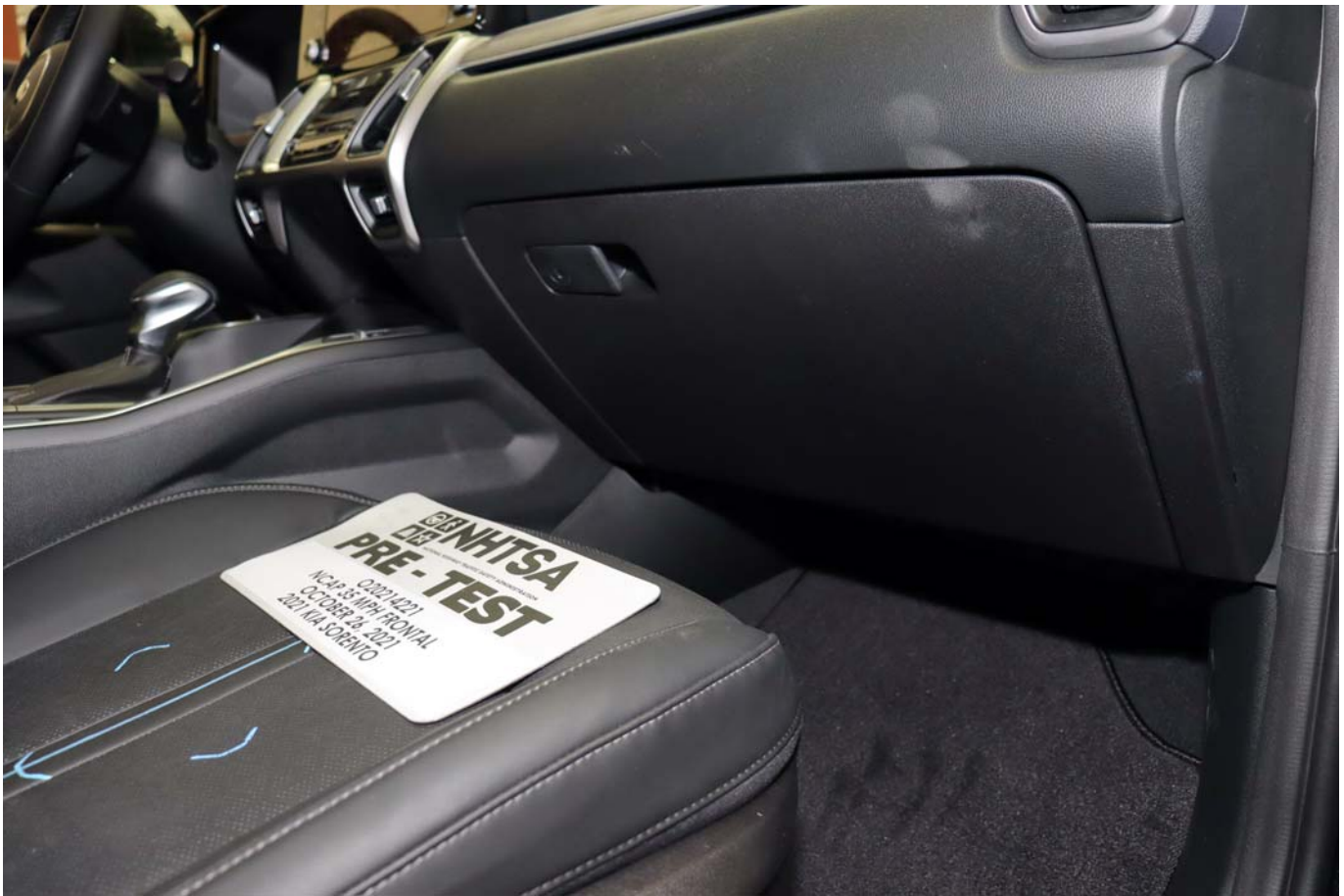
Photo No. 067 - Pre-Test Passenger Side Knee Bolster
