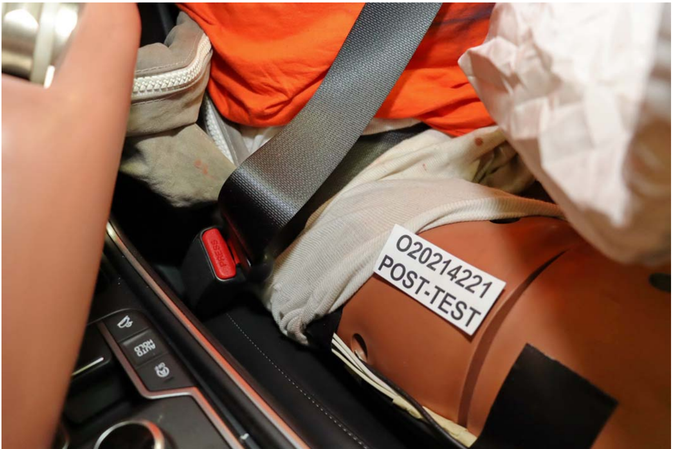
Photo No. 041 - Post-Test View of Belt Buckle and Latch Plate for Driver Dummy
