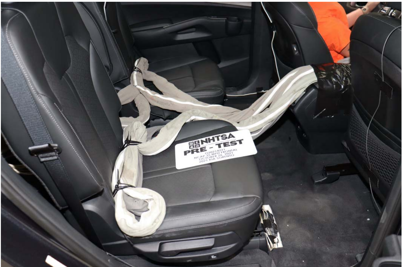
Photo No. 028 - Pre-Test Dummy Cable Routing
