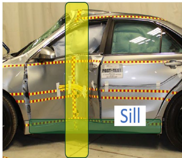
Main Load Paths during FMVSS No 214 (a) Pole; (b) MDB; and (c) Static Door Crush
