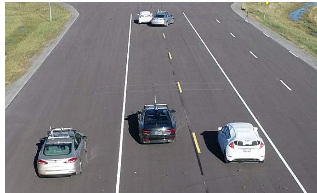
Figure 24. TJA Suddenly Revealed Stopped Vehicle (SRSV) Test Procedure Scenario
