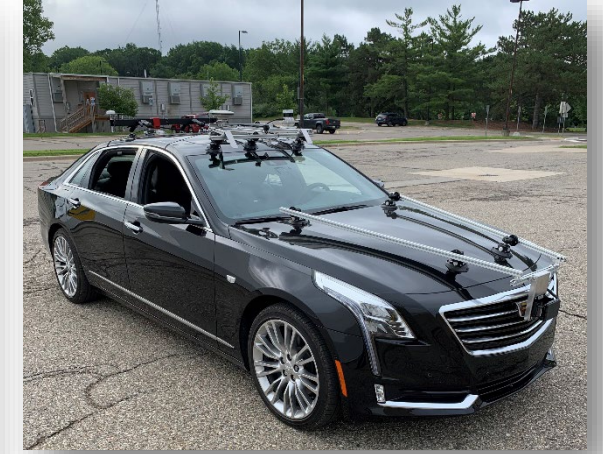
On-road Ground Truth Trip Recorder
