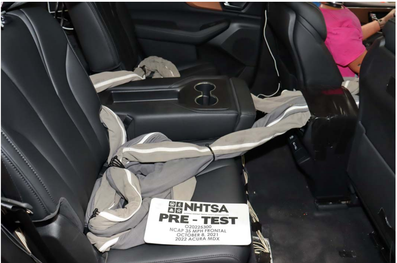
Photo No. 028 - Pre-Test Dummy Cable Routing
