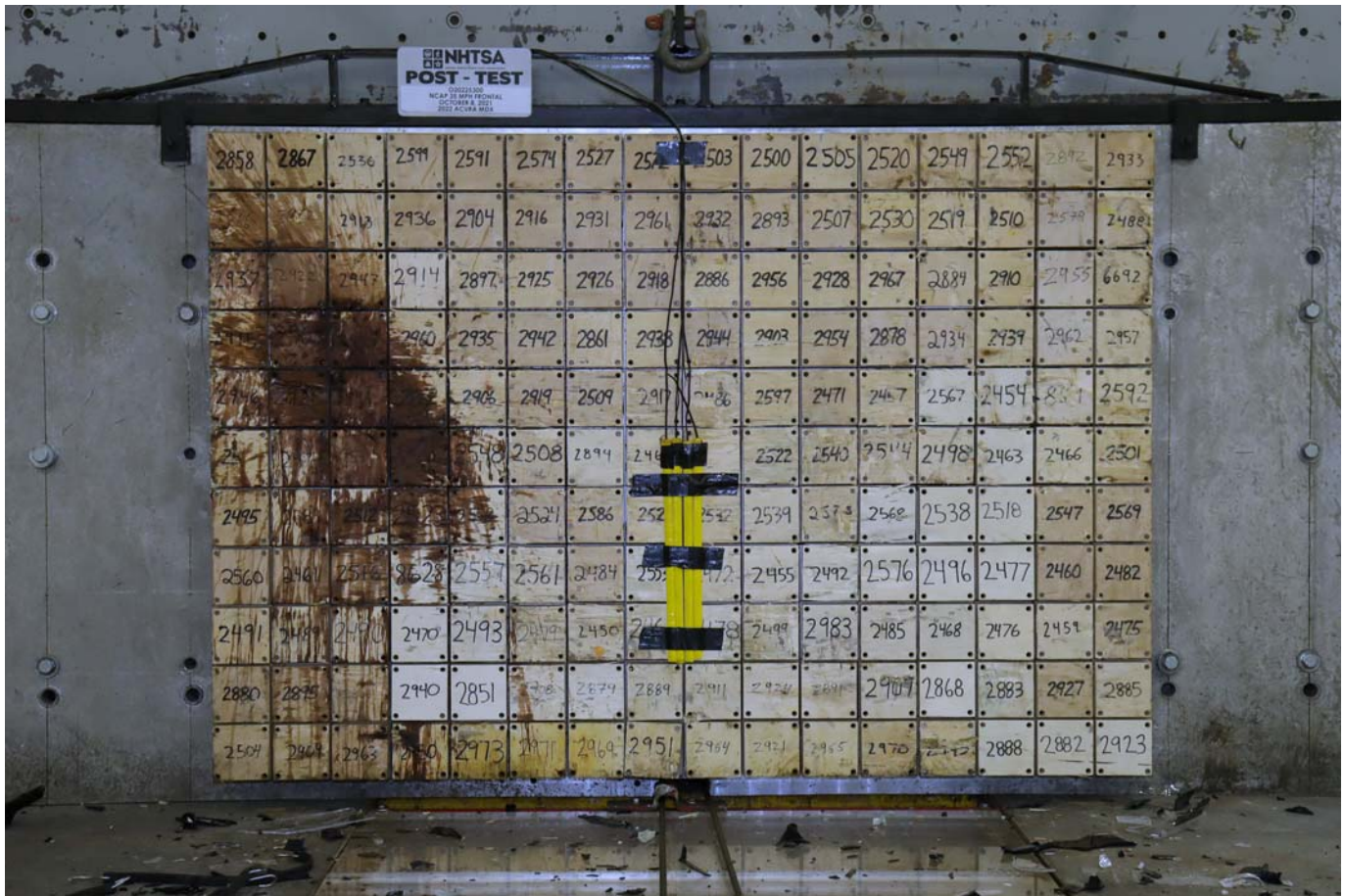
Photo No. 003 - Post-Test Load Cell Wall
