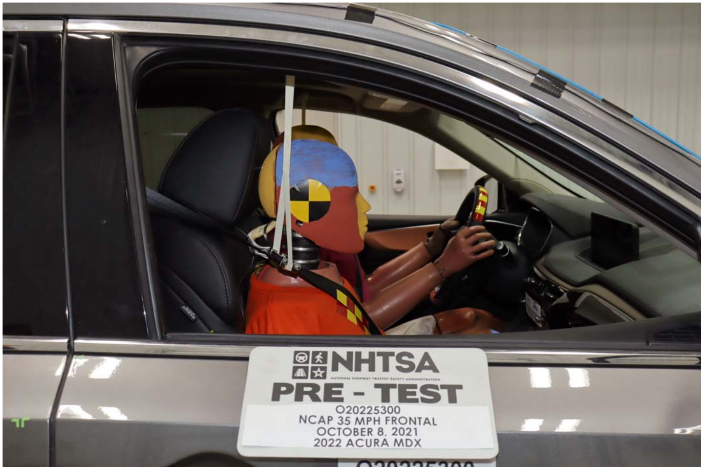
Photo No. 055 - Pre-Test Passenger Dummy Window View
