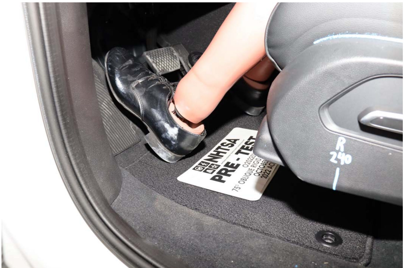
Photo No. 032 - Pre-Test Placement of Dummy Feet
