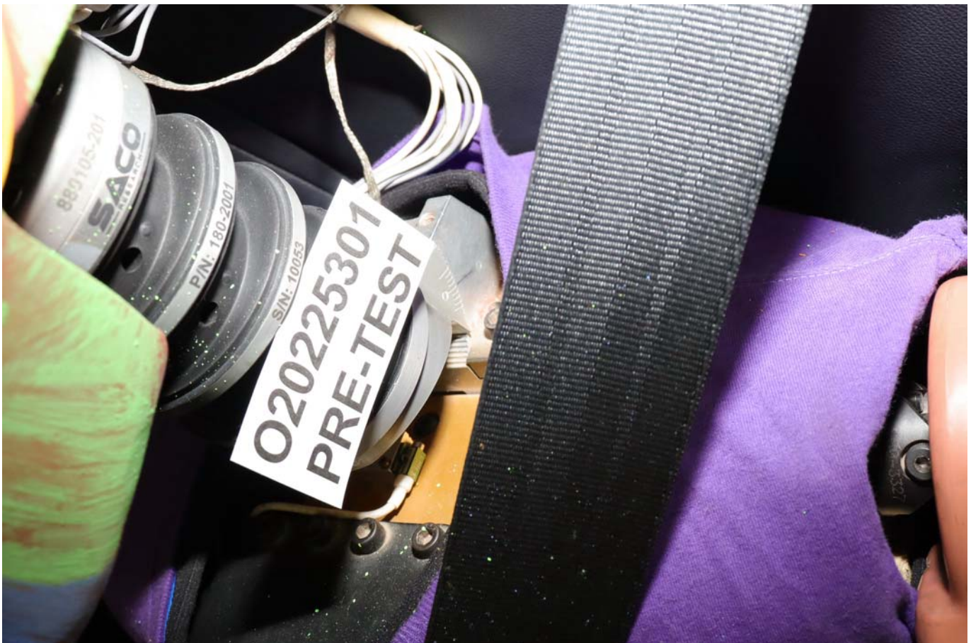
Photo No. 030 - Pre-Test Left Side View of Dummy Neck Showing Position of Adjustable Neck Bracket
