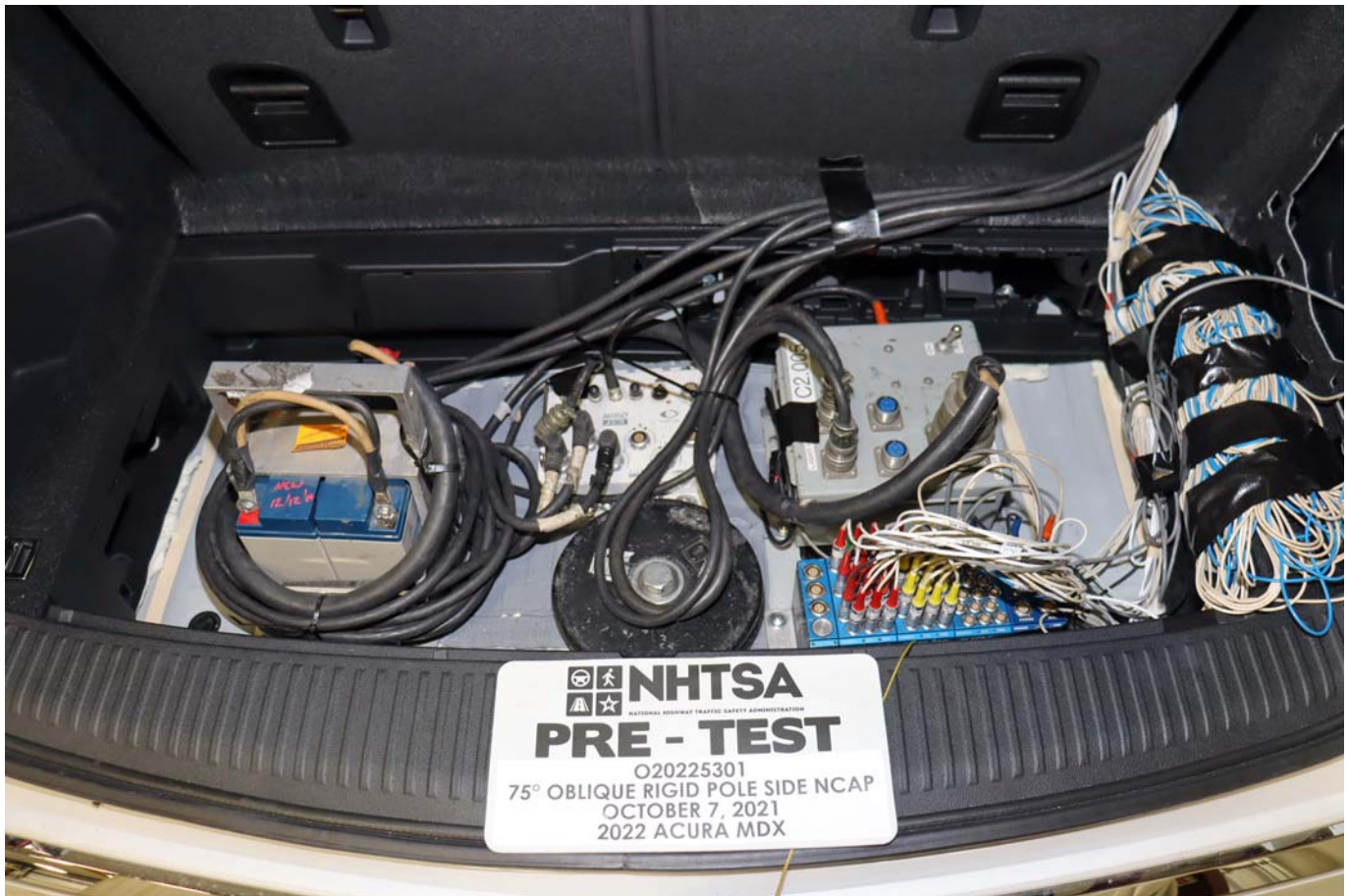
Photo No. 063 - Pre-Test Ballast View
