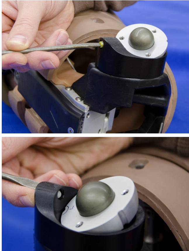
Figure 55. Back out spring-loaded set screw
