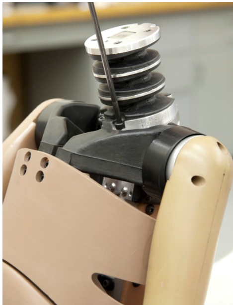
Figure 21. Remove screws from front base of neck using ball tip hex wrench
