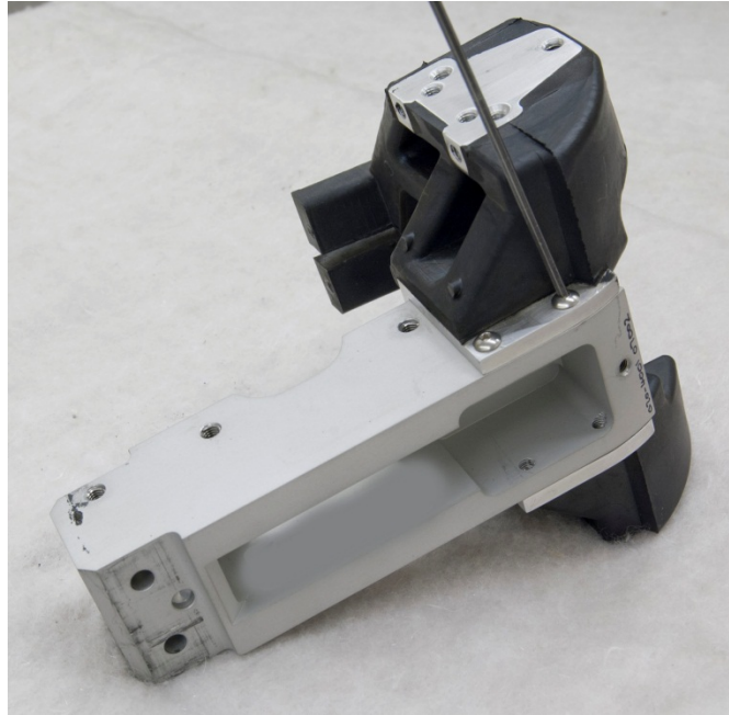
Figure 71. Remove screws on opposite side of accelerometer adaptor
