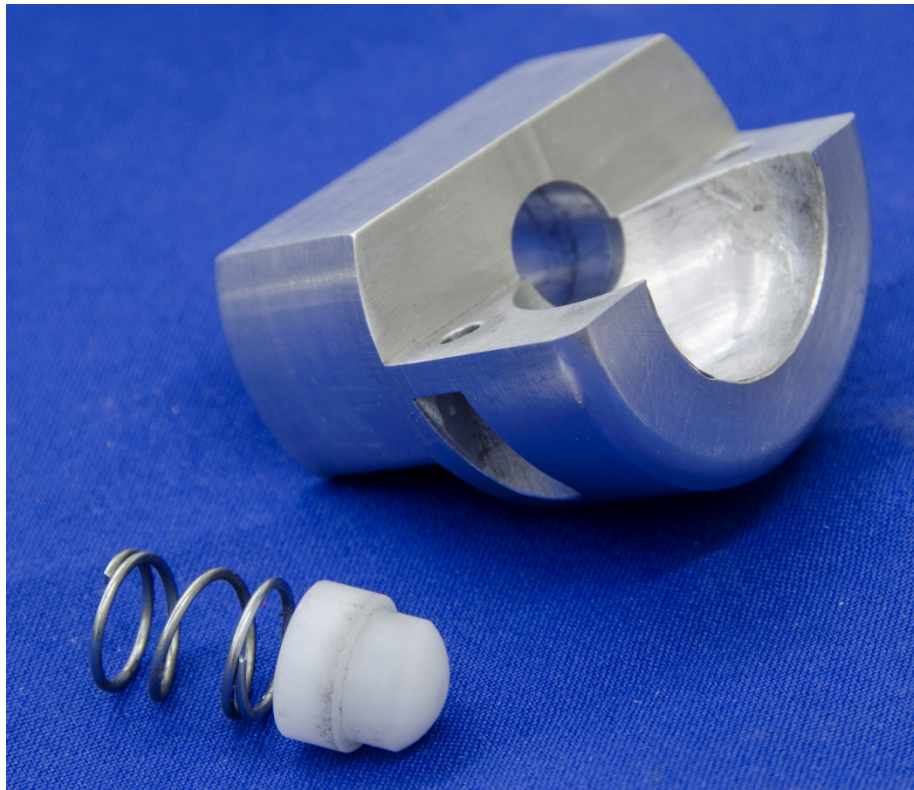
Figure 88. Spring and detent peg removed from hip joint assembly
