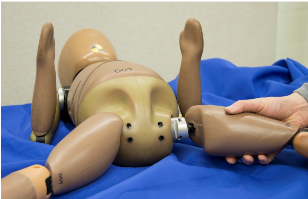
Figure 44. Separate leg from pelvis
