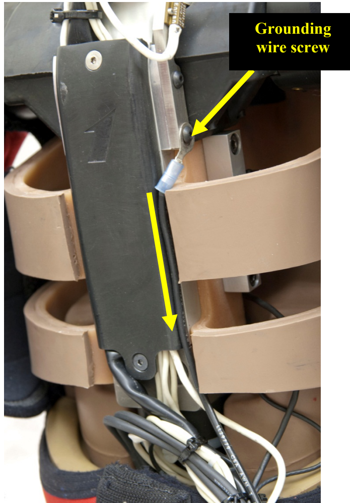
Figure 157. Installing grounding wire
