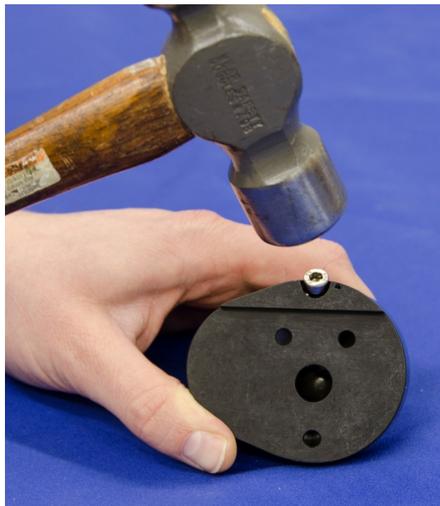
Figure 58. Using a hammer to remove shoulder ball
