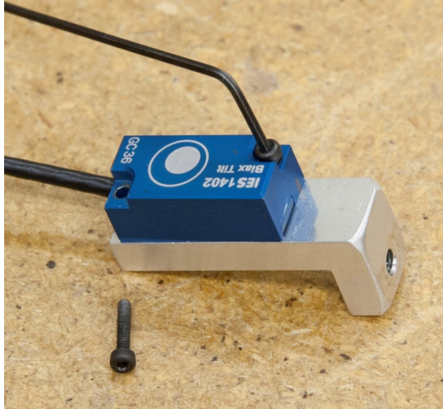
Figure 137. Install tilt sensor to bracket
