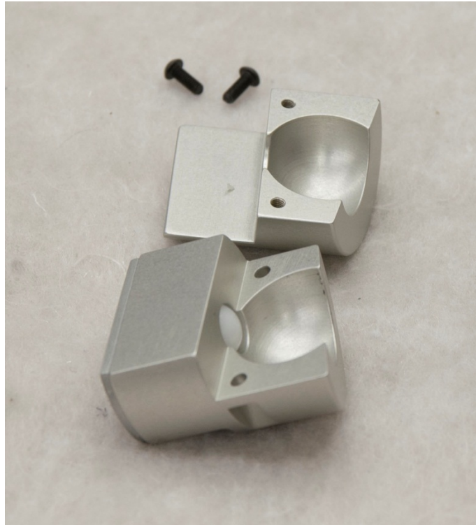
Figure 85. Hip joint after separating from leg
