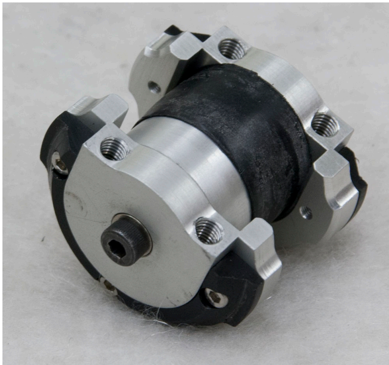
Figure 97. Pubic load cell assembly after removal from machined pelvis
