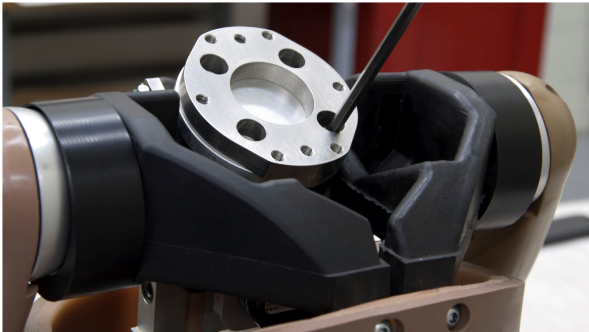
Figure 117. Install lower neck load cell to torso
