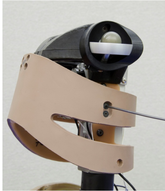
Figure 133. Secure IR-TRACC bracket to ribcage
