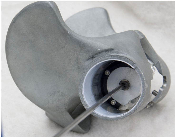
Figure 96. Remove pubic load cell assembly from machined pelvis
