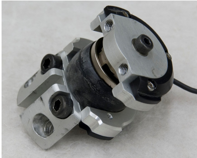
Figure 146. Install hip joint slide cover on struck side of pubic load cell assembly then compress pubic buffer
