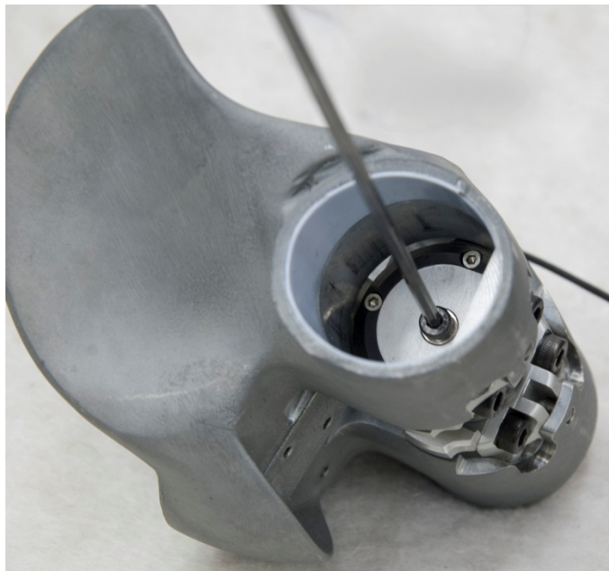
Figure 149. Remove SHCS to relive compression on pubic buffer
