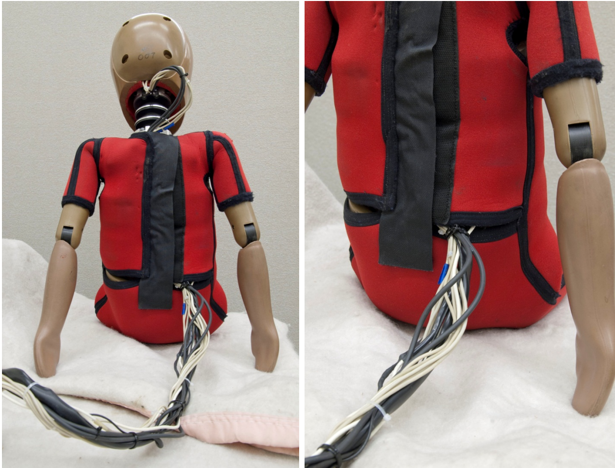
Figure 166. Wiring bundles after installation of suit
