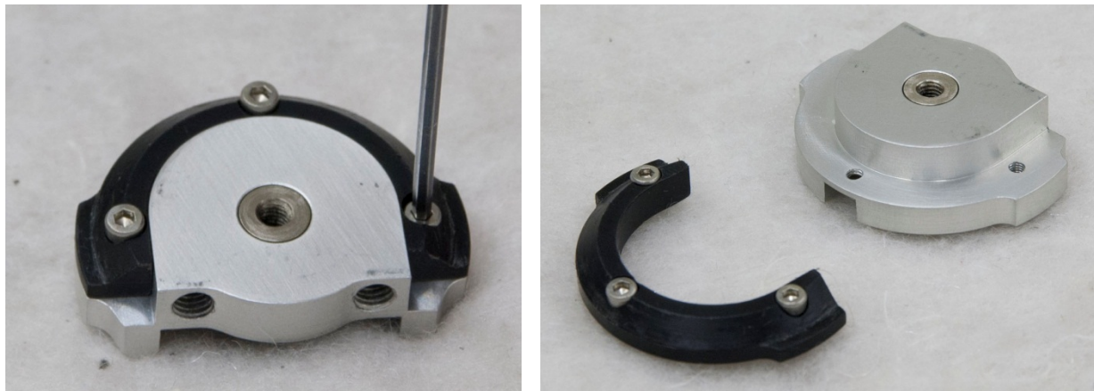
Figure 99. Remove hip joint slide spacer from hip joint slide assembly
