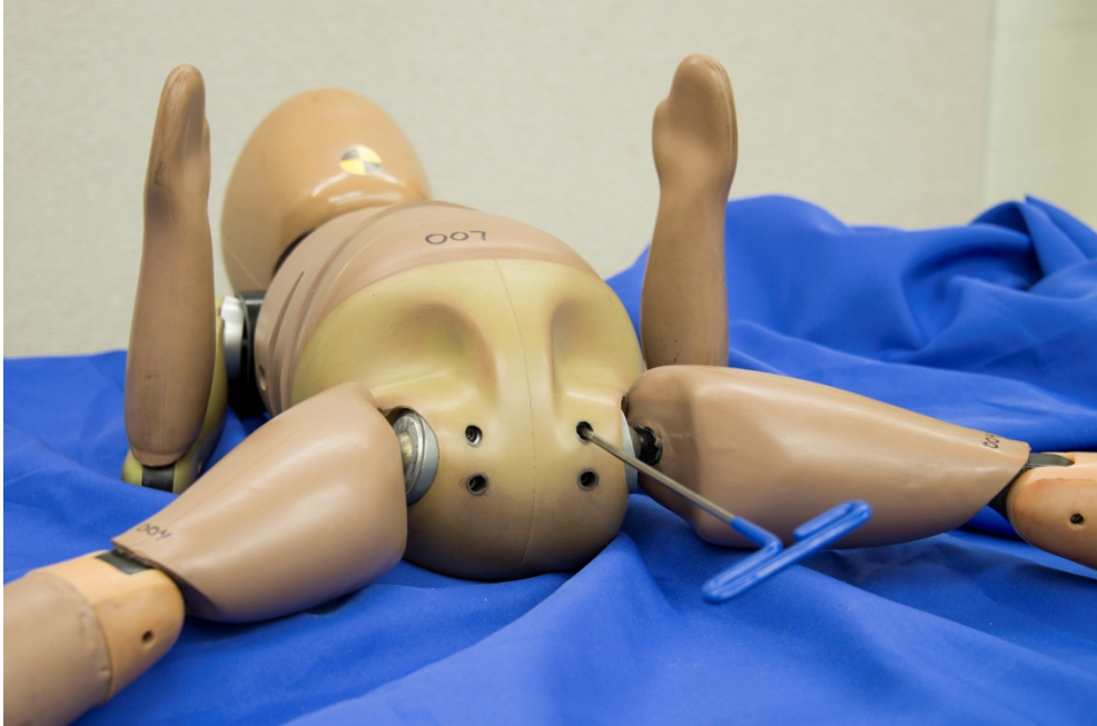
Figure 43. Remove SHCS from pelvis
