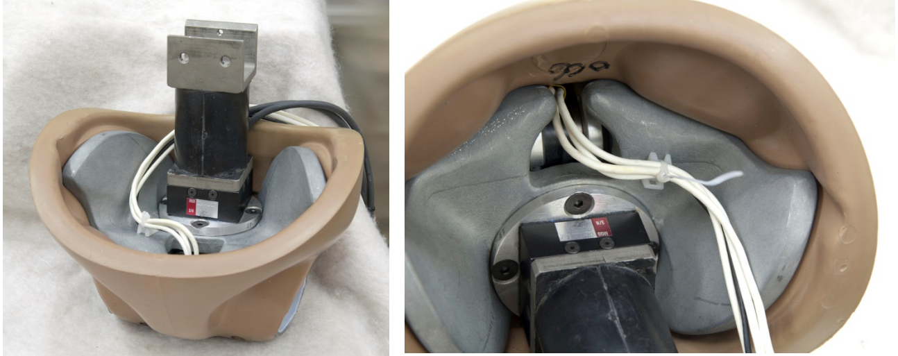
Figure 163. Pelvic wiring with pelvis skin installed
