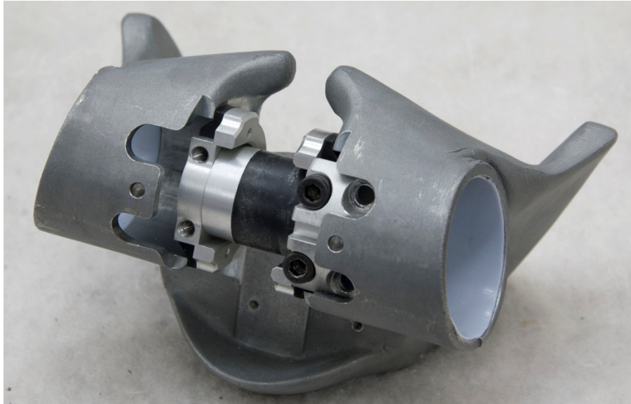
Figure 95. Remove hip joint cover on pubic load cell structural replacement side of machined pelvis
