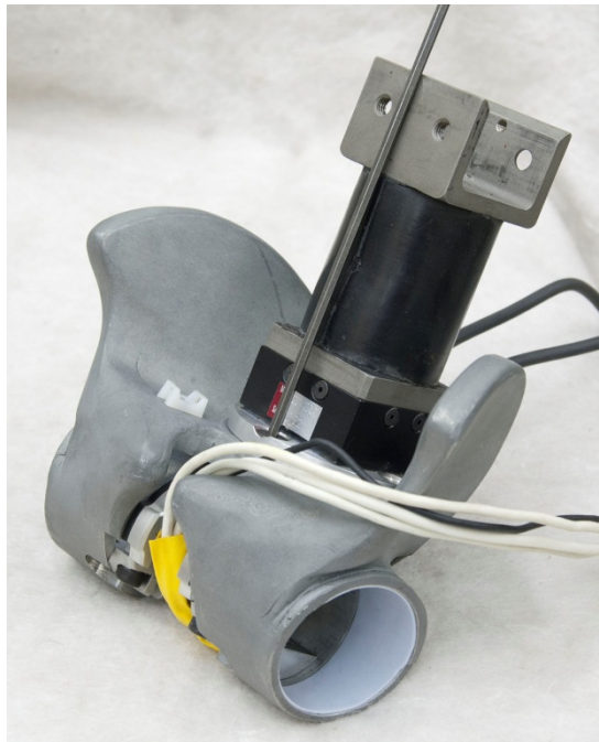
Figure 162. Wire route for pelvis accelerometers, pubic load cell, and lumbar load cell
