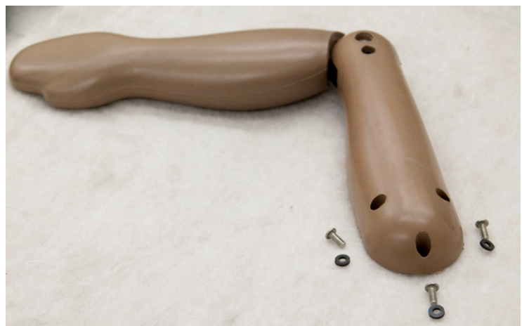
Figure 37. Arm removed from Q3s showing Viton® washers at shoulder
