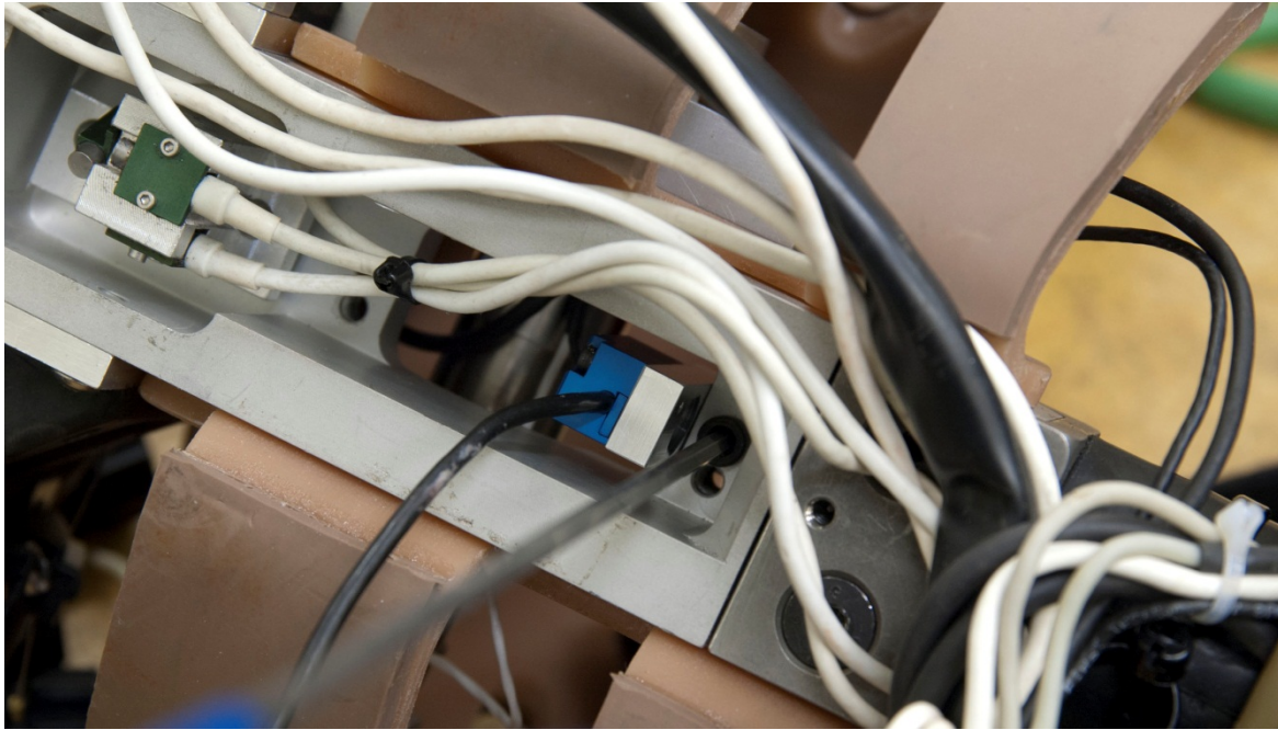
Figure 139. Install tilt sensor mount to thoracic spine
