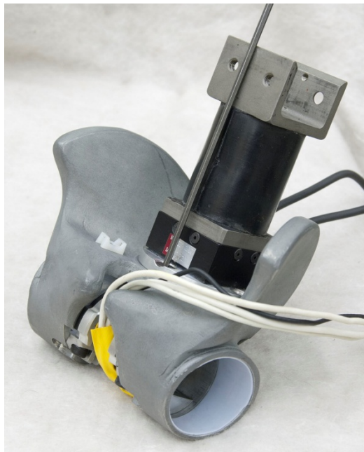
Figure 155. Install lumbar load cell to machined pelvis
