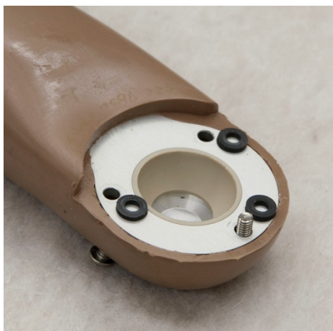
Figure 37. Arm removed from Q3s showing Viton® washers at shoulder
