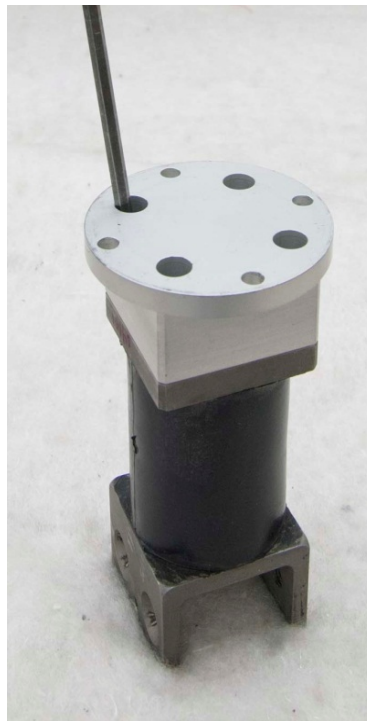
Figure 92. Remove lumbar load cell structural replacement
