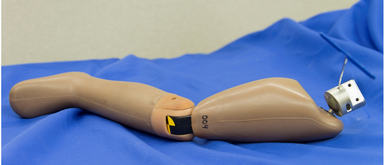
Figure 83. Remove hip joint assembly from leg
