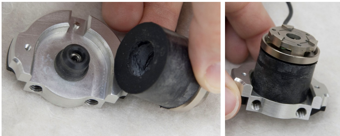
Figure 143. Install pubic buffer into hip joint slide assembly (spacer side)
