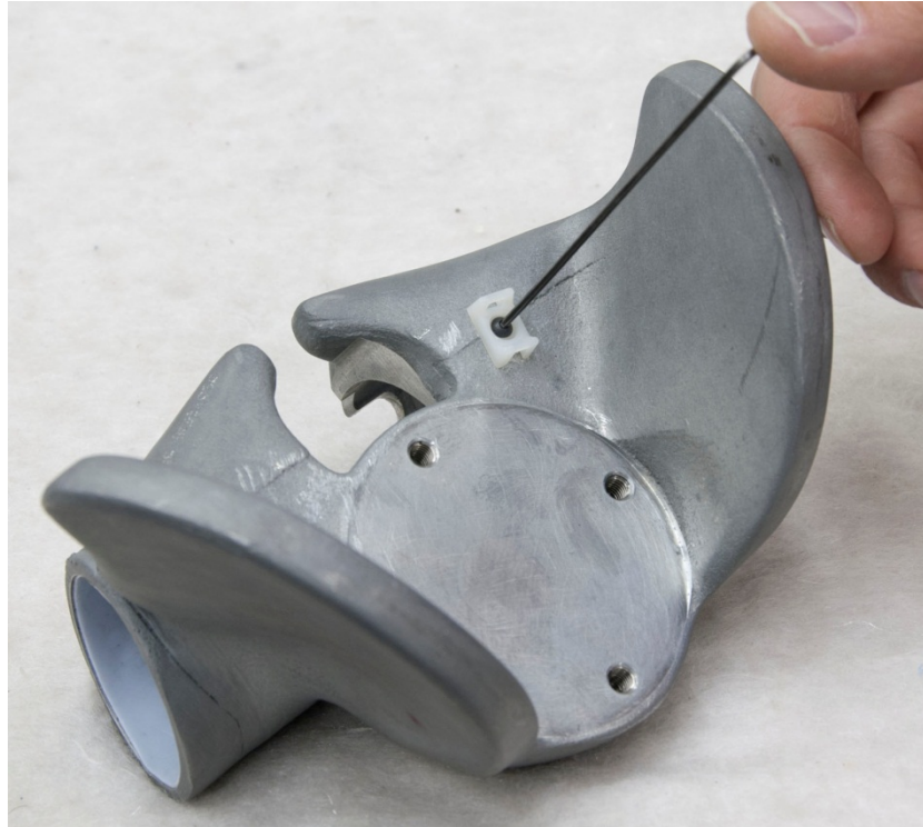
Figure 100. Remove #4 cable tie mount from machined pelvis
