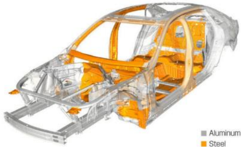
Illustration 1. Cadillac CT6 Multi-Material Body Structure 2
