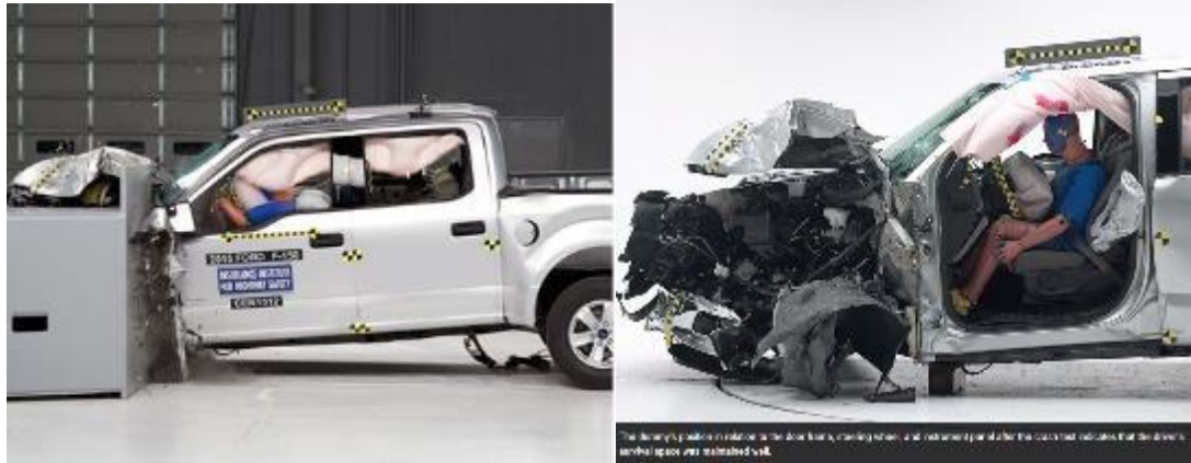
2015 Ford F-150 Front Fixed Barrier Crash Testing
