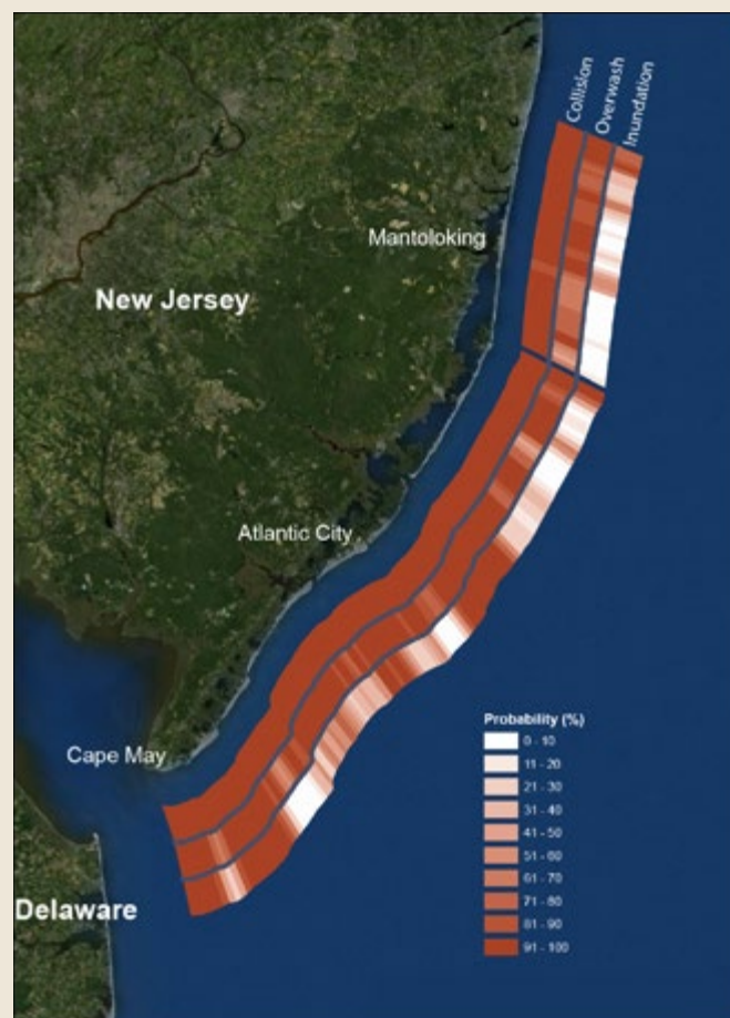
Figure 16.4. Predictions of coastal erosion prior to Sandy's arrival provided the region's residents and decision-makers with advance warning of potential vulnerability. The map shows three bands: collision of waves with beaches causing erosion on the front of the beach; overwash that occurs when water reaches over the highest point and erodes from the rear, which carries sand inland; and inundation, when the shore is severely eroded and new channels can form that lead to permanent flooding. The probabilities are based on the storm striking at high tide. For New Jersey, the model estimated that 21% of the shoreline had more than a 90% chance of experiencing inundation. These projections were realized, and made the New Jersey coastline even more vulnerable to the nor'easter that followed Hurricane Sandy by only 10 days. (Figure source: ESRI and USGS 2012 25 ).
