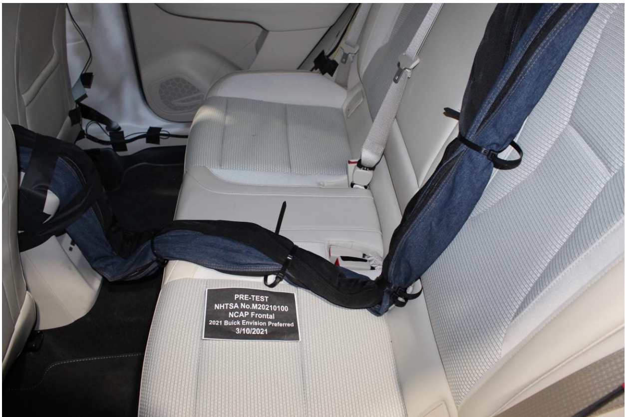
Figure A-28: Pre-Test Dummy Cable Routing
