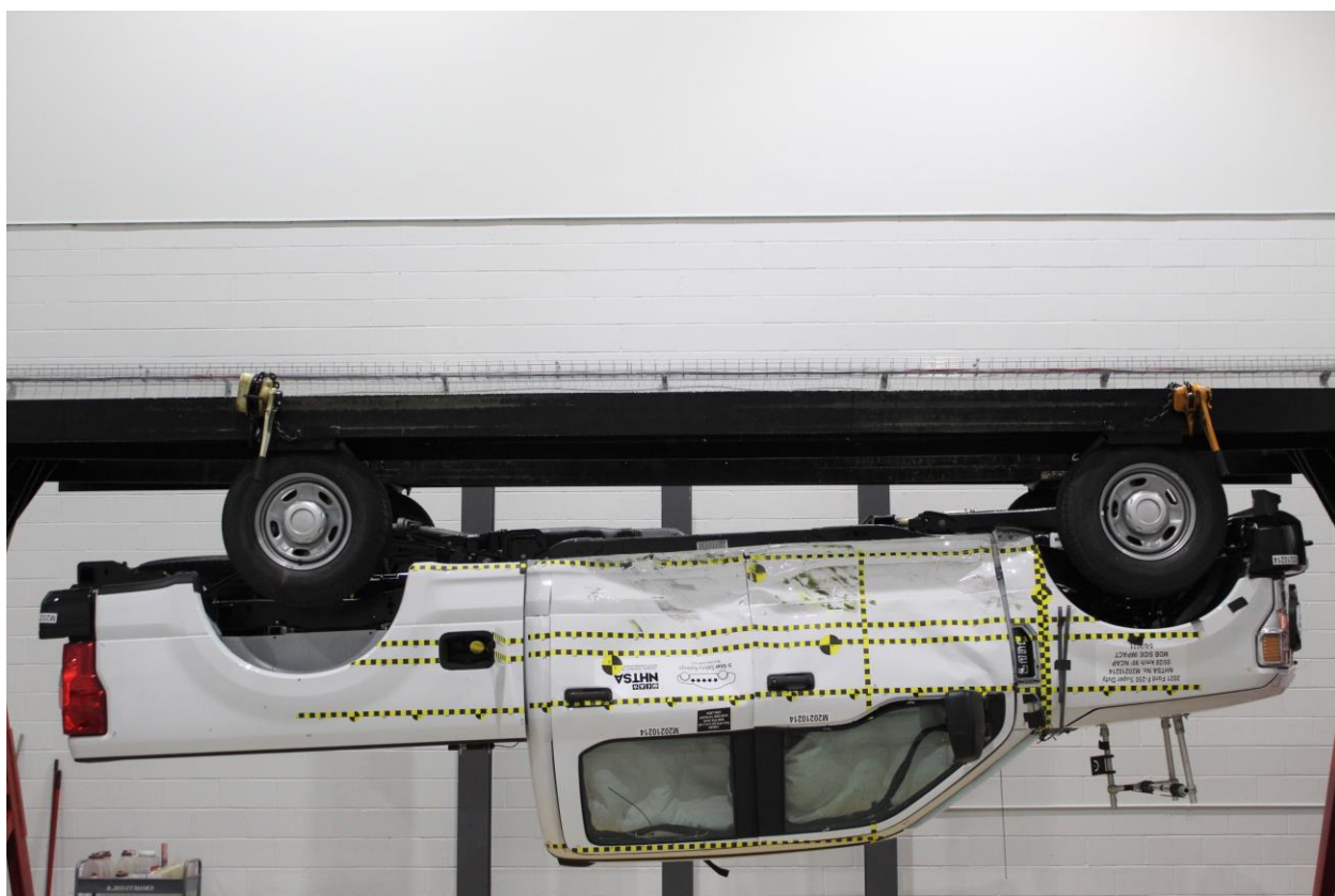
Figure A-98: FMVSS No. 301 Static Rollover 180 Degrees
