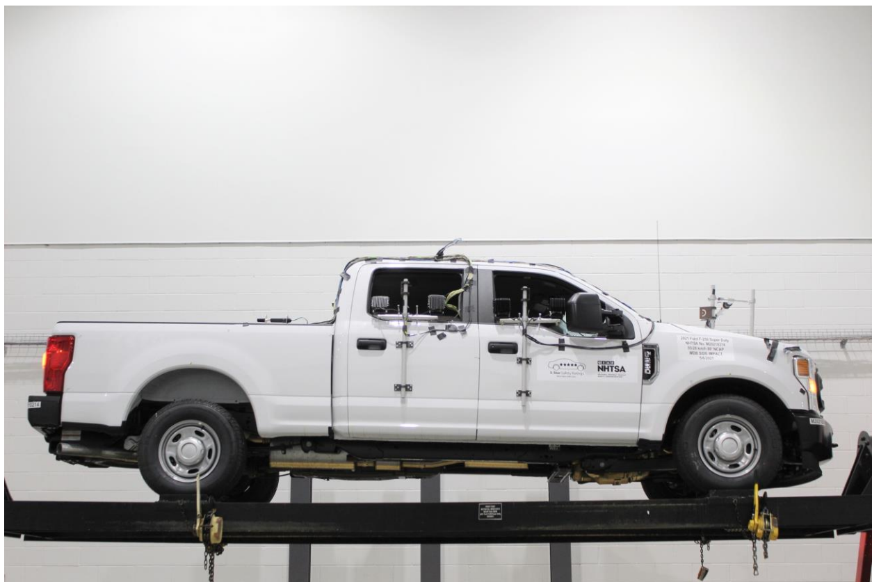
Figure A-100: FMVSS No. 301 Static Rollover 360 Degrees
