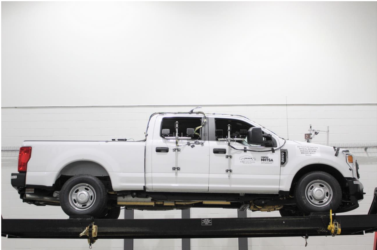
Figure A-96: FMVSS No. 301 Static Rollover 0 Degrees
