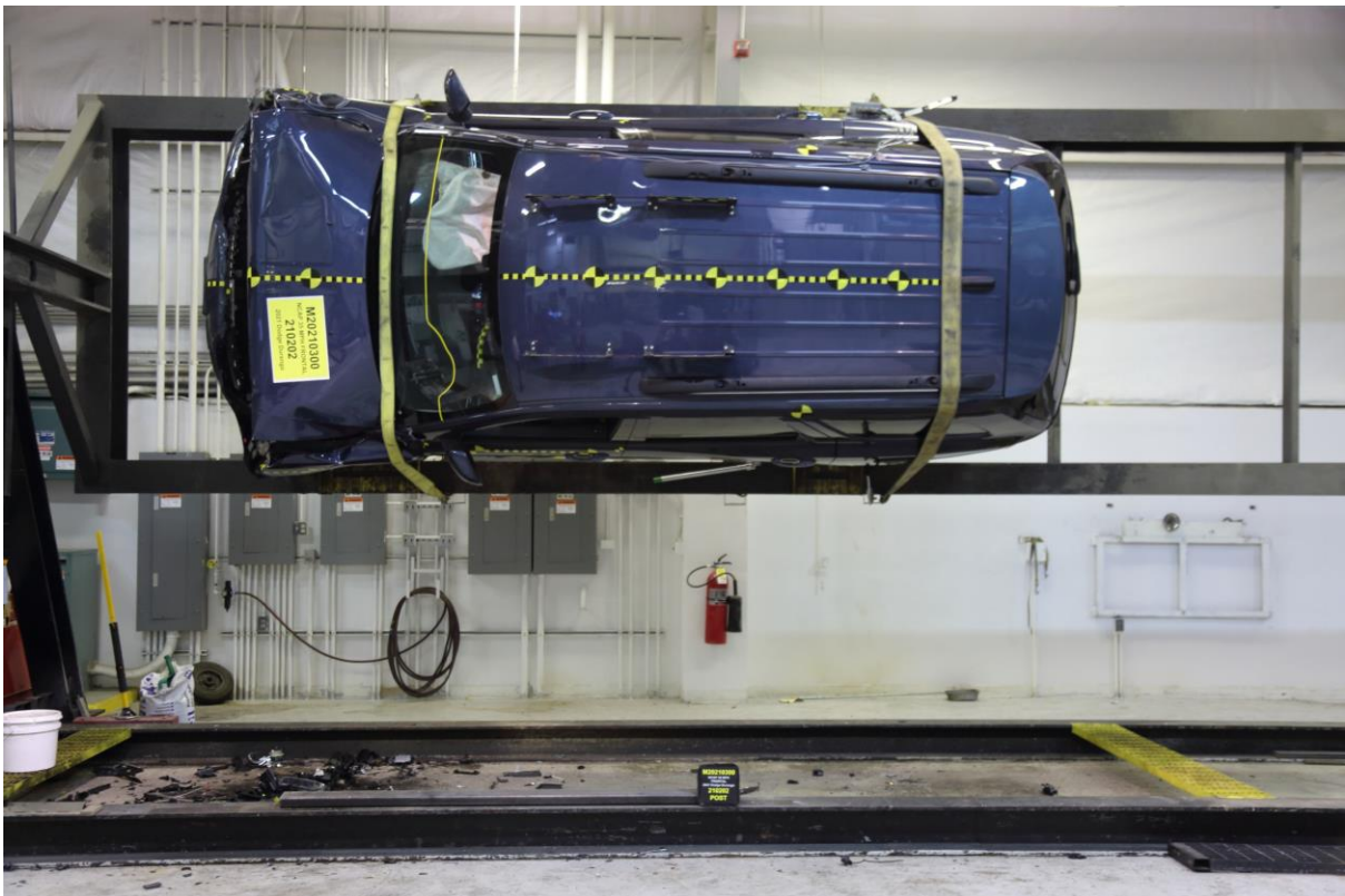
078 Vehicle at 90° on Static Rollover Device
