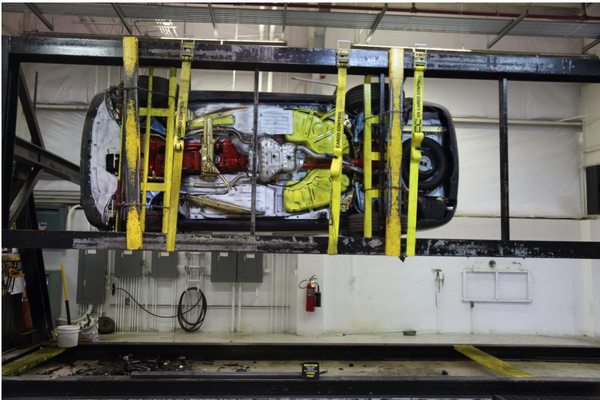
080 Vehicle at 270° on Static Rollover Device
