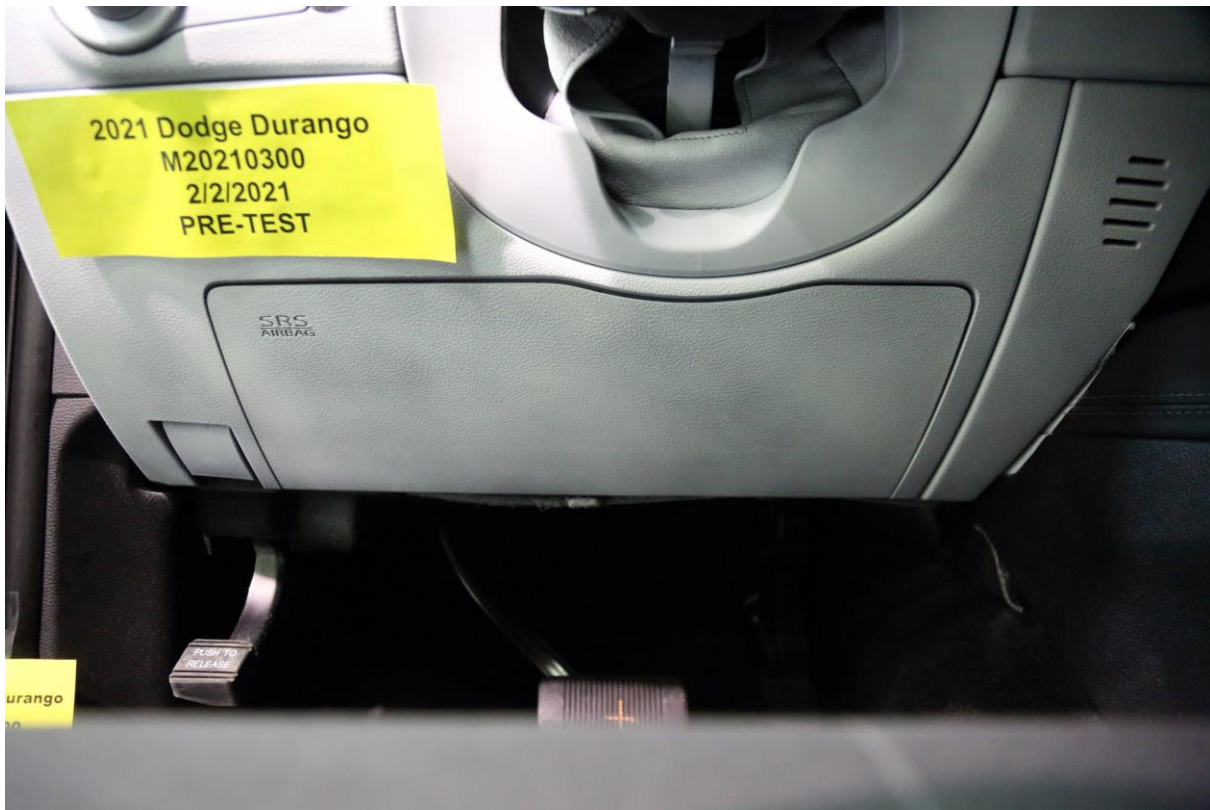
044 Pre-Test Driver's Side Knee Bolster
