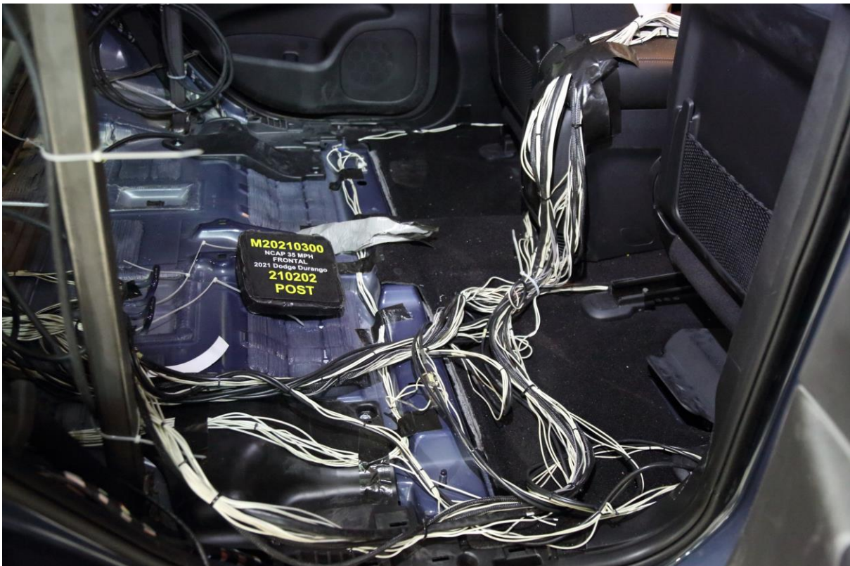
029 Post-Test Dummy Cable Routing
