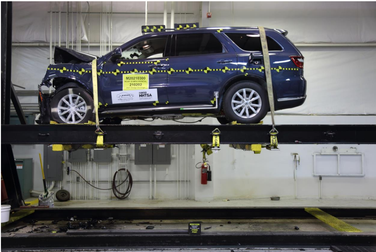
077 Vehicle at 0° on Static Rollover Device
