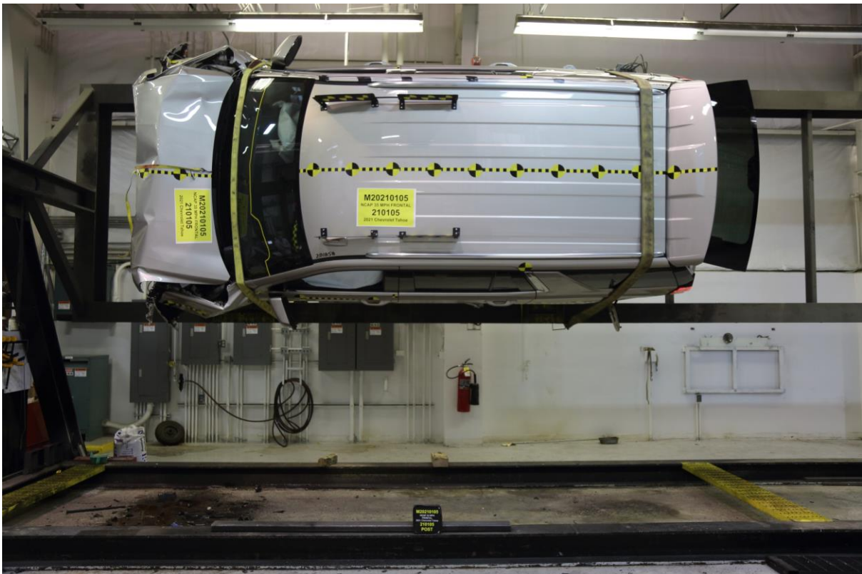
078 Vehicle at 90° on Static Rollover Device
