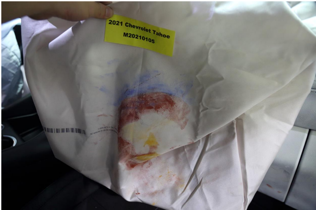
072 Post-Test Passenger Dummy Contact with Airbag
