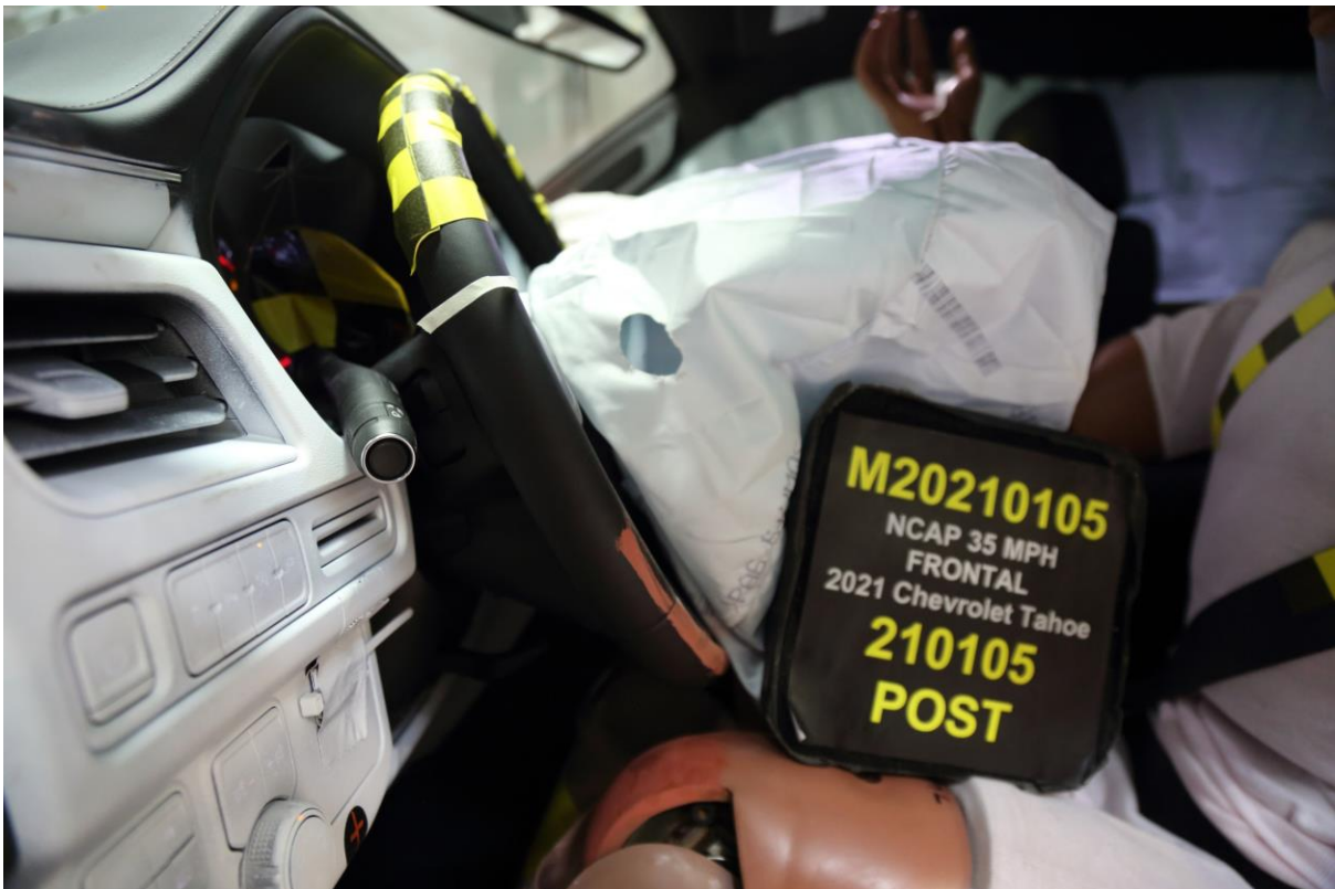
052 Post-Test View of the Steering Wheel
