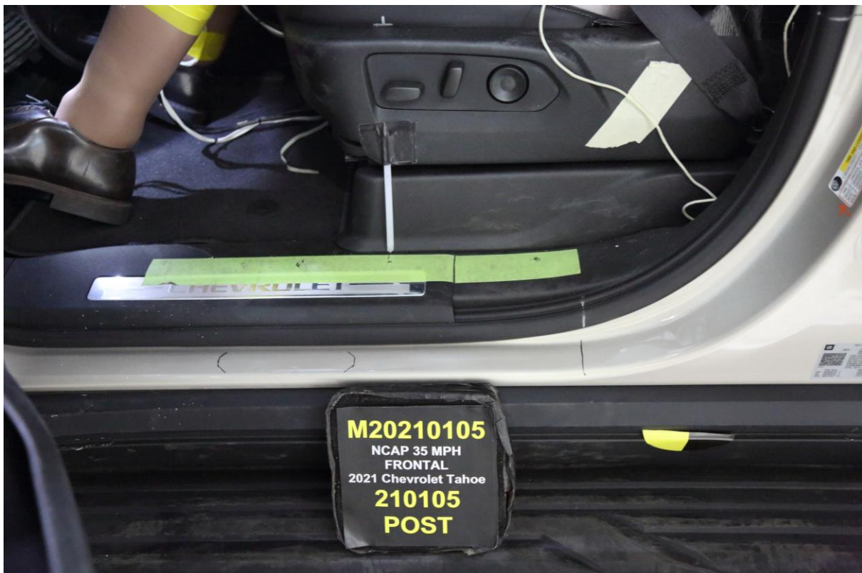
037 Post-Test Driver's Seat Fore-Aft Markings
