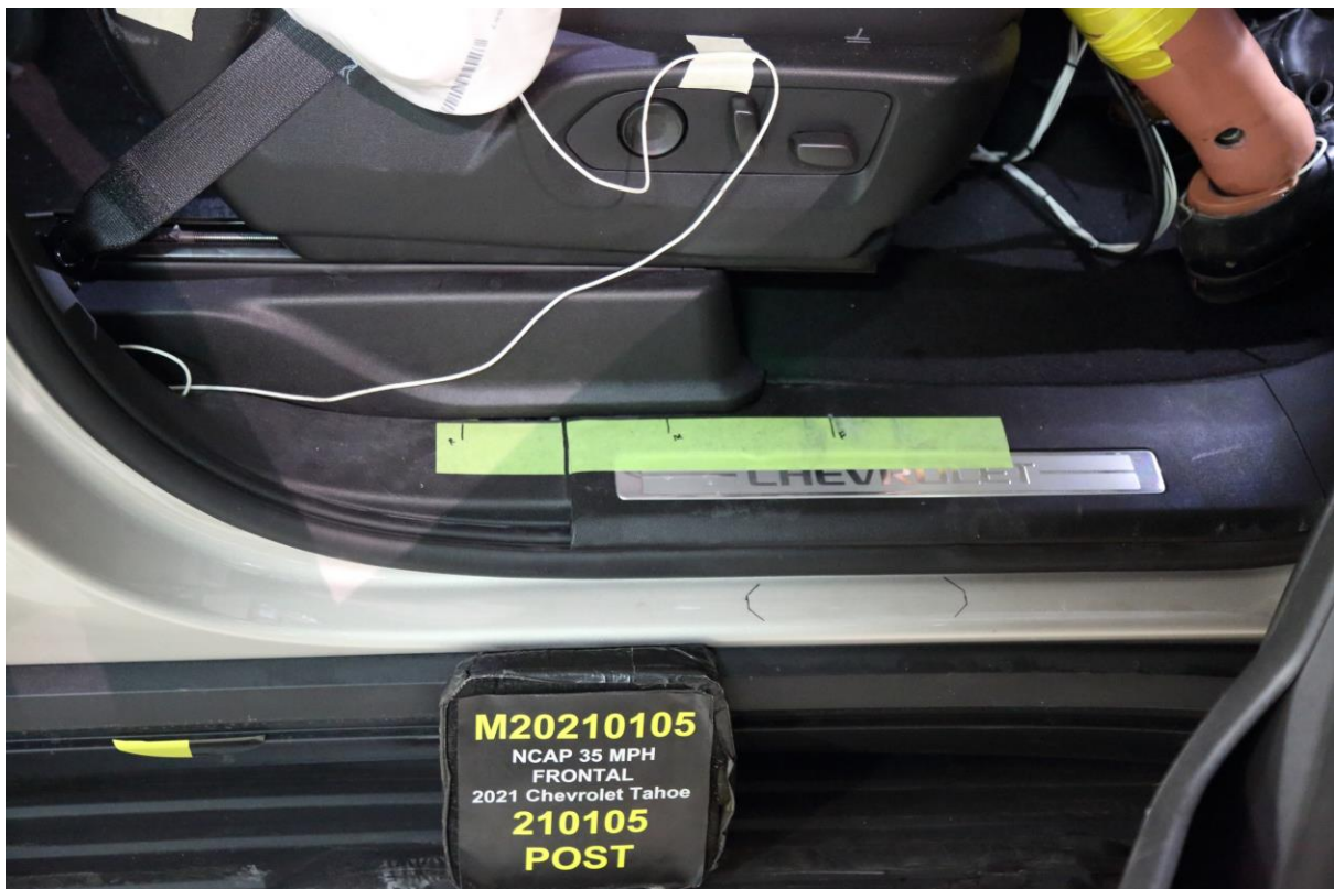
060 Post-Test Passenger's Seat Fore-Aft Markings
