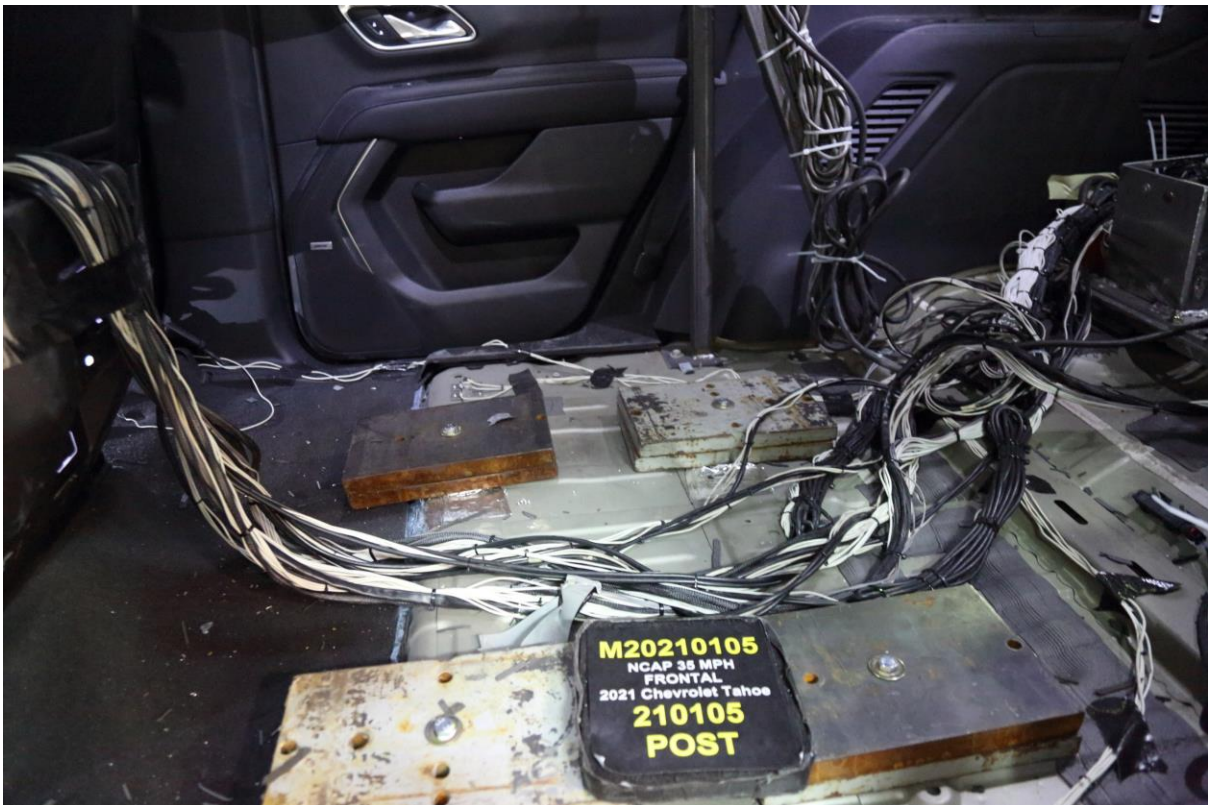
029 Post-Test Dummy Cable Routing
