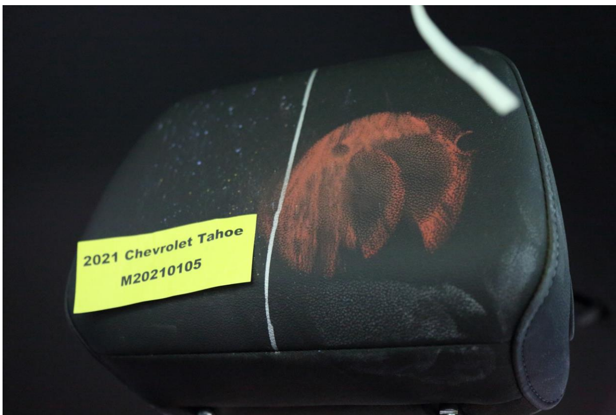
050 Post-Test Driver Dummy Contact with Headrest
