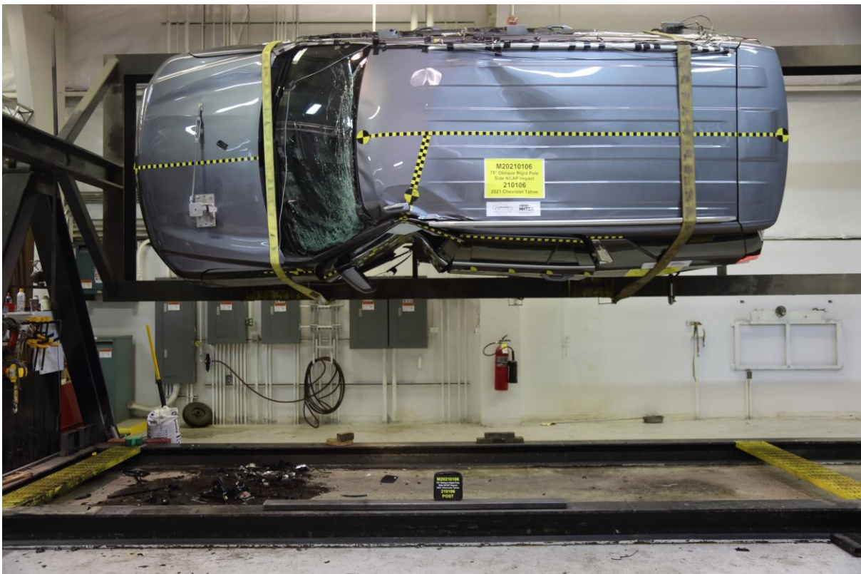
No. 066 FMVSS No. 301 Static Rollover 90 Degrees
