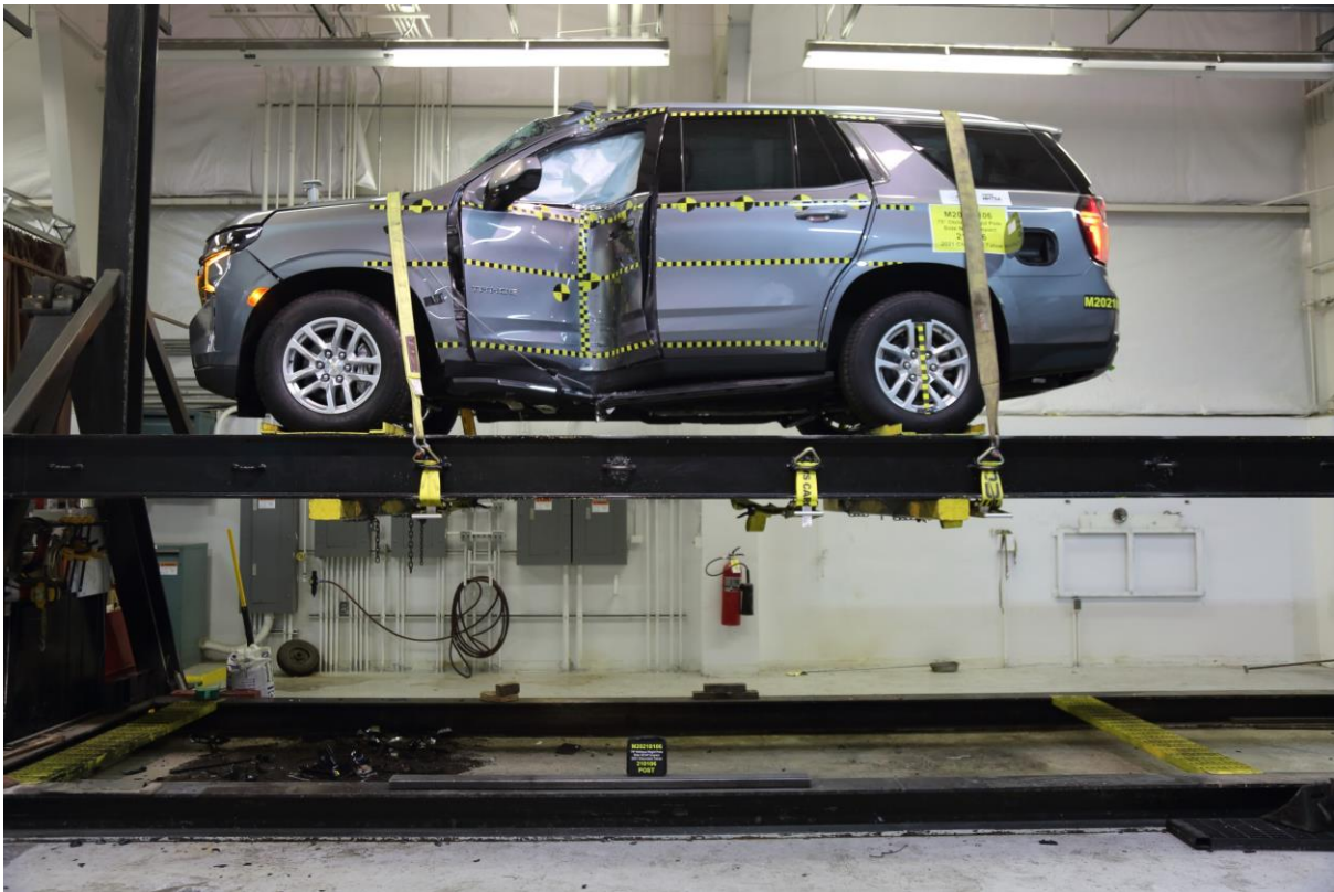
No. 065 FMVSS No. 301 Static Rollover 0 Degrees
