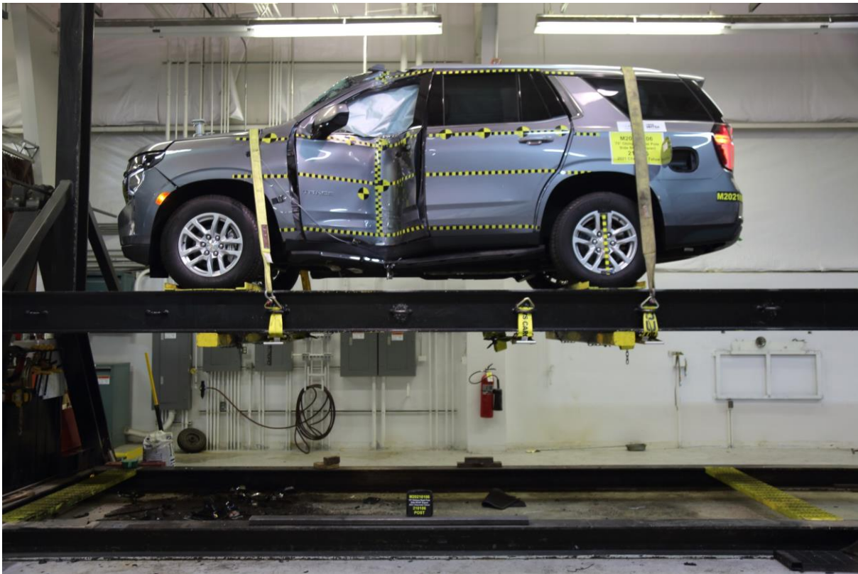
No. 069 FMVSS No. 301 Static Rollover 360 Degrees
