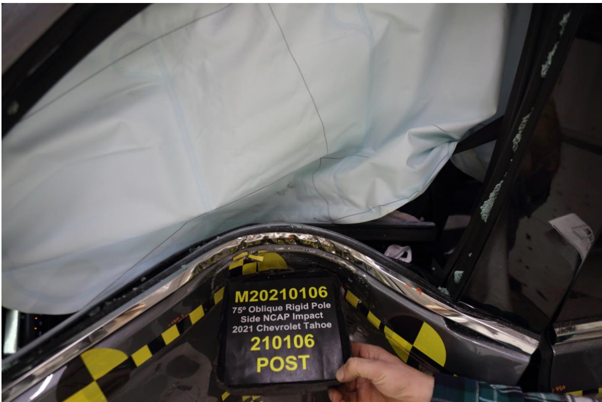
No. 041 Post-Test Dummy and Door Clearance View
