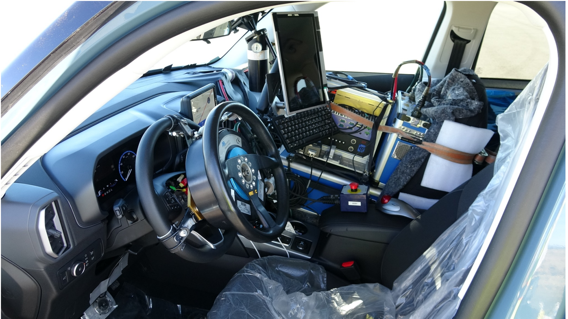
Figure A9. Steering Controller and Computer
