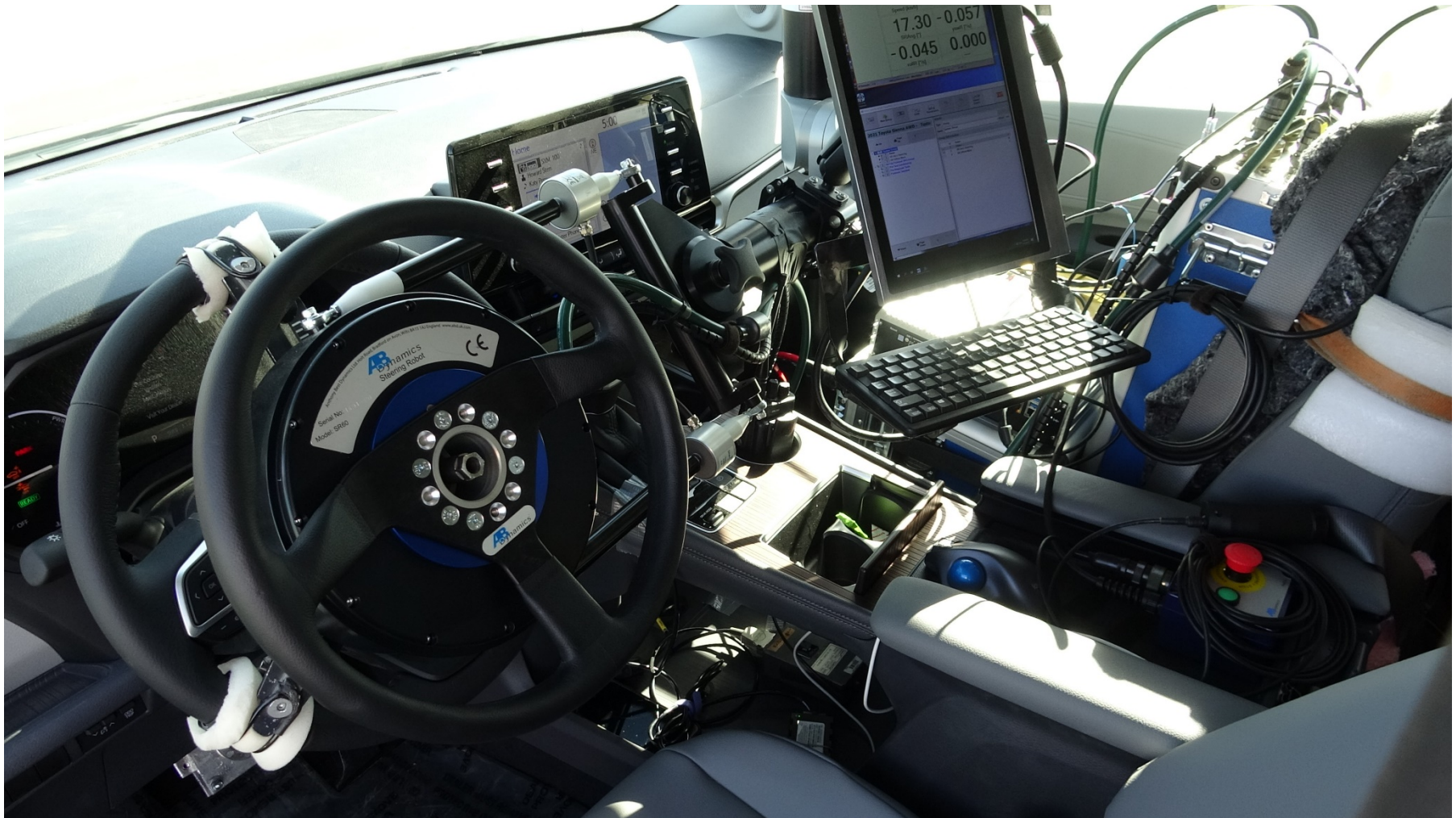
Figure A9. Steering Controller and Computer
