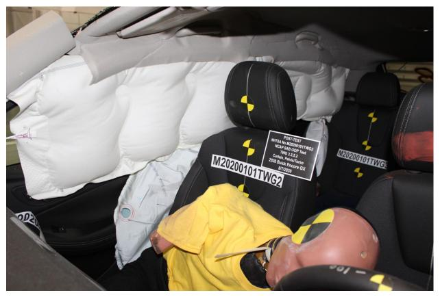
Figure A-14: Post-Test Dummy Left 3/4 Front View
