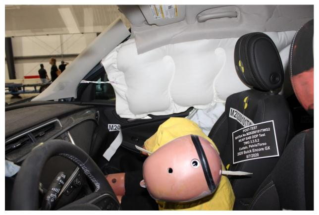
Figure A-10: Post-Test Dummy Left Side View
