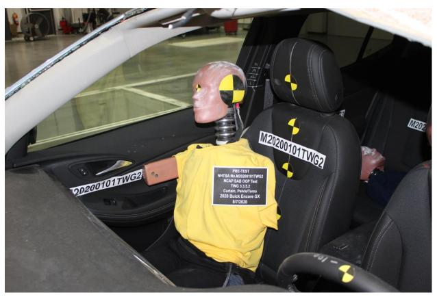
Figure A-13: Pre-Test Dummy Left 3/4 Front View
