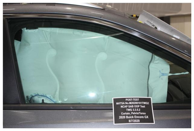
Figure A-24: Post-Test Dummy Right Side View
