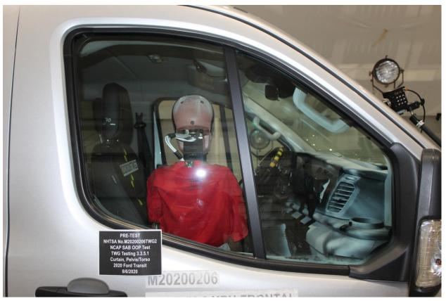
Figure A-23: Pre-Test Dummy Right Side View
