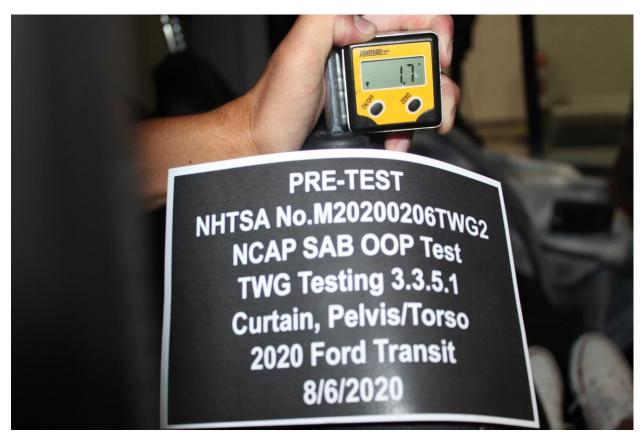
Figure A-8: Pre-Test Vehicle Seat Back Angle
