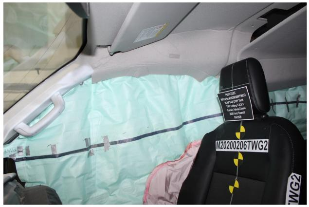
Figure A-27: Post-Test Curtain Air Bag Left <sup>3</sup>/<sub>4</sub> Front View
