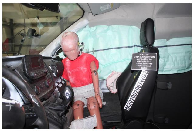
Figure A-10: Post-Test Dummy Left Side View
