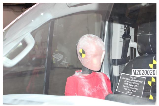
Figure A-15: Pre-Test Dummy Left <sup>3</sup>/<sub>4</sub> Close-up View
