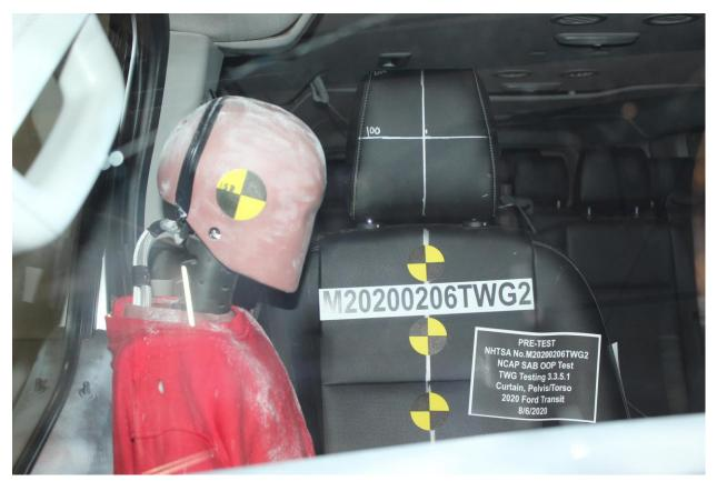
Figure A-19: Pre-Test Dummy Front Close-up View
