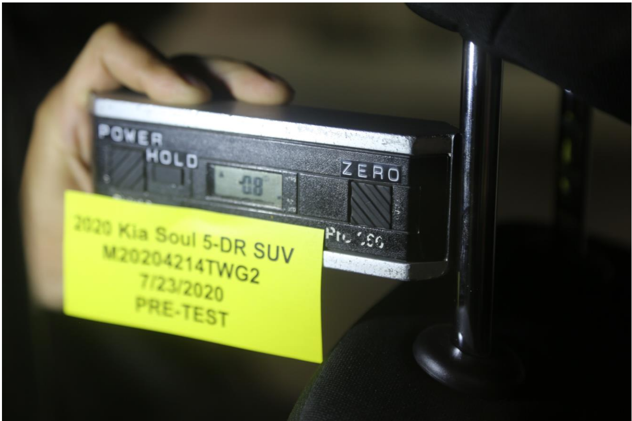
Figure A-8 Pre-Test Vehicle Seat Back Angle
