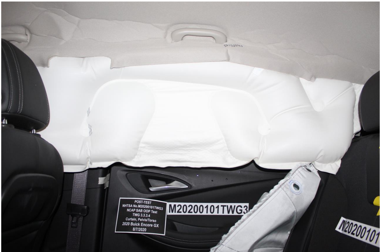
Figure A-26: Post-Test Curtain Air Bag Left Side View
