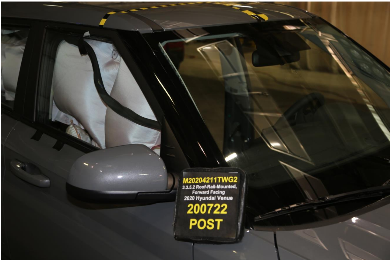
Figure A-22 Post-Test Dummy Right \frac{3}{4} Front View
