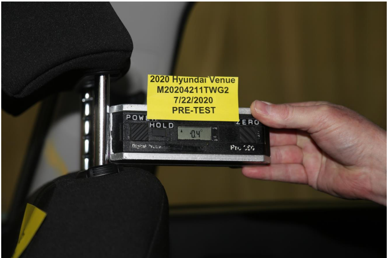
Figure A-8 Pre-Test Vehicle Seat Back Angle
