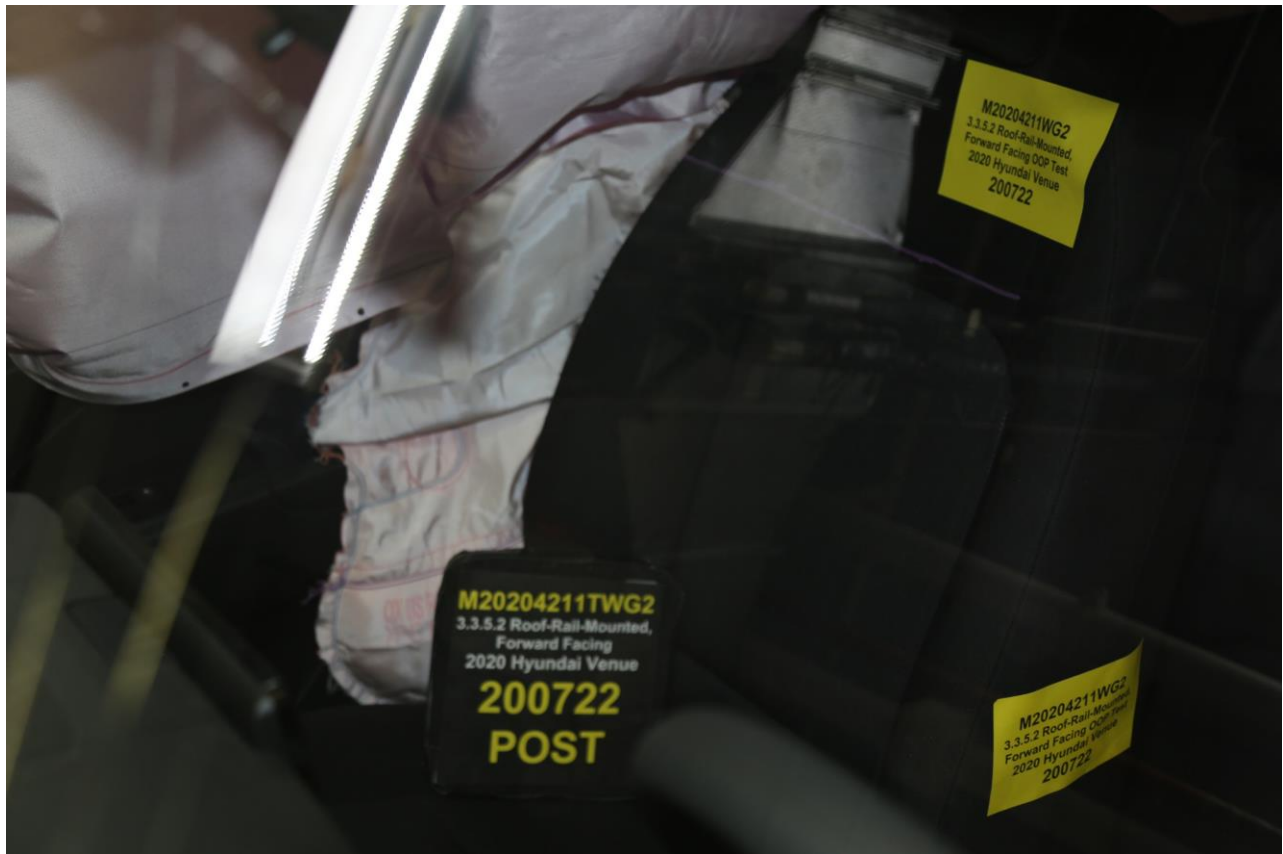
Figure A-27 Post-Test Curtain Air Bag Left ¾ Front View
