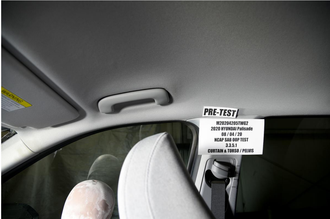
FIGURE 5. Pre-Test Vehicle Location of Air Bag 1 (vehicle headliner for curtain air bag)
