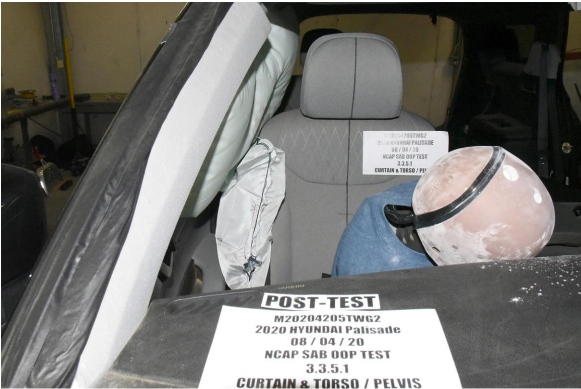
FIGURE 28. Post-Test Curtain Air Bag Front View
