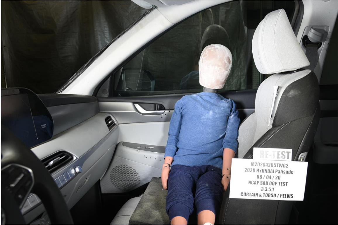
FIGURE 11. Pre-Test Dummy Left Side Close-up View
