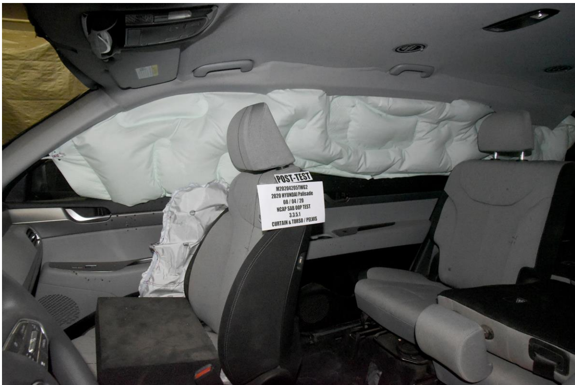
FIGURE 26. Post-Test Curtain Air Bag Left Side View
