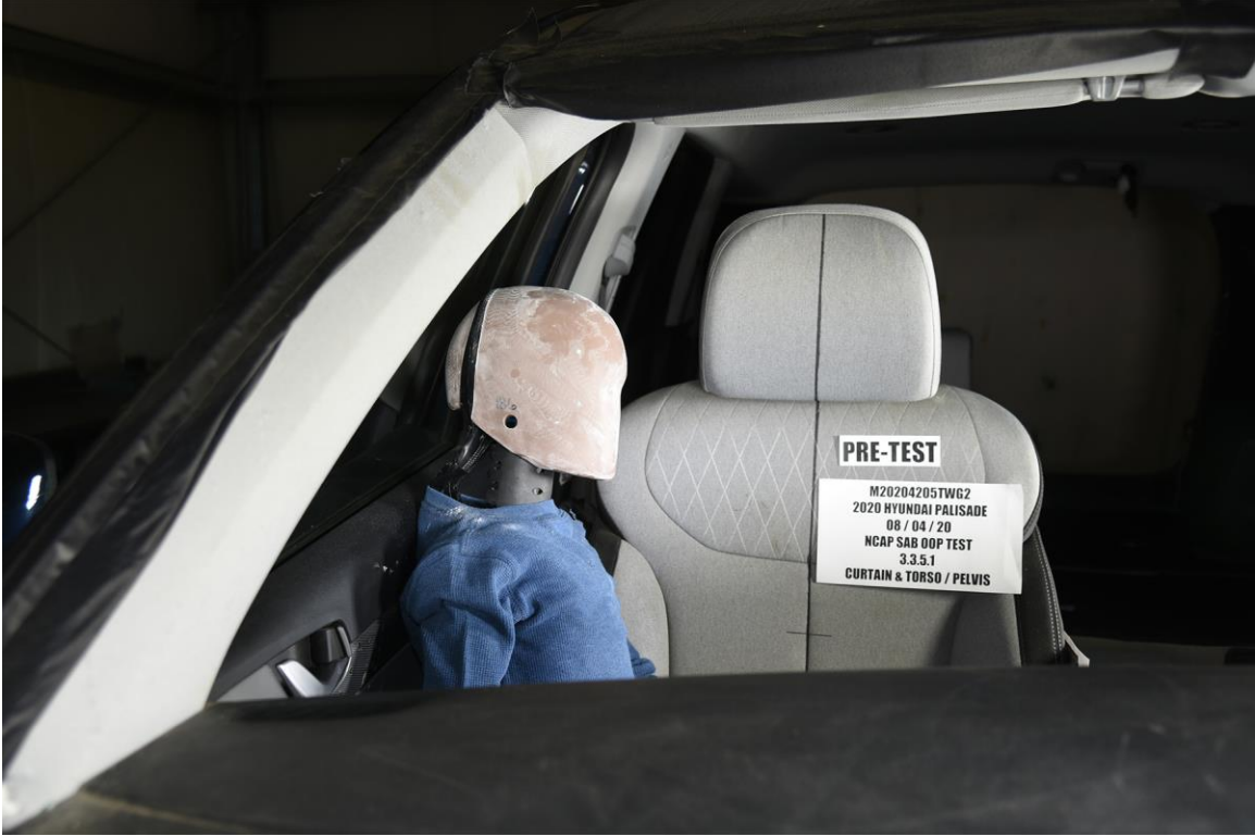
FIGURE 17. Pre-Test Dummy Front View
