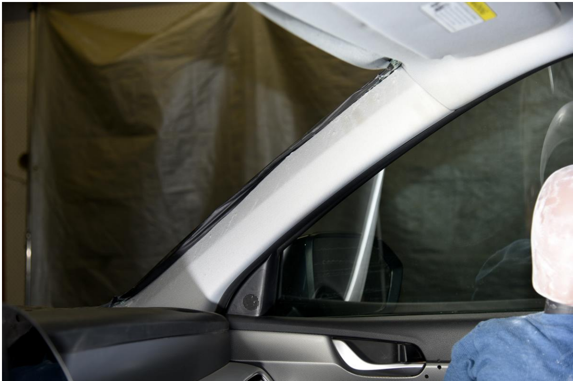
FIGURE 6. Pre-Test Vehicle Location of Air Bag 2 (vehicle a-pillar for curtain air bag)
