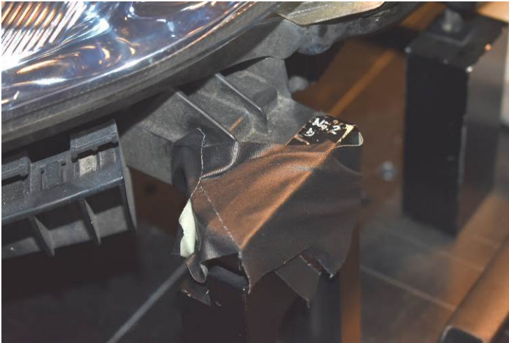
H-LH2 secured to fixture using gaffer tape.
