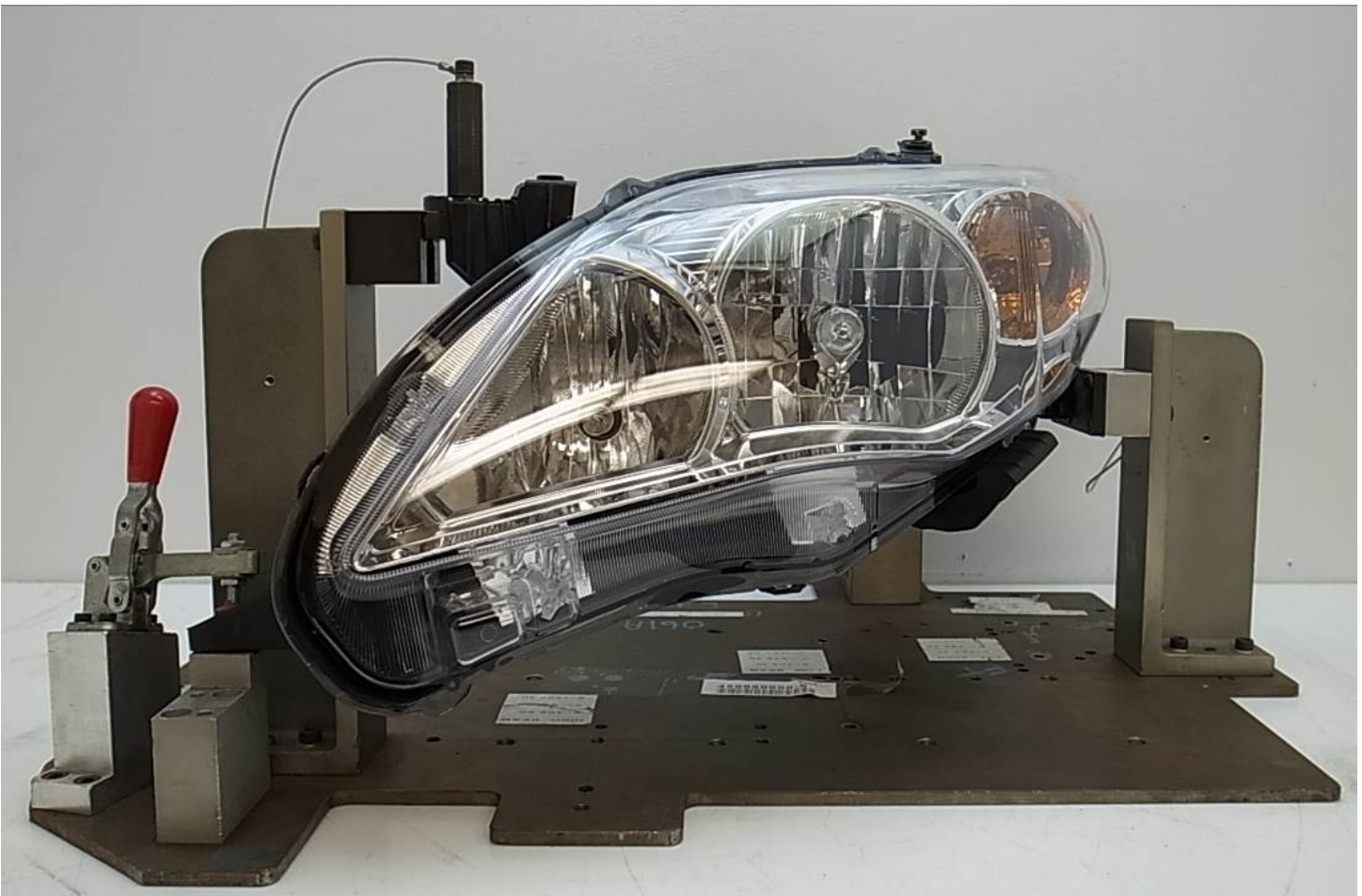
Lamp on Provided Fixture
