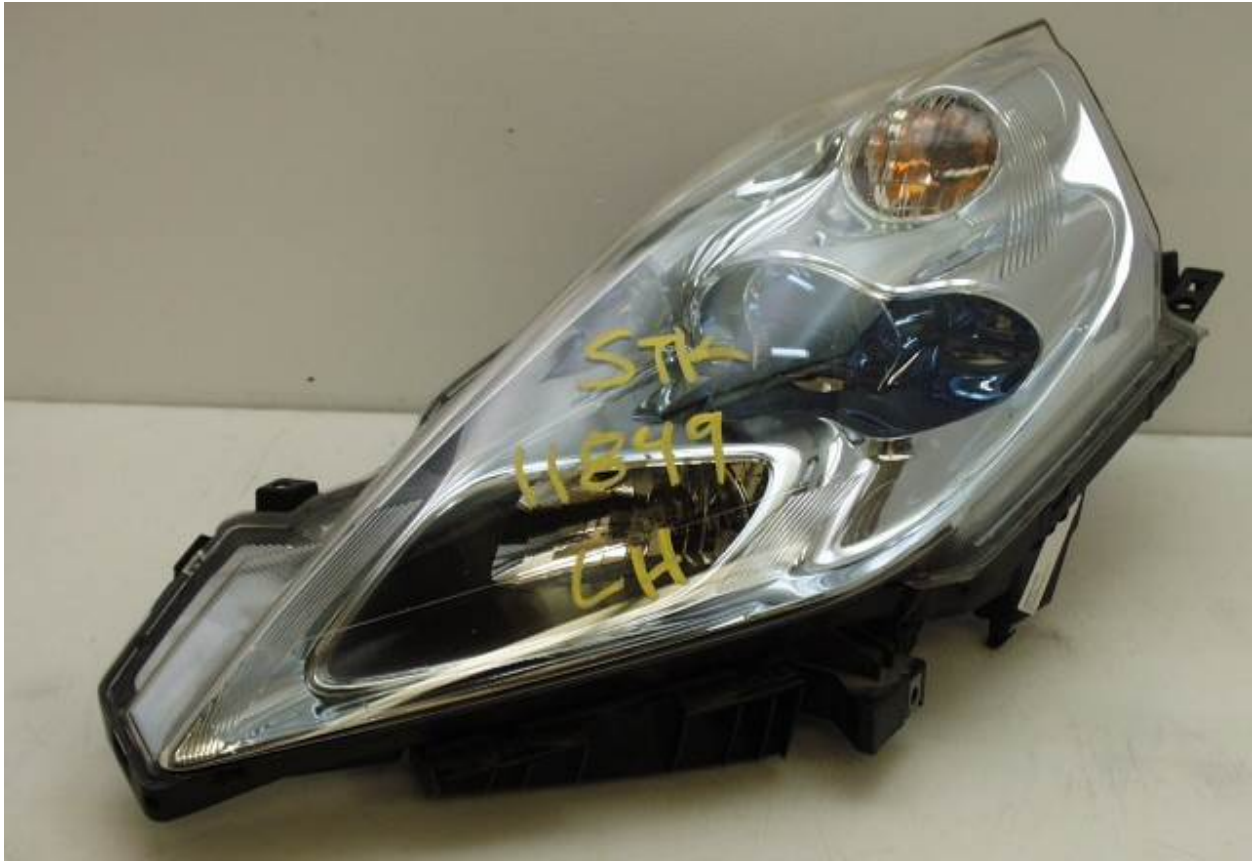
H-LH1 from 2012 Nissan Leaf (Markings removed from lens with alcohol prior to testing)
